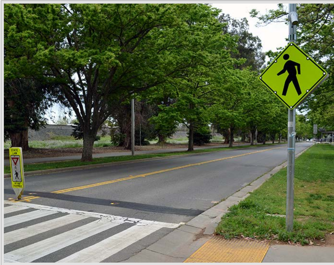
In the picture above, notice the lights within the crosswalk sign, and the lights on the street as well. The LEDs installed illuminate when pedestrians or cyclists approach the crosswalk.
