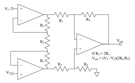
2. Build an instrumentation amplifier using the AD524 or the INA101. These chips have the desired high input impedance and the AD524 has several built in gain settings (it doesn't come cheap). Hook up your chip according to the data sheet instructions for a gain of 10. Verify the gain with known input voltages.
