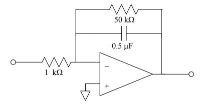
Measure the gain as a function of frequency. What is the approximate cutoff frequency? How does it compare to the theoretical value?
