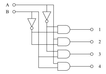
Wire the inputs to the logic switches to the +5 and GND lines on the ELVIS to select the states of A and B. Wire outputs 1-4 to LEDs (with resistors) as logic indicators.
