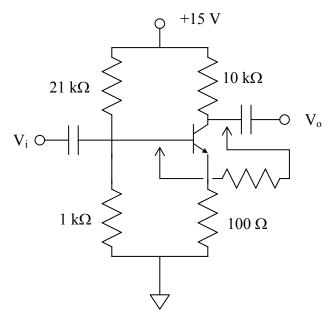
Add the feedback network (a 20 k $\Omega$  resistor). Measure the gain as a function of frequency. Again observe the output when driven by a triangle-wave. At what frequency is the triangle wave distorted?
