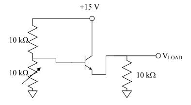
Measure the voltage across the load as you adjust the decade box from 1 k $\Omega$  to 10 k $\Omega$ . Now remove the amplifier and measure the voltage across the
