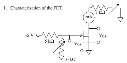
Build the above circuit, use the datasheet for the appropriate JFET to identify the terminals. For a fixed  $V_{GS}$ , record  $V_{DS}$  and  $I_D$  as you vary the voltage on the drain. Do not exceed the transistor ratings (see datasheet). Try to do this for  $V_{GS} \approx 0$ , -0.3, -0.6, -1, and -2 V. Pay special attention in the region where  $V_{DS}$  is between 0 and 1 V.
