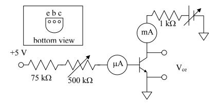
Build the above circuit. For a fixed  $I_b$ , record  $V_{ce}$  and  $I_c$  as you vary the voltage on the collector. Use the positive variable supply for the variable voltage on the collector side. Do not exceed the transistor ratings (see data sheet). Try to do this for  $I_b\approx 10,\,20,\,30,\,40,\,50~\mu A$ . Observe how the value of  $\beta$  varies depending on the value of  $I_b$  and  $V_{ce}$ .
