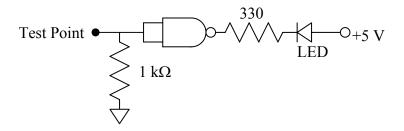
What is the purpose of the 1 k $\Omega$  resistor connected to the test point? What would happen if it were removed? In your write-up describe to me why this circuit works.
