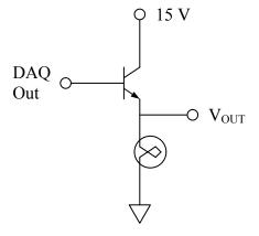
Because of the voltage drop across the BJT, also record the voltage across the lamp with your VI so that an accurate intensity versus voltage curve can be obtained. Plot the intensity as a function of the voltage in an x-y graph (use the XY Graph Express VI) in your VI. Write the XY Data file out to a file. Save this project as DAQ7 *name*.vi.
