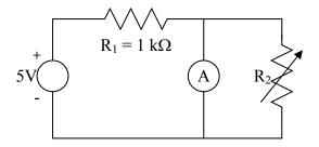
Initially, the resistance of  $R_2$  (a decade resistance box with a resolution of 0.1  $\Omega$  or less) should be "near infinite" resistance.
