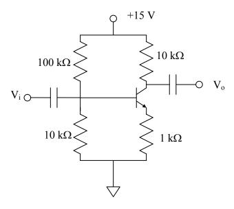
Use the largest capacitors you can find for the input and output. Measure the gain of the amplifier up to about 2 MHz. Does this amplifier behave as you would expect?
