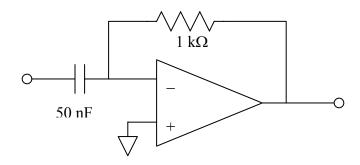
Observe the input and output with 1 kHz sine, triangle, and square-waves. Do your measured values make sense given what you know about the differentiator circuit?
