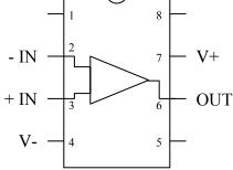
keep in mind that in circuit diagrams, the connections for  $V\pm$  are rarely shown.
