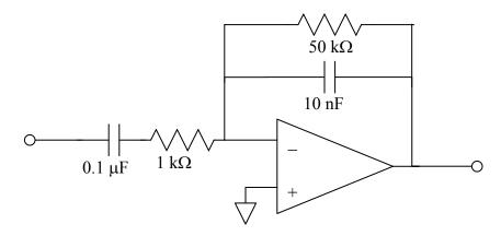
Measure the gain as a function of frequency. In your write-up, calculate the theoretical transfer function and compare it to what you observed.
