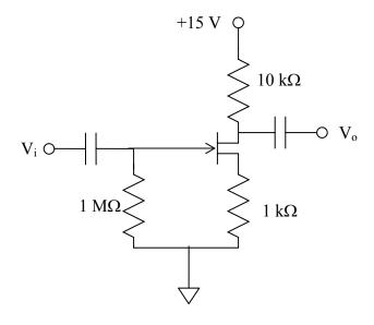
Use the largest capacitors you can find for the input and output. Measure the gain of the amplifier up to about 2 MHz. Does this amplifier behave as you would expect?
