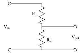
Select  $R_1$  and  $R_2$  so that they add to  $\sim 5~k\Omega$  (within 10%) and the gain of the circuit is 0.33 (within 2%). You may have to combine resistors to get a system that meets these requirements.
