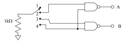
Use a wire as the four-way switch. You can use LEDs with 500  $\Omega$  resistors as simple logic probes. Does this circuit behave as you expect? Do not disassemble your circuit; you will use it in part 3.
