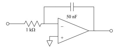
Observe the input and output with 1 kHz sine, triangle, and square-waves. Do your measured values make sense given what you know about the integrator circuit?
