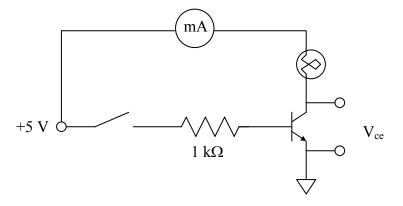
Activate the switch by inserting or removing the wire connecting the +5 V to the 1 k $\Omega$  resistor. Take note of the values of  $I_c$  and  $V_{ce}$  for the two cases
