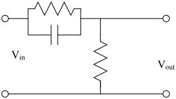
6. Build the LRC circuit below. Measure the transfer function of this filter. What is the FWHM of the transfer function? How does this compare to the RC bandpass filter you designed in your homework assignment? Which might be considered more useful?
