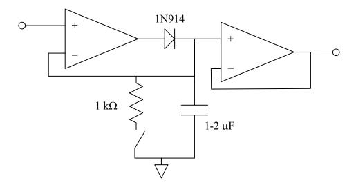
By varying the input voltage, verify the operation of this circuit. This circuit is best observed by watching the trace of the input and output signals on the oscilloscope using a 0.5 s/div timebase.
