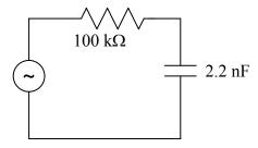
b. Set the generator to a  $\sim$  400 Hz square-wave and adjust the amplitude and DC offset so that the output switches from 0 to 1.5 V.
