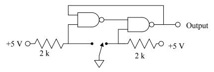
Use a wire as the switch. Describe the action of this switch, using your logic probe to test the output. Use what you've learned about digital logic to explain to me in your report why this circuit works the way it does.
