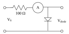
For the negative bias case, use the negative variable voltage source. Keep "an eye" on the resistor to make sure that you don't overload it. Plot your results for your write-up (I as a function of V). Prepare a second plot focusing on the region where the curve changes the most. What is the diode voltage drop in the forward direction? Estimate the forward and reverse resistances from this plot.
