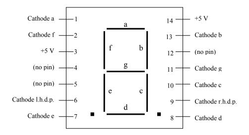
The lettering of the individual LEDs is industry standard and allows fairly easy interchange of components. The MAN-72 does not have any internal resistance in series with the LEDs so you  $\underline{MUST}$  have a small series resistor each cathode and the decoder output. Resistors of value  $400 - 700 \Omega$  will suffice. This prevents the forward bias current from getting to high and burning out the LEDs.
