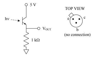
The DAQ card will not provide enough current to power the lightbulb so you will have to use a BJT as a power/current amplifier.
