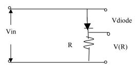
Note: when  $V_{in} > 0$ ,  $R_{diode} = 0$ , so  $V_{diode} = 0$  and  $V_R = V_{in}$  when  $V_{in} < 0$ ,  $R_{diode} = large$ , so  $V_{diode} = V_{in}$  and  $V_R = 0$
