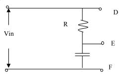
b) At what time will the voltage between E and F reach 0.0 V? (8 pts)  $V_{EF} = V_C = V_{in} - V_R = 0 = 3.00 \text{ V} - [3.00 \text{ V} - (-2.00 \text{ V})]e^{-t/(185000 \cdot 3.0 \text{ x} \cdot 10^{\circ} - 6)} \text{ or } 100/5.00 = e^{-t/(185000 \cdot 3.0 \text{ x} \cdot 10^{\circ} - 6)} \text{ or } 100/6.00 = -t/(185,000 \cdot 3.0 \text{ x} \cdot 10^{\circ}) \text{ or } t = (0.555 \text{ s})(-\ln 0.6)$  t = 0.28 s
