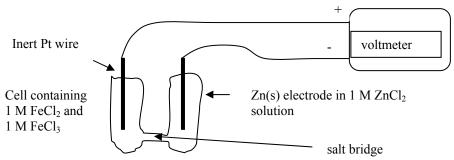
a) The voltmeter reads + 1.53 V (which is also E° for the net reaction). From this information write the reactions occurring at each half cell and a balanced net reaction. (8 pts)
