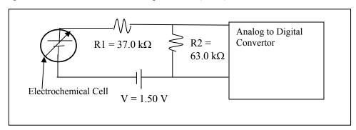
a) The binary number read by the A/D converter is 011000100110. What is the decimal number corresponding to this? (3 pts)
