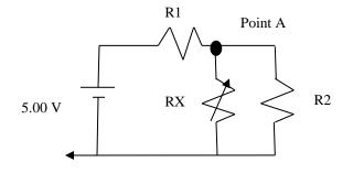
b) The current across resistor RX (6 pts)  $I_{R1} = I_{R2} + I_{RX} \text{ or } I_{RX} = I_{R1} - I_{R2} \text{ and } I_{R2} = V_A/R2 = 2.31 \text{ V}/370 \ \Omega = 0.00624 \text{ A}$  $I_{RX} = 0.0122 A - 0.00624 A = 0.0060 A$
