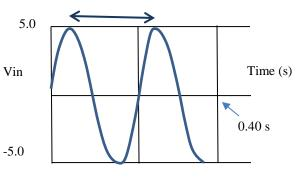
b) If the plot above represents a perfect sine wave and extends infinitely along the time axes, describe what a Fourier transform of it would look like. *If a sine wave, a single line at 5 Hz would show up.*
