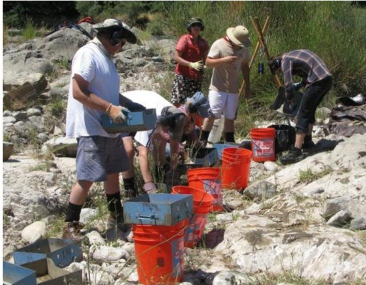
Figure 20: Bulk sample sieve line. The dried gravel was sorted by grain size with rocker sieves and size fractions were stored in 5 gallon buckets for individual weight measurements.
