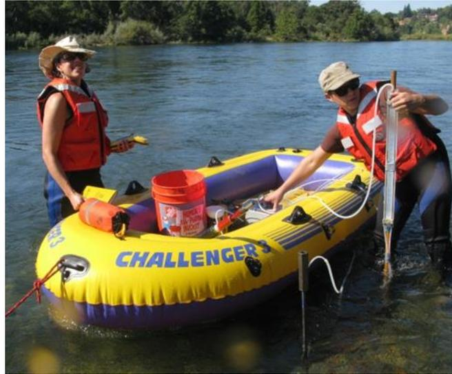
Figure 26: CSUS river crew students measuring up/downwelling conditions with boat, peristaltic pump, in-stream baffle (not pictured), 30cm deep well, and manometer board.
