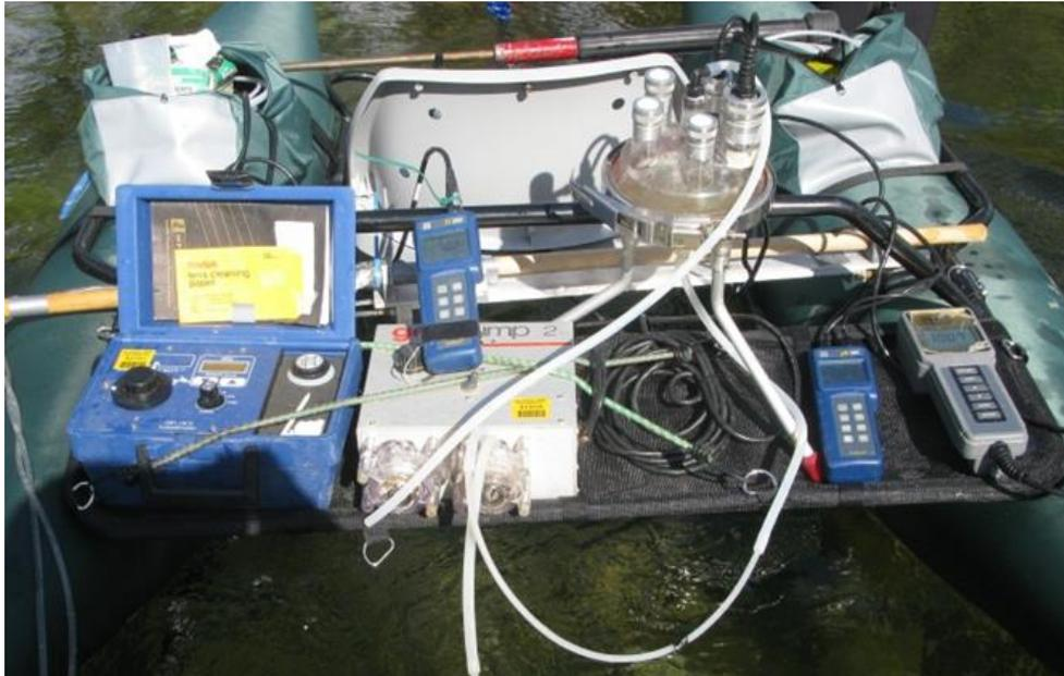
Figure 27: Sampling boat and equipment consisting of (from left to right) a DRT turbidity meter, an YSI model electrical conductivity meter atop the peristaltic pump, a flow thru cell, an YSI model pH meter, and a YSI 95 dissolved oxygen meter.
