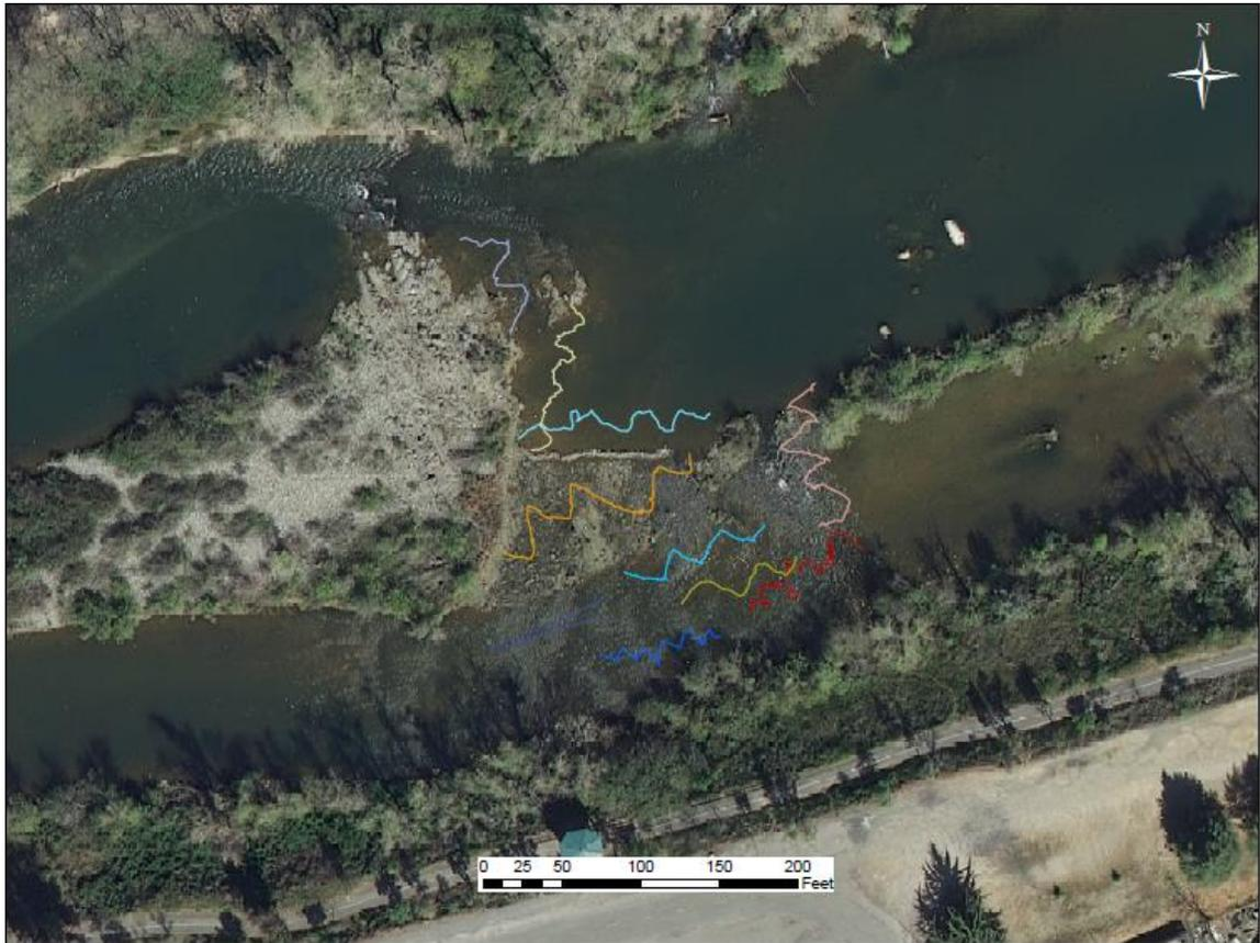
Figure 30: Transect paths of the pebble counts collected at Cottonwood/Hatchery Riffle. The colored transects correspond to the colored lines on the Cottonwood Hatchery Riffle Pebble Count Distribution.
