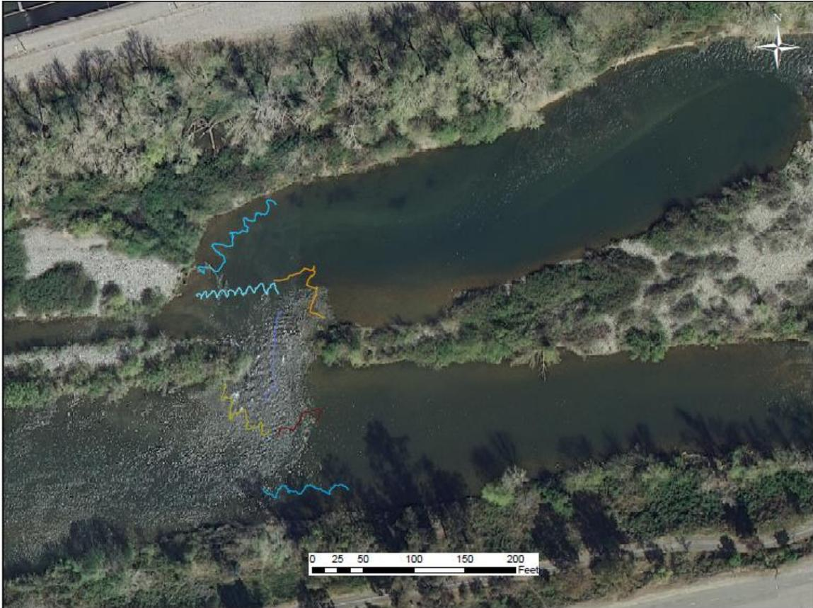
Figure 32: Transect paths of the pebble counts collected at Upper Auditorium Riffle. The colored transects correspond to the colored lines on the Upper Auditorium Riffle pebble count distribution.
