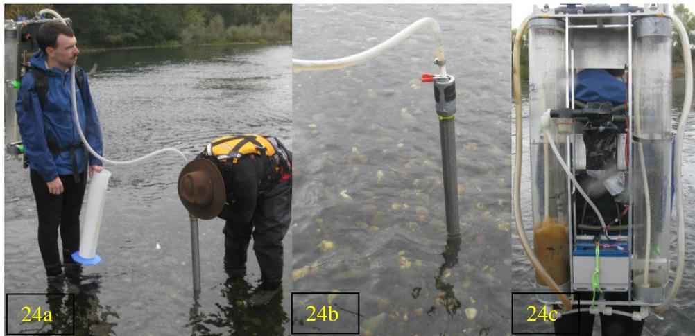
Figure 24: Barnard McBain standpipe test. 24a) Listening for the “slurping” sound to establish a depth to water. 24b) Standpipe with 1 inch drawdown test being conducted. 24c) Backpack pump with reservoirs for collecting the sample volume.
