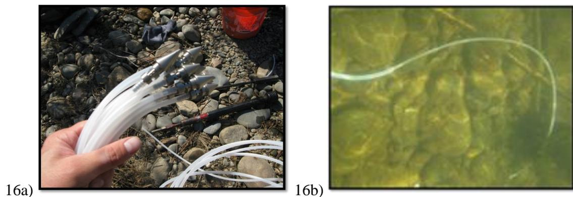
Figure 16: 16a) A handful of mini-piezometer tips is ready for installation in the river. 16b) Mini-piezometer installed at 30cm depth, with plastic tubing that allows sampling of hyporheic conditions from a discrete interval in the subsurface.
