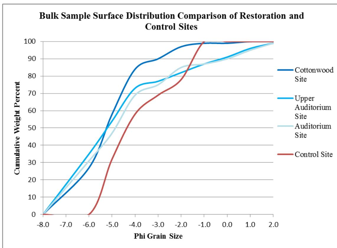
Figure 55: Comparison graph of the mean surface bulk sample data from all sites studied.
