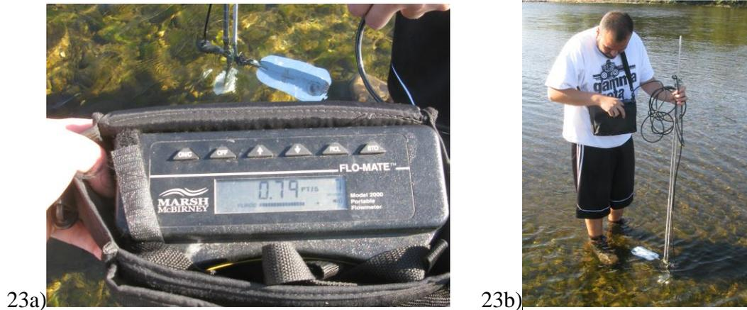
Figure 23: 23a) Marsh McBirney current meter used to measure flow velocity in the river. 23b) Sacramento State student demonstrating use of the current meter.
