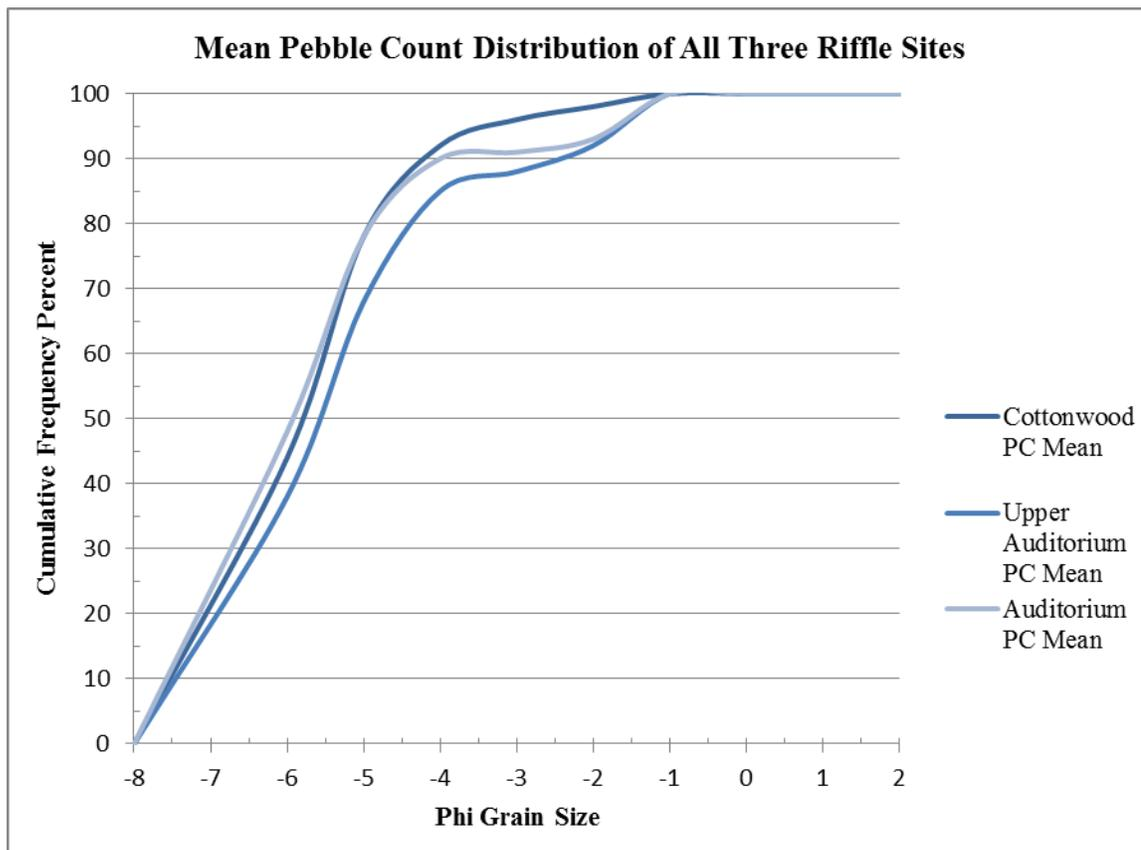
Figure 36: Pebble count distribution graph showing the mean pebble count line for each restoration site.
