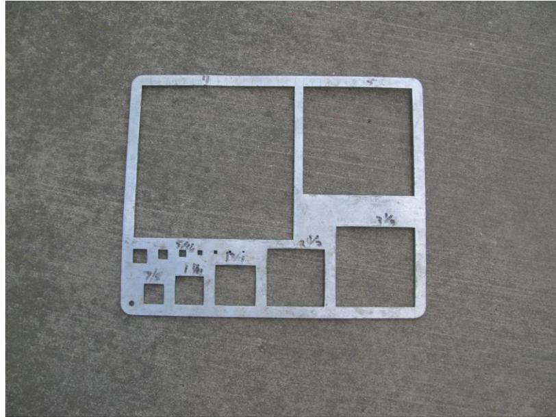
Figure 17: Gravelometer used to measure the intermediate axis of a grain during the pebble count transects.
