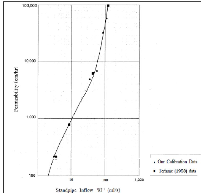
Figure 25: Permeability vs. standpipe inflow rate calibration curve. The collected standpipe inflow rate from a particular test is compared to the chart to reveal a permeability value. Image from Barnard McBain (1994).
