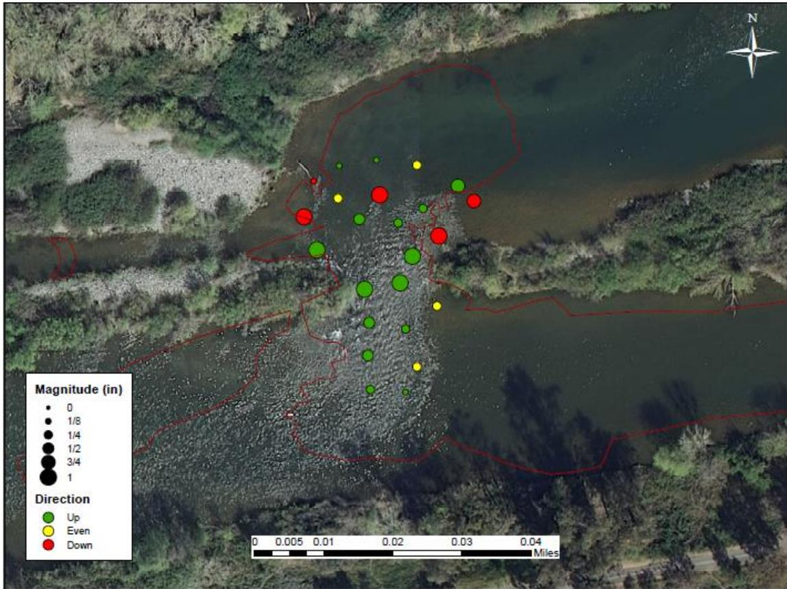
Figure 74: Upwelling/Downwelling map of the Upper Auditorium Riffle.
