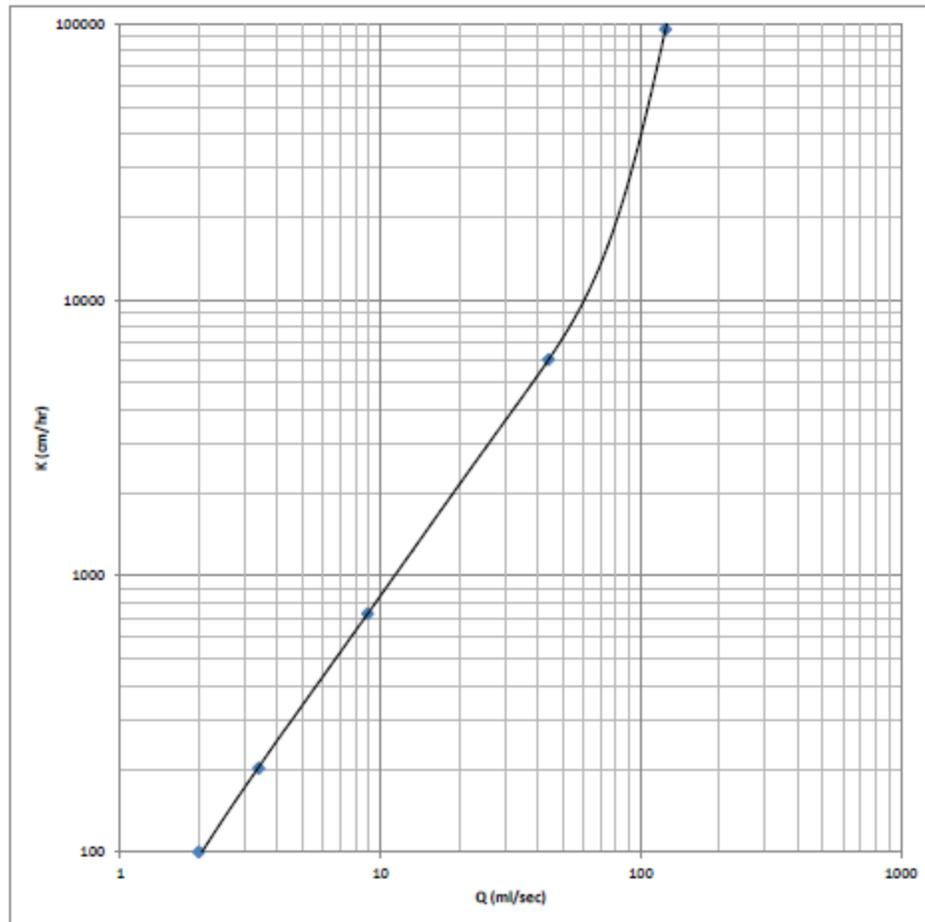
Figure 59: Permeability vs. standpipe inflow rate calibration curve. The collected standpipe inflow rate is compared to the chart to reveal a permeability value. Image from Barnard McBain (1994).
