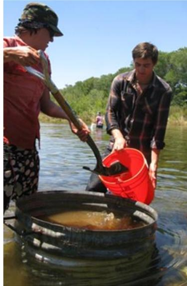
Figure 19: Bulk sample collection technique using corrugated metal tube and 5 gallon bucket. The metal tube prevents the loss of fine material.
