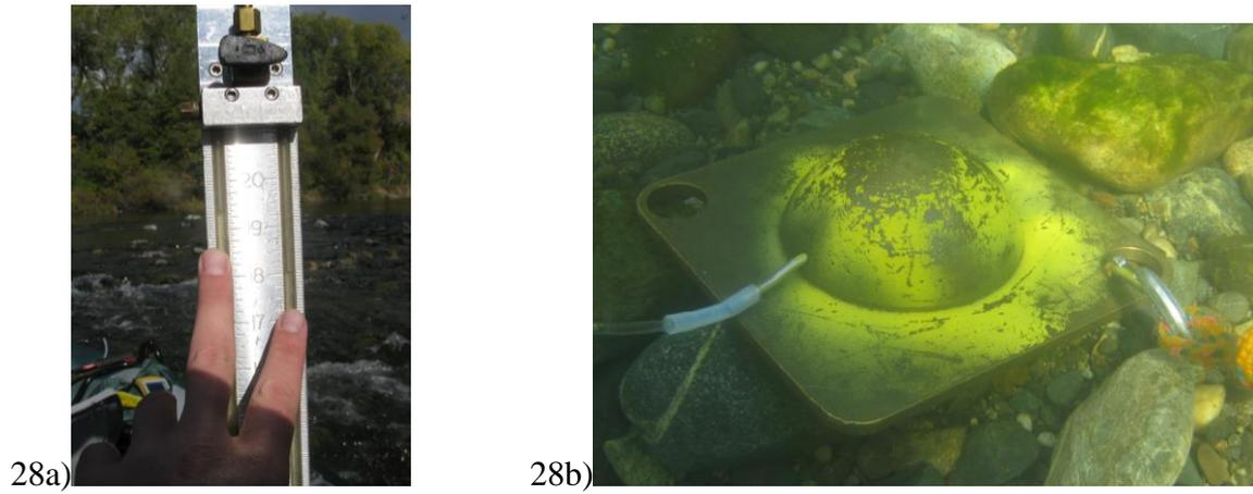
Figure 28: 28a): Manometer board showing pressure head differences between the 30cm deep well and the in-stream baffle. The left (well) side is higher pressure than the right (baffle) side indicating upwelling conditions. 28b): In-stream baffle used during up/downwelling measurements to compare the pressure of the river to the pressure at 30cm deep in the subsurface. The baffle removes the effect of surface flow.
