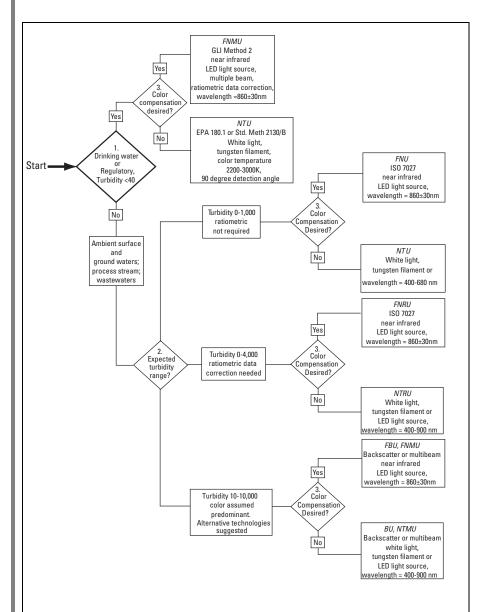
**Figure 6.7-2.** Decision tree to determine appropriate instrumentation designs for intended turbidity measurements.
