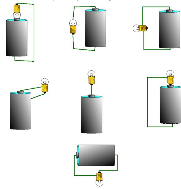
Work with a partner to check which ones will light. Circle the ones that light up. CAREFUL: DO NOT TOUCH THE BARE WIRE OR THE METAL PARTS OF THE BULB OR BATTERY WHEN DOING THIS EXPERIMENT: DIRECT CONTACT MAY RESULT IN A SKIN BURN.
