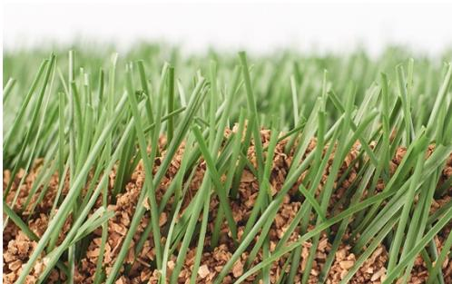
Another option is a non-toxic thermoplastic elastomer (TPE). This product is made of a plastic material which mimics the feel of rubber infill allowing for adequate cushion and safety of the athletes.
