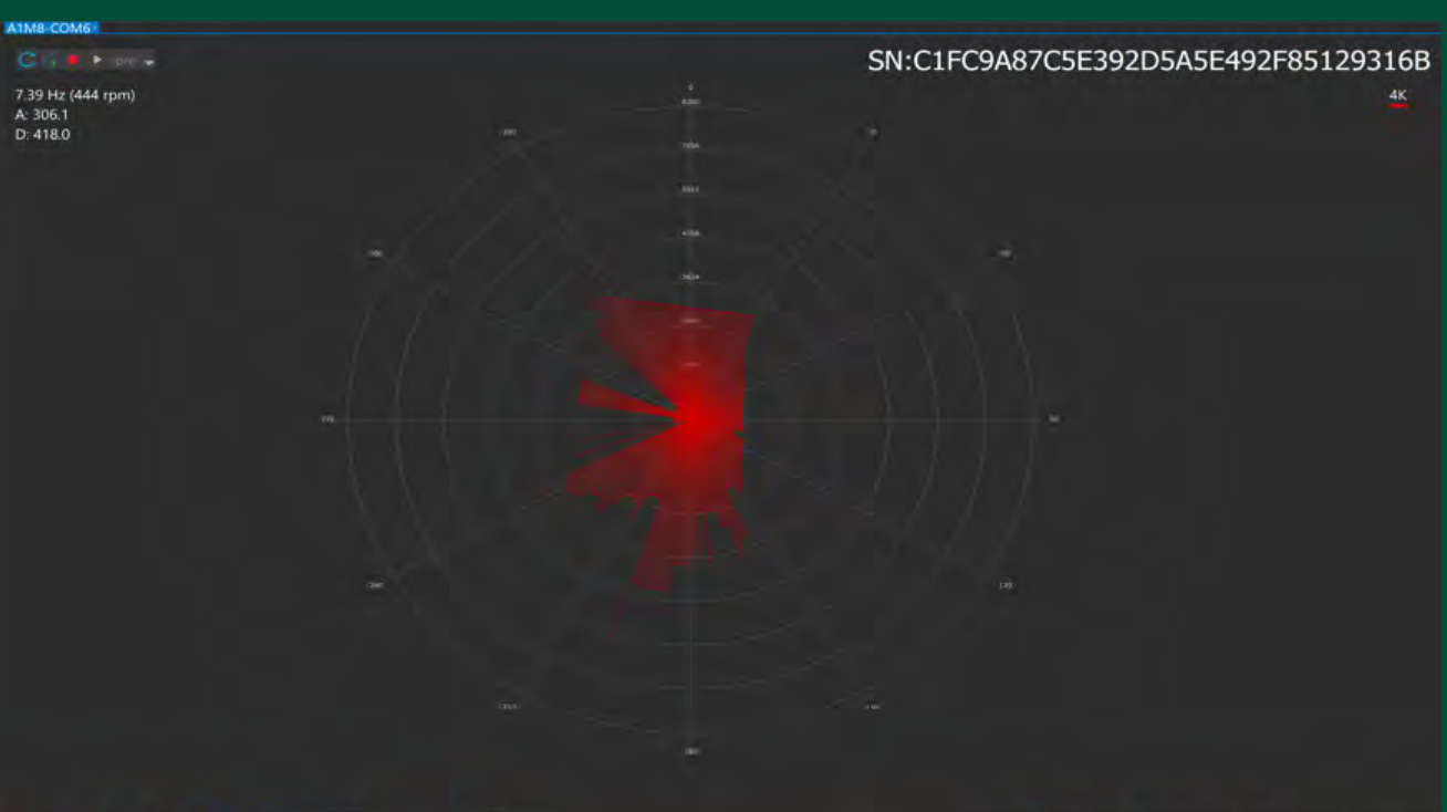
Figure 3: (left) the outline of the environment is scanned by RPLIDAR A1 sensor.
