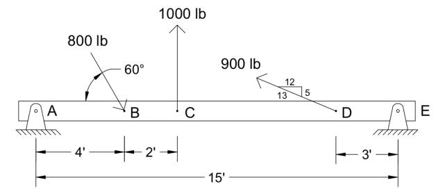
3. Replace the loading system by an equivalent resultant force and specify where the resultant's line of action intersects line AC, measured from point A.
