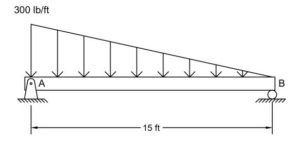
2. Determine the magnitude and location of the resultant force, measured from Point A.
