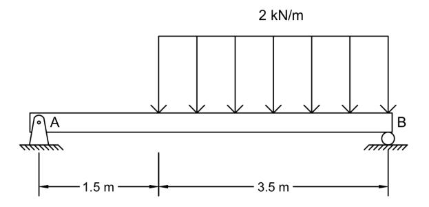
3. Determine the magnitude and location of the resultant force, measured from Point B.
