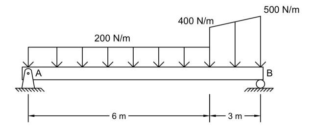
4. Determine the magnitude and location of the resultant force, measured from Point B.
