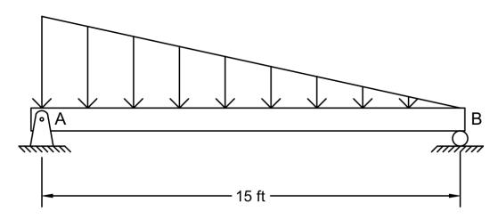
3. Determine the magnitude and location of the resultant force, measured from Point B.
