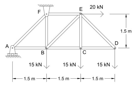
2. Using the method of sections, determine the force in members CD, BF, and EF of the truss shown. Indicate whether the members are in tension or compression.
