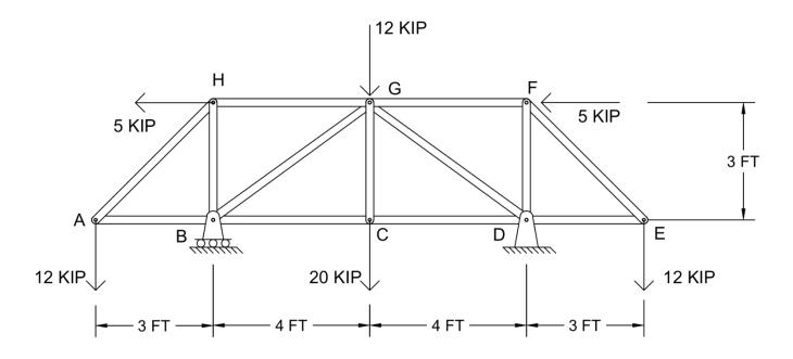
3. Using the method of sections, determine the force in members GF, DG, and CG of the truss shown. Indicate whether the members are in tension or compression.
