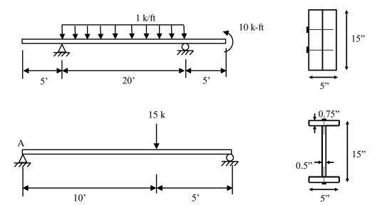
3. Determine the shear force in each nail if the nails are spaced 12 inches apart along the length of the beams below.
