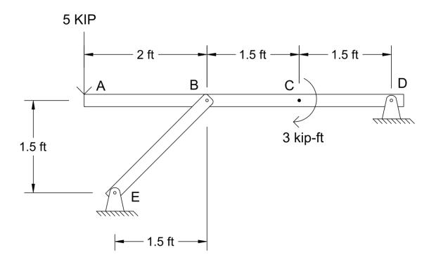
2. Refer to the figure below. Draw a FBD of the entire frame, a FBD of member AC, and a FBD of member BD. Identify any two-force members. Determine the support reactions at A and D.
