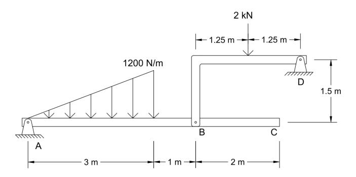
3. Refer to the figure below. Determine the support reactions at A and B.
