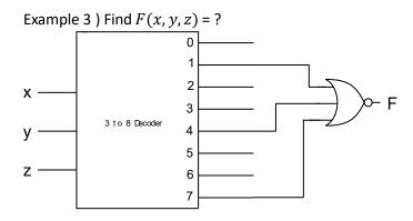
Since a NOR gate connected to output  $F(x, y, z) = \sum (0.2, 3.5, 6)$
