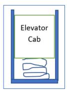
8. The 2000 kg elevator cab fell from a height of 15 meters above the top of the elevator shaft spring. The spring has stiffness constant 10,0000 N/m. Determine the spring compression when the elevator cab's vertical speed reaches 0 meters/sec.
