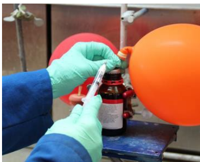
Figure 5: Hold plunger and force excess reagent back into the bottle.
