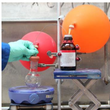
Figure 9: Arrangement of reagent bottle and receiving flask.
