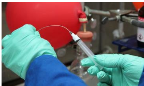
Figure 4: Prepared syringe demonstrating the bend in the needle and keeping the inserted side secure.
