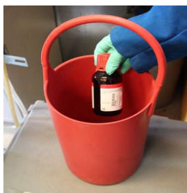
Figure 2 Secondary containment for transport of pyrophorics.
