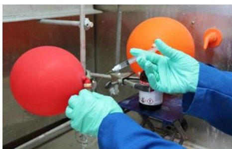
Figure 7: Transfer of reagent into receiver flask.
