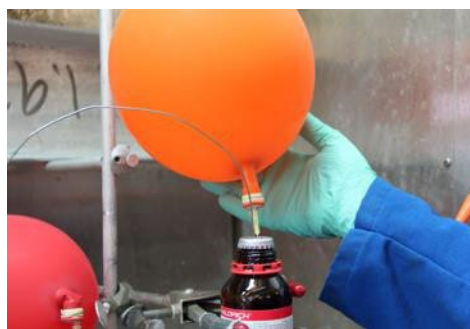
Figure 8: Insert the cannula into the reagent bottle.
