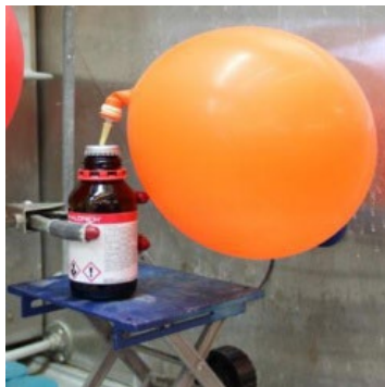
Figure 3 Secured reagent bottle with positive pressure
