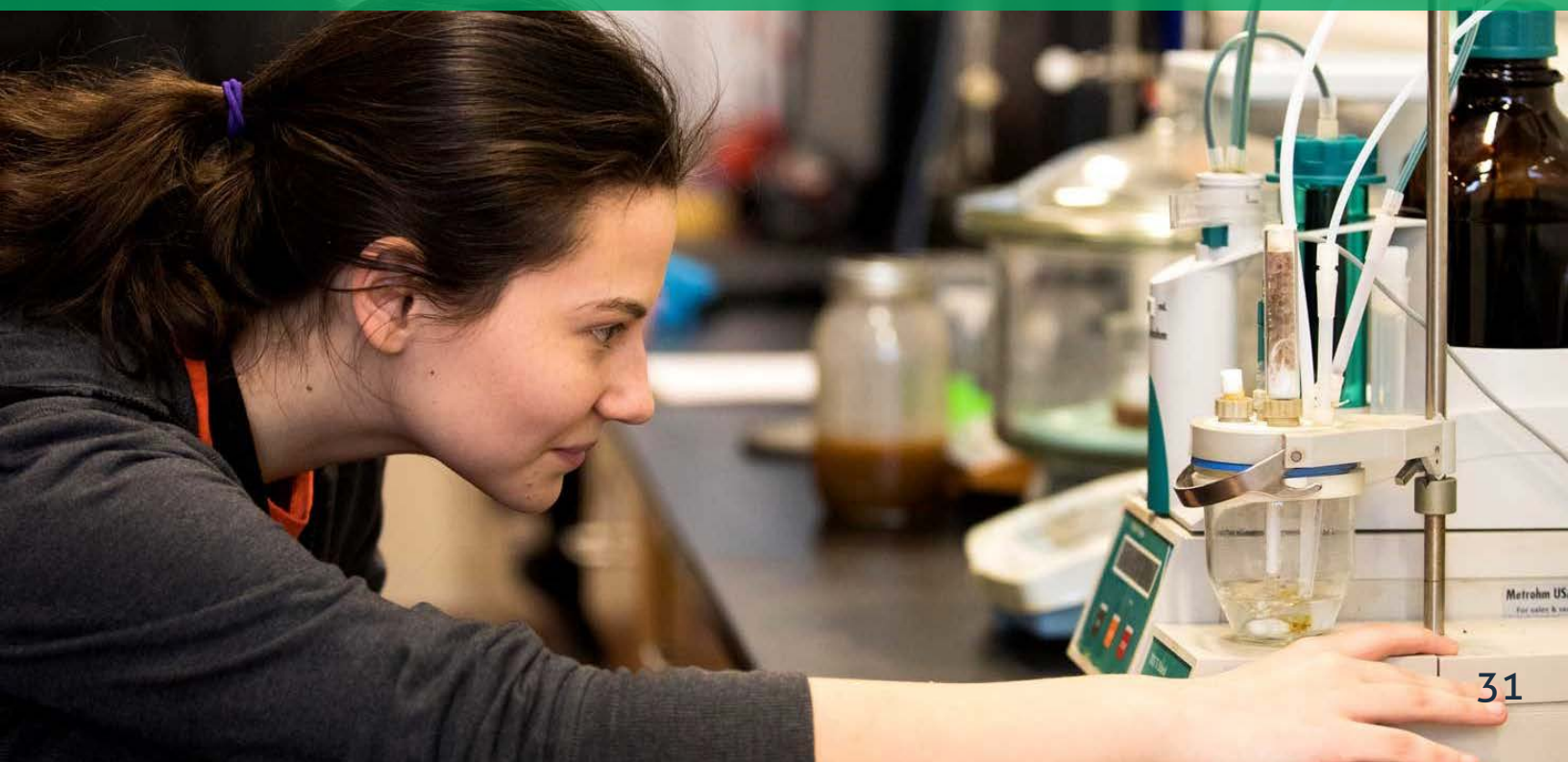
Student running a Karl Fischer titration QA/QC test for water levels in finished biodiesel batches at Loyola University Chicago.
