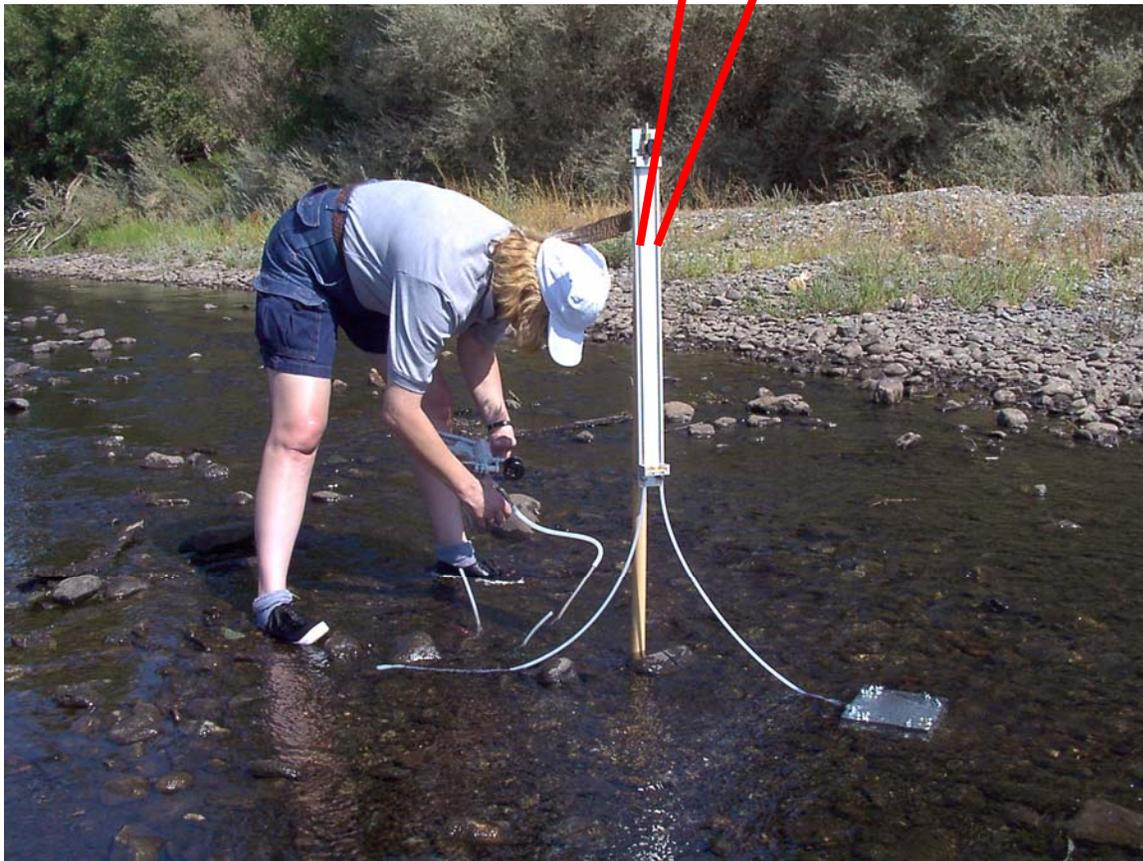
Figure 20: A manometer board is attached to subsurface sampling tubes to measure differences in hydraulic head. Higher head in the stream indicates losing conditions, although gaining conditions (upwelling) are common at the downstream ends of riffles and gravel bars. A baffle box is used to restrict current flow and minimize pressure differences past the open end of the tube.
