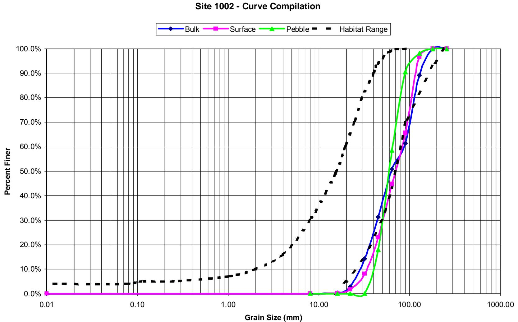
Figure 24: Sieve analysis for Sailor Bar site 1002. Sample is slightly coarse, but does not have significant armoring. This is an improvement over pre-project conditions.
