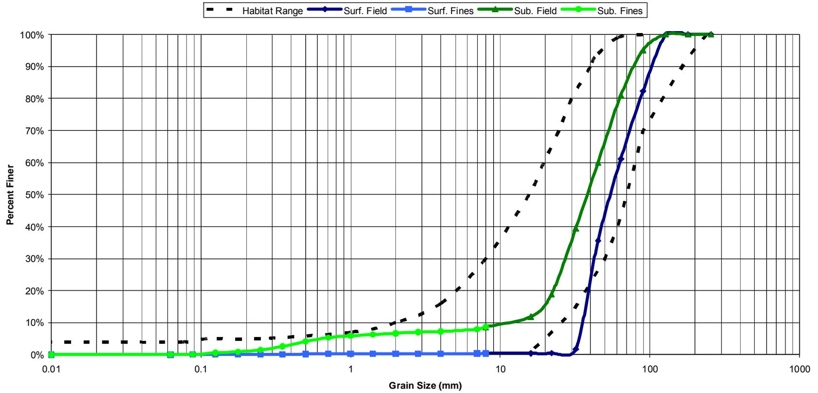
Figure 9: Grain size analysis compilation curve- surface and subsurface samples.
