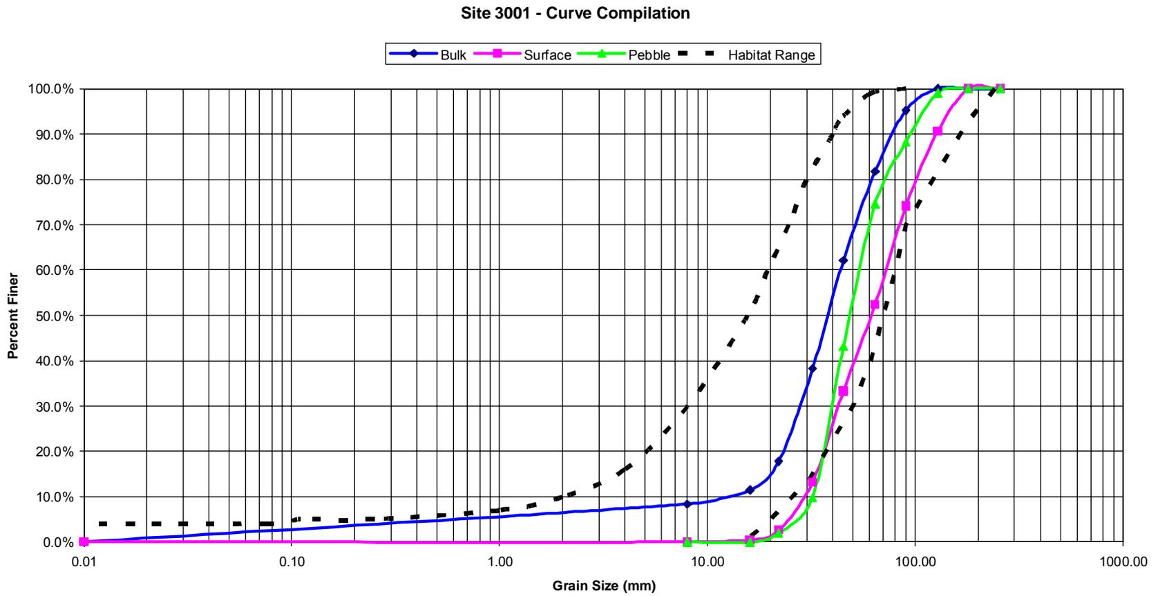
Figure 27: Sieve analysis for Lower Sunrise Access site 3001. Comparison of surface and subsurface grain size distribution shows coarser surface layer (armoring).
