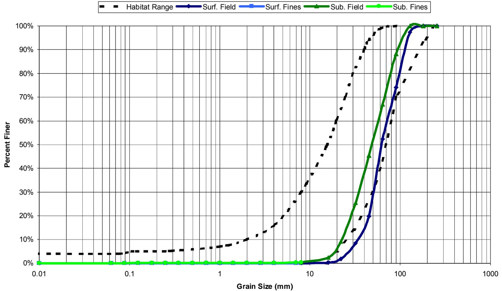
Figure 25: Sieve analysis for Sailor Bar site 1003. Sample is slightly coarse, but does not have significant armoring. This is an improvement over pre-project conditions.
