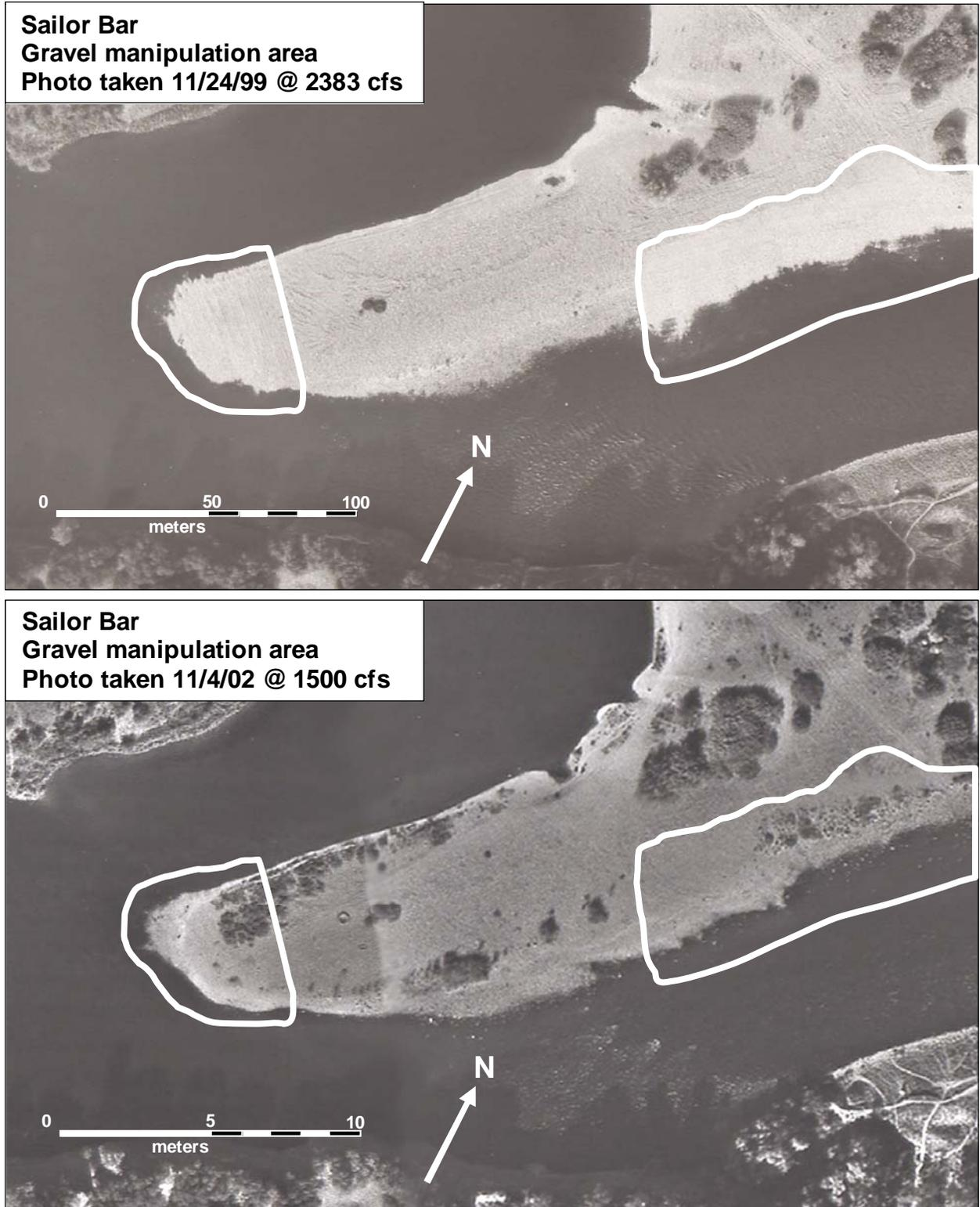
Figure 4: Sailor Bar immediately after gravel emplacement (top picture) and three years later (bottom picture)
