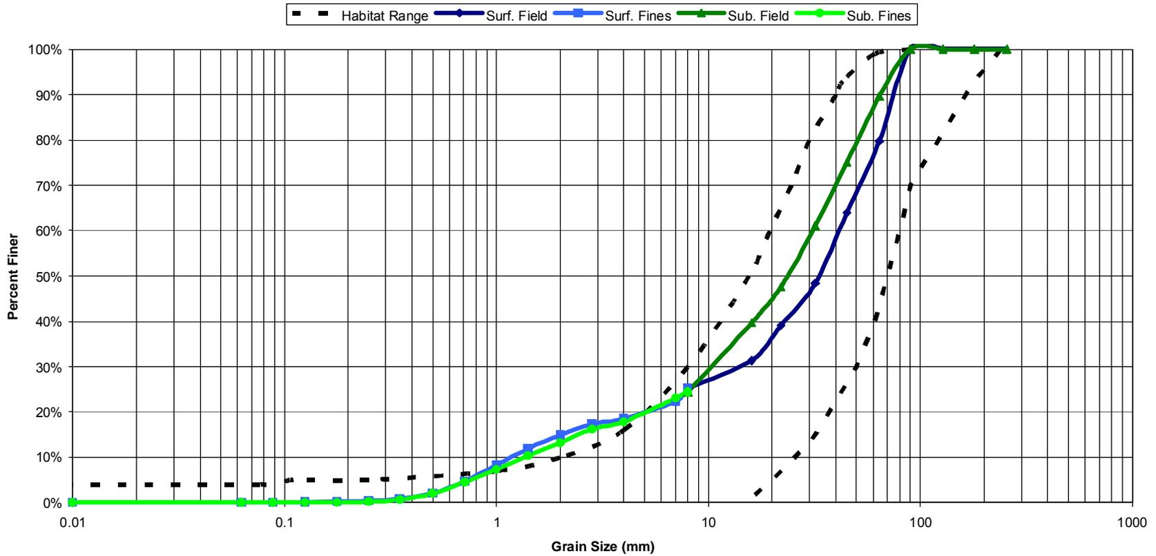
Figure 30: Sieve analysis for Lower Sunrise Access site 3004. Comparison of surface and subsurface grain size distribution shows little or no armoring, but there is an excess of fine sediment at this site that might limit spawning habitat.
