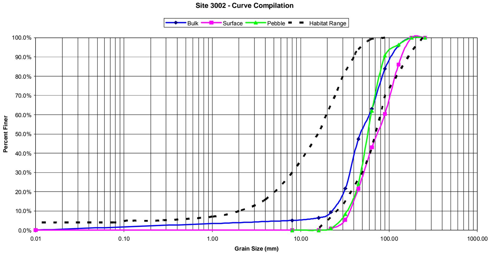
Figure 28: Sieve analysis for Lower Sunrise Access site 3002. Comparison of surface and subsurface grain size distribution shows coarser surface layer (armoring).
