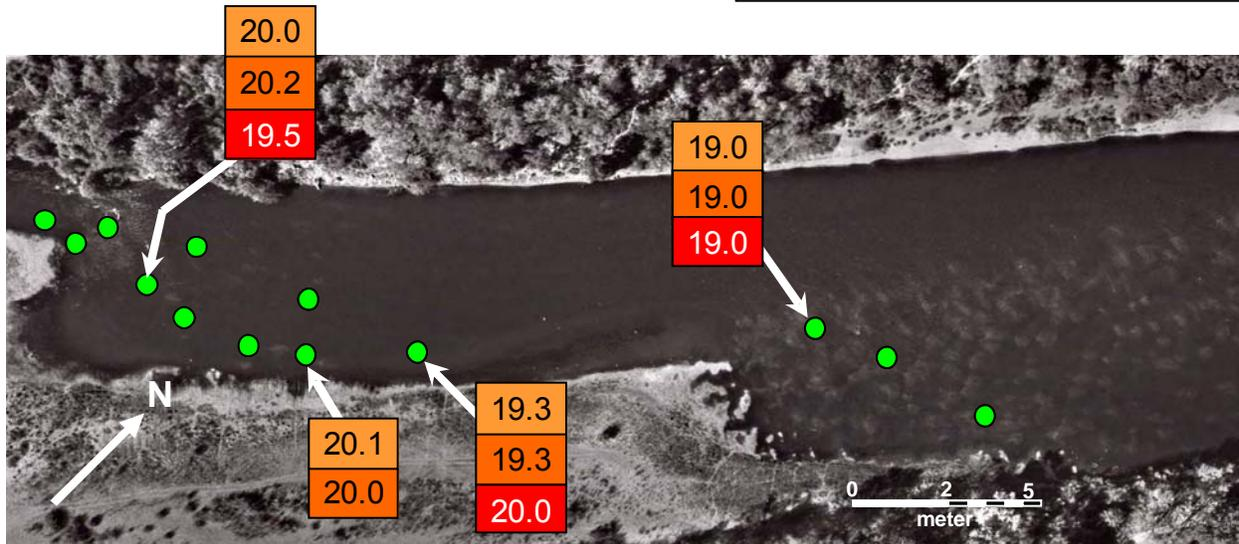
Figure 40: Temperature measurements from Lower Sunrise Access, collected when river temperature = 15.9°C. Field parameters (including temperature) are measured in a flow-through cell, and temperature may not be representative of conditions in the gravel.
