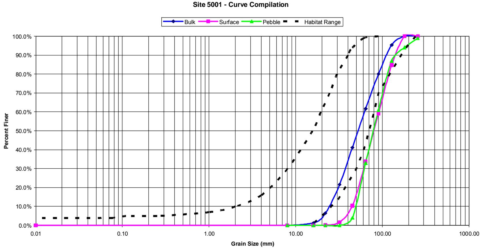
Figure 32: Sieve analysis Sacramento Bar site 5001. Comparison of surface and subsurface grain size distribution shows slight armoring and generally coarse grain size distribution.
