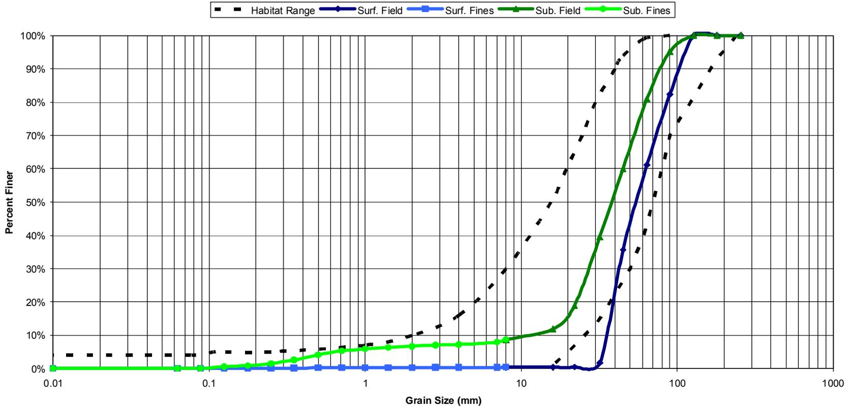
Figure 29: Sieve analysis for Lower Sunrise Access site 3003. Comparison of surface and subsurface grain size distribution shows coarser surface layer (armoring), although grain size distribution is generally within the acceptable range.
