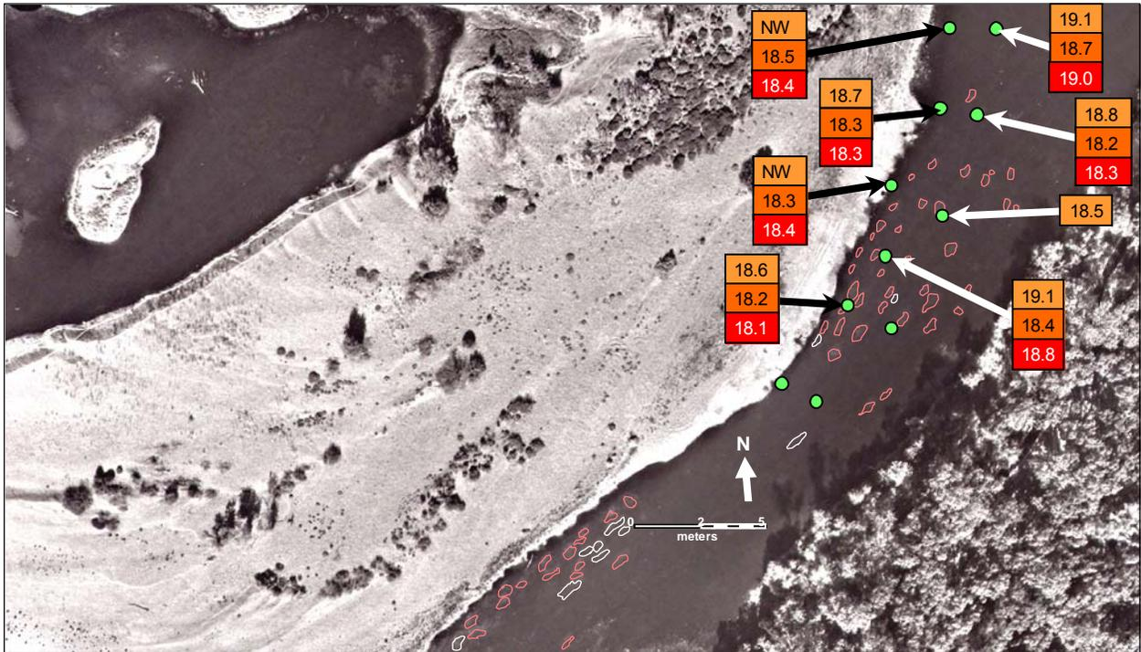
Figure 18: Temperature measurements from Sacramento Bar, when river temperature = 15.9°C. Temperature is measured in a flow-through cell, and may not be representative of conditions in the gravel.
