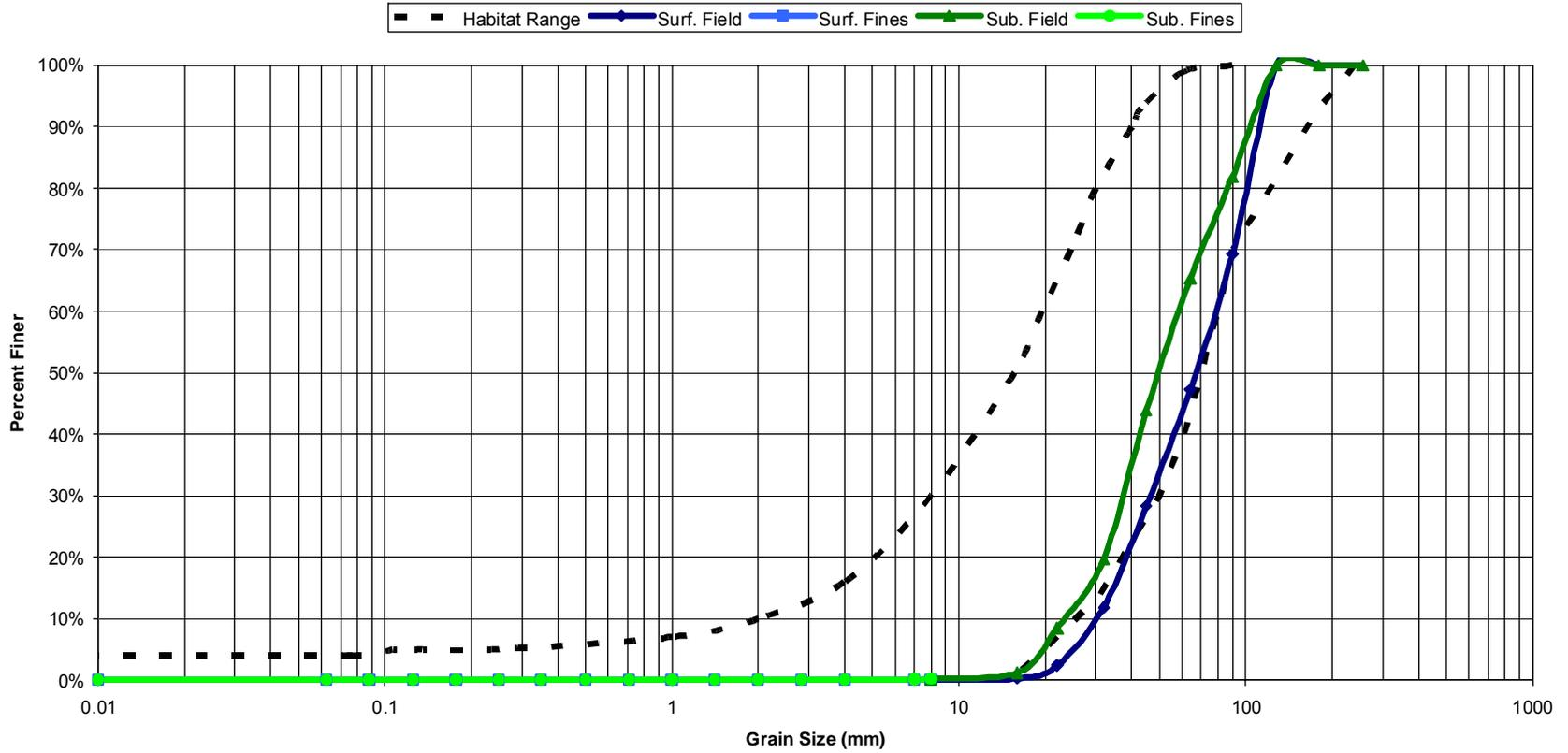
Figure 34: Sieve analysis Sacramento Bar site 5003. Comparison of surface and subsurface grain size distribution shows coarse grain size distribution, and very slight armoring.
