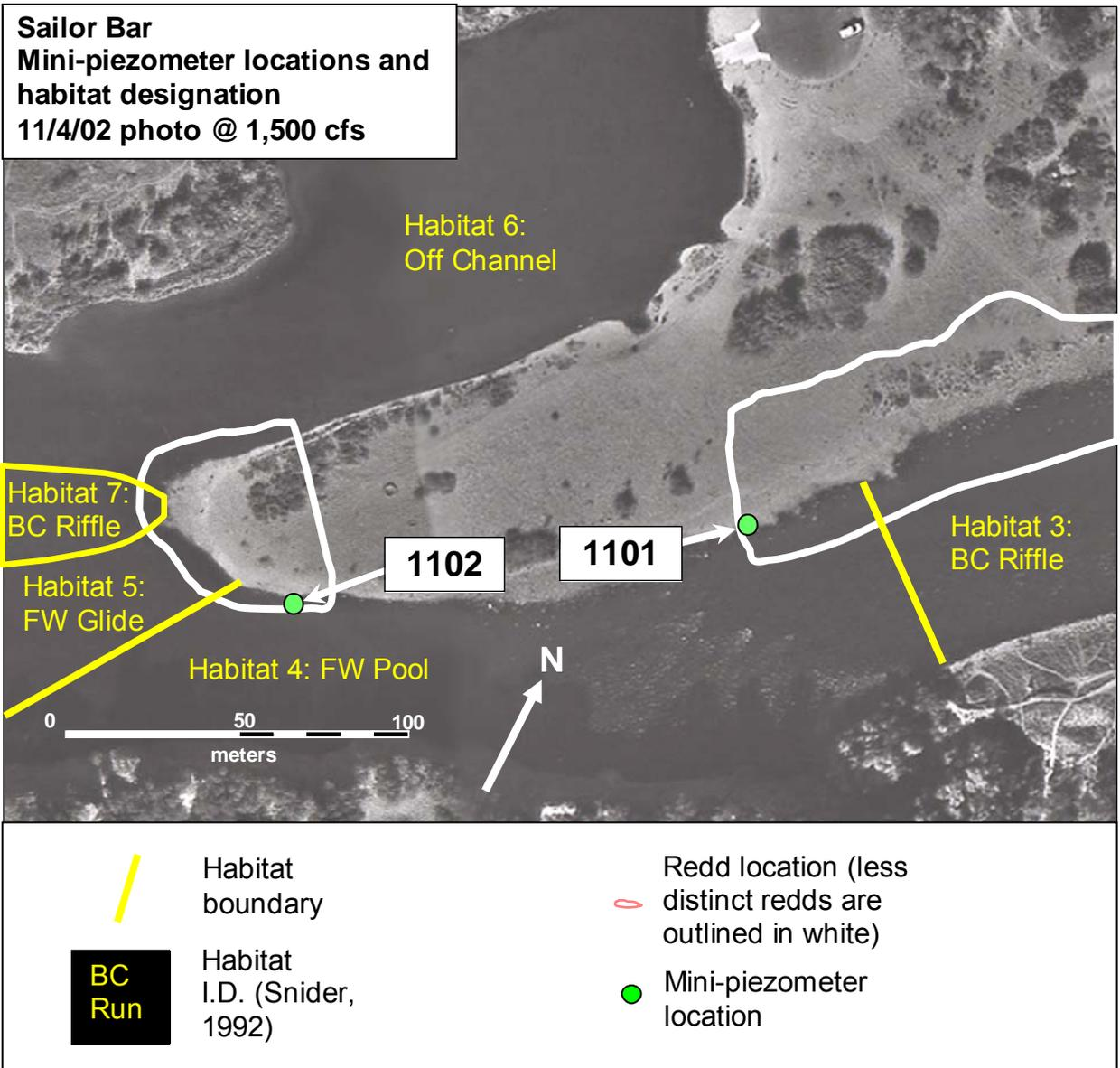
Figure 13: Mini-piezometer locations and habitat units at Sailor Bar. Gravel enhancement areas are outlined by white lines. Additional piezometers will be installed as part of the 2003/2004 gravel assessment project.
