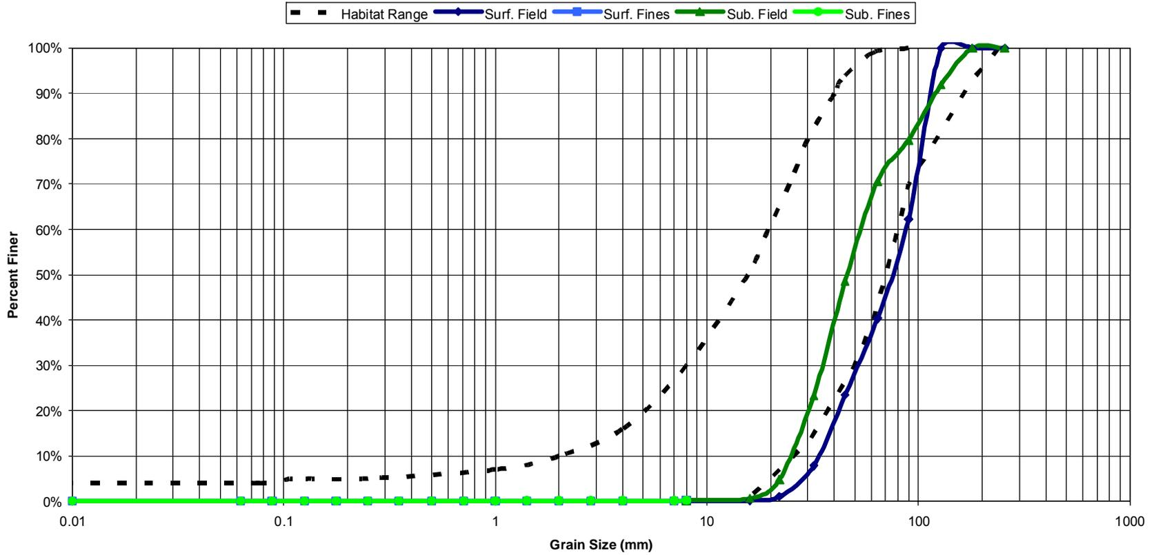
Figure 35: Sieve analysis Sacramento Bar site 5004. Comparison of surface and subsurface grain size distribution shows coarse grain size distribution with some surface armoring.
