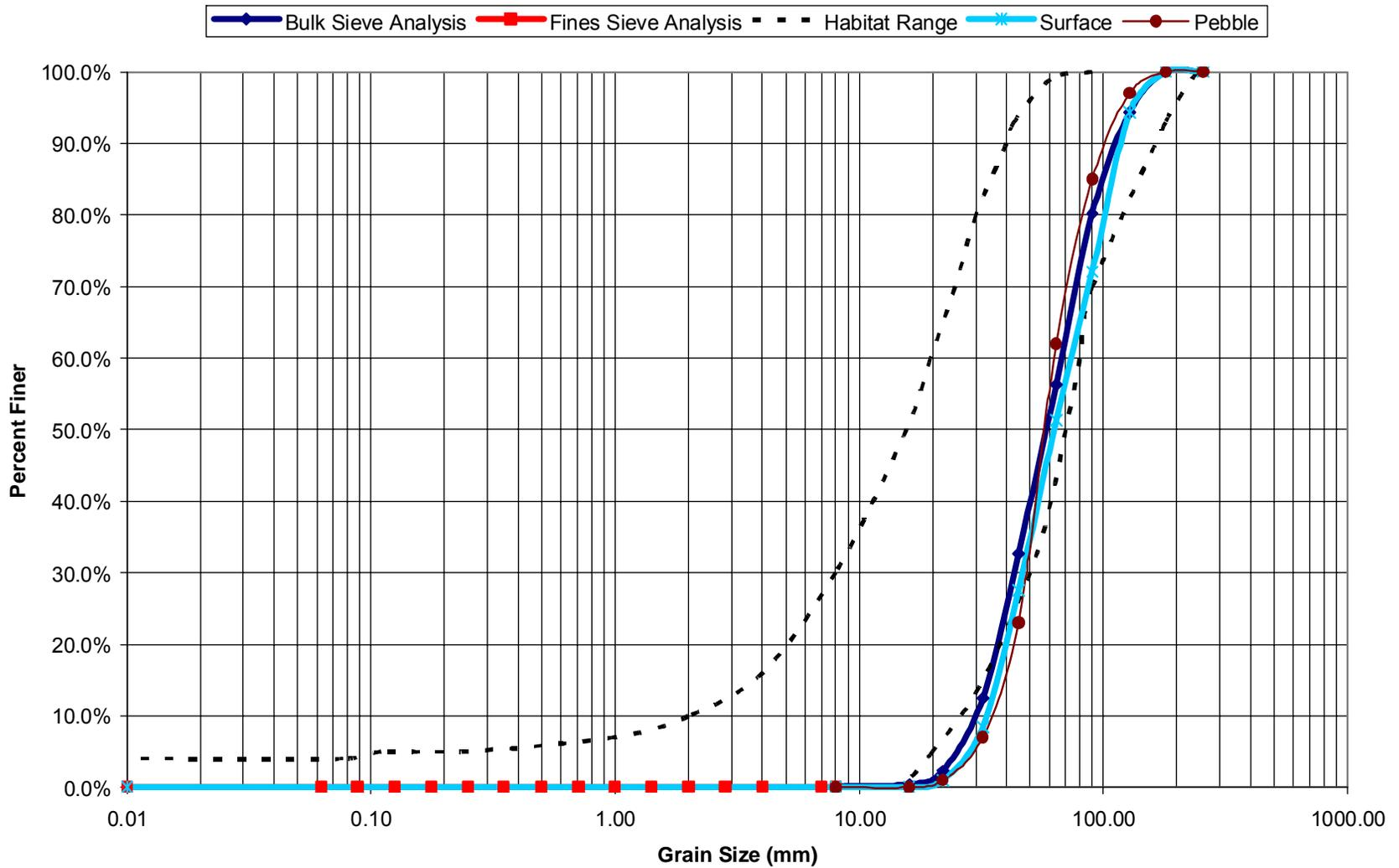
Figure 33: Sieve analysis Sacramento Bar site 5002. Comparison of surface and subsurface grain size distribution shows coarse grain size distribution, but no appreciable armoring.
