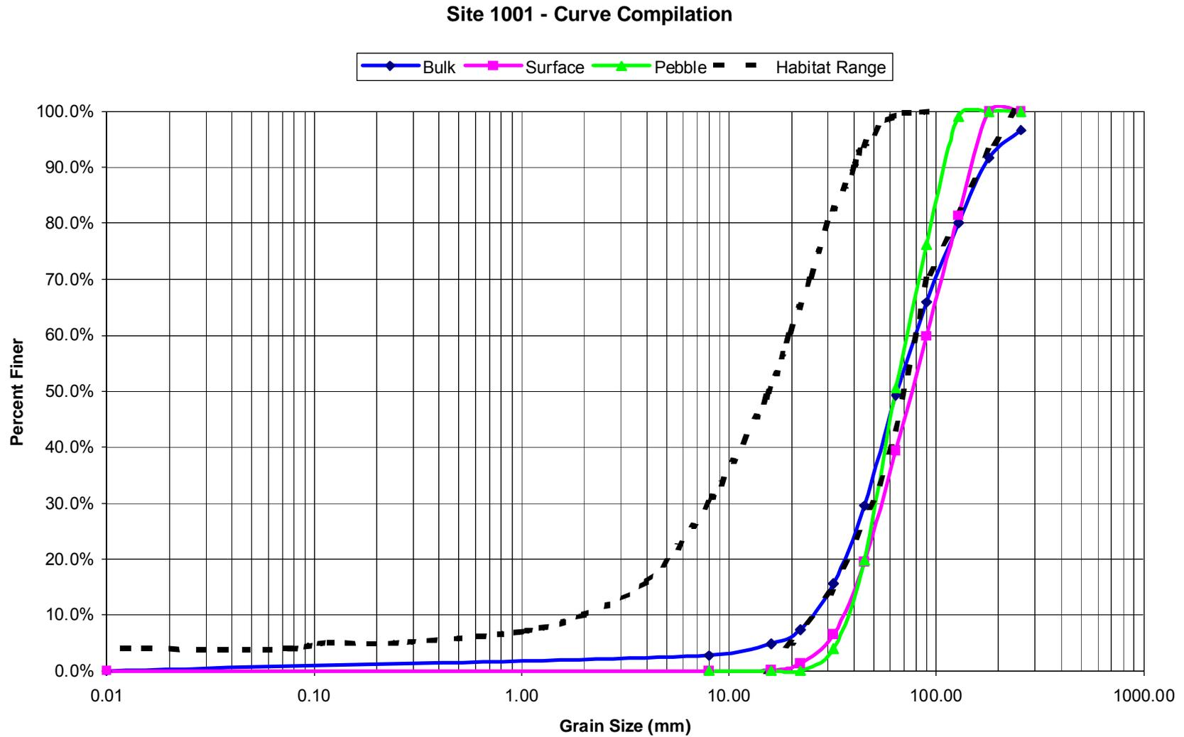
Figure 23: Sieve analysis for Sailor Bar site 1001. Sample is slightly course, but does not have significant armoring. This is an improvement over pre-project conditions.
