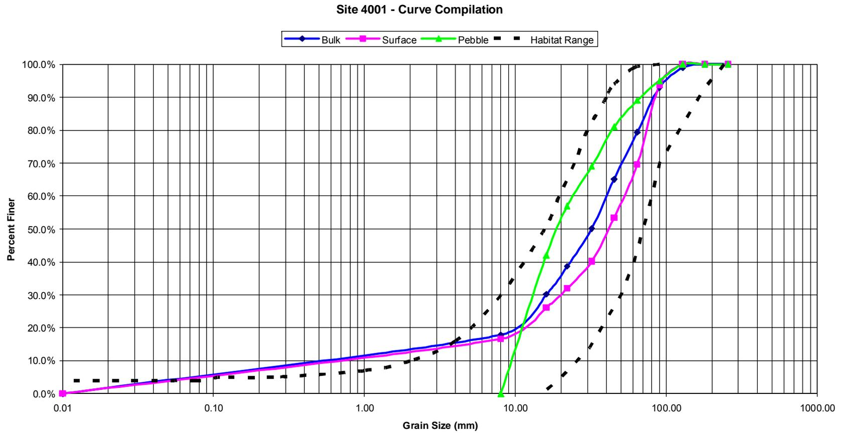
Figure 31: Sieve analysis for Lower Sunrise Access site 4001. Comparison of surface and subsurface grain size distribution shows slight armoring (coarsening) of the surface layer
