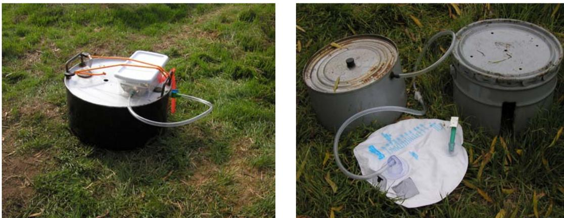
**Figure 4.** Large seepage meter with attached housing unit (left ) and small seepage meter with housing unit (right).
