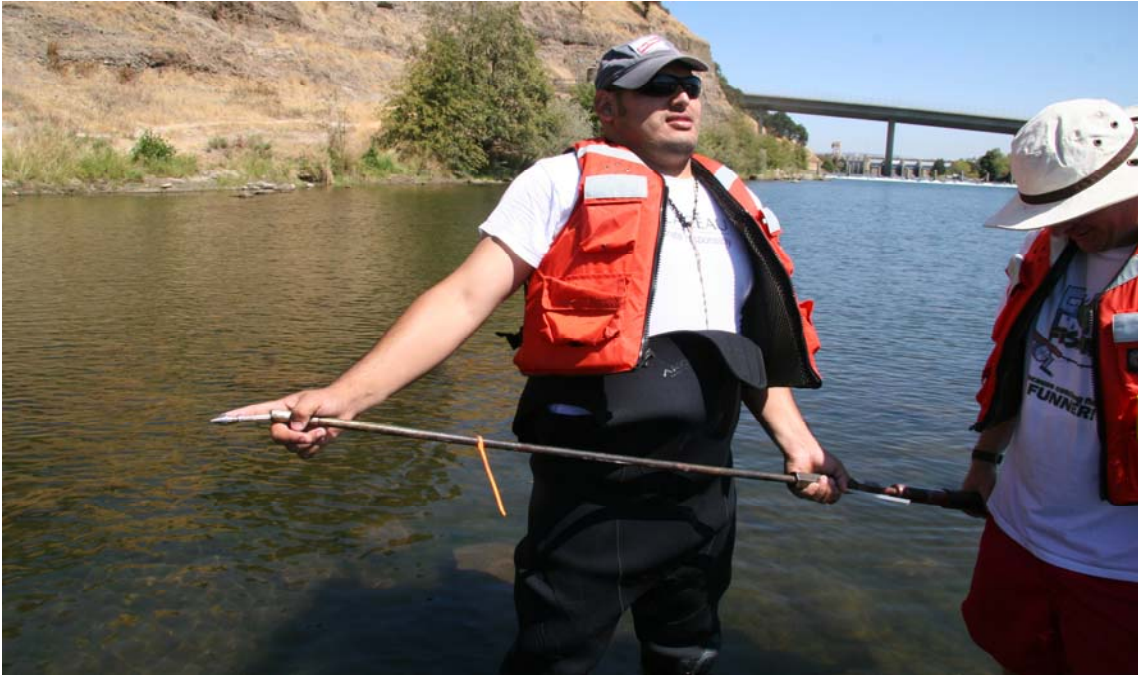
Figure 3: Picture of the piezometer tip and ¼ inch tubing used for mini piezometers. The mini piezometer is inside of the drive rod device used for mini piezometer installation.
