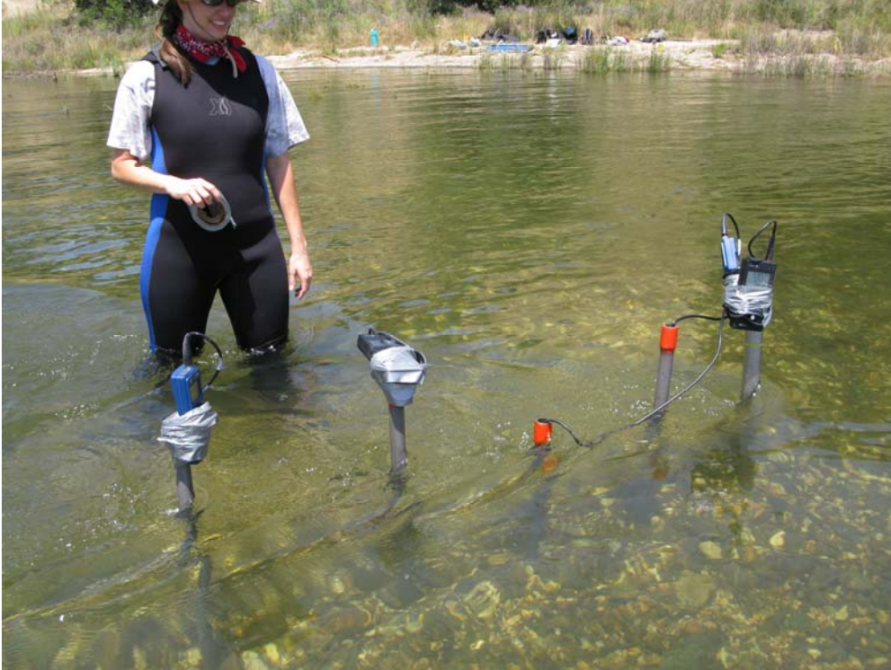
Figure 7: Picture showing the field set up of the permeability measurements.
