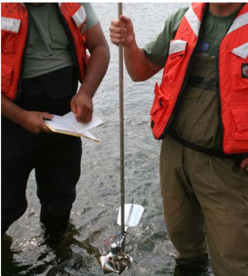
Figure 6: Picture showing the Price AA wading rod stream velocity measuring equipment.
