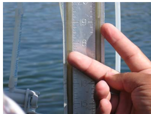
Figure 5: Picture of the manometer used for measuring the upwelling or downwelling for each mini piezometer. The photo to the right shows a close-up view of the different pressure heads from a measurement.
