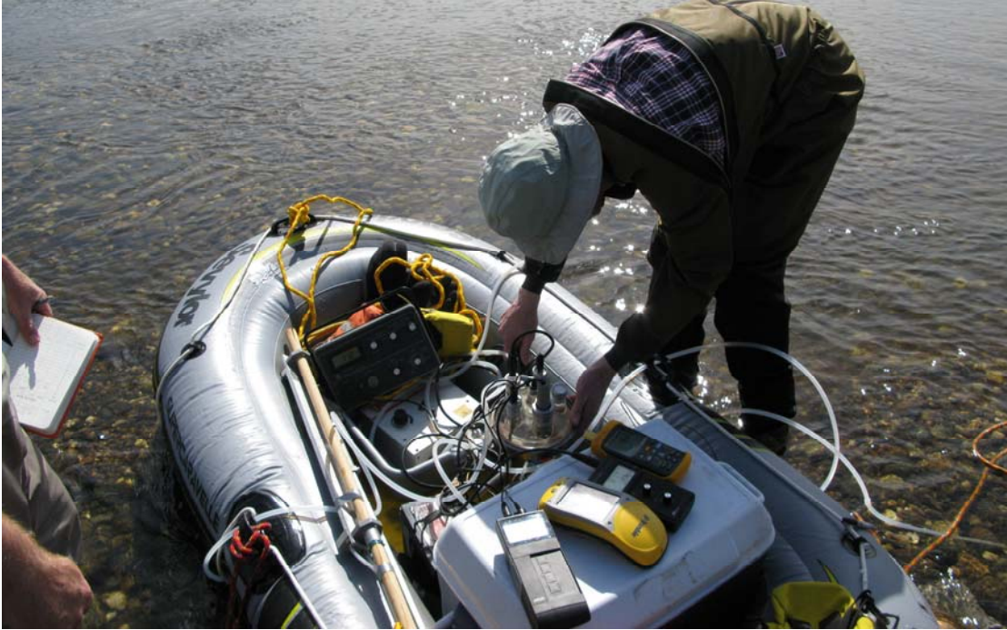
Figure 4: Picture of the field setup for the flow-through cell and water quality equipment.
