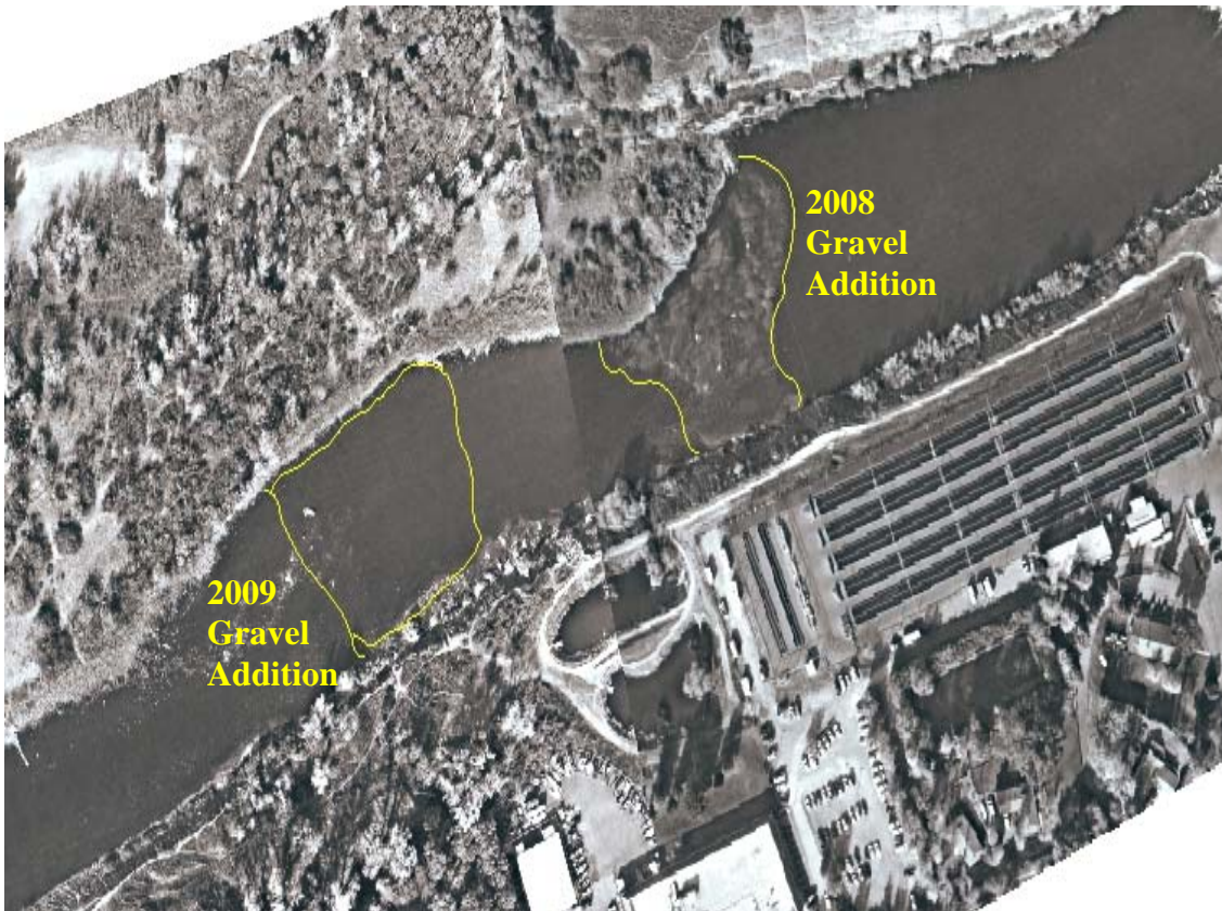
Figure 1: Map showing the outline in yellow of the gravel additions from 2008 and 2009. The Nimbus fish hatchery is in the lower right corner.
