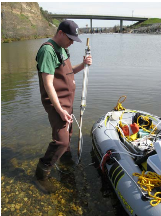
Figure 5: Picture of the manometer used for measuring the upwelling or downwelling for each mini piezometer. The photo to the right shows a close-up view of the different pressure heads from a measurement.
