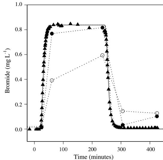
Fig. 3. Bromide concentrations measured in the channel (triangles) and those predicted by the OTIS model for the channel (solid line) and for the storage zone (dotted line), compared to values measured at downwelling hyporheic sites (filled circles) and upwelling sites (open circles) during the June 26, 1996 addition to the Oksrukuyik Creek.
