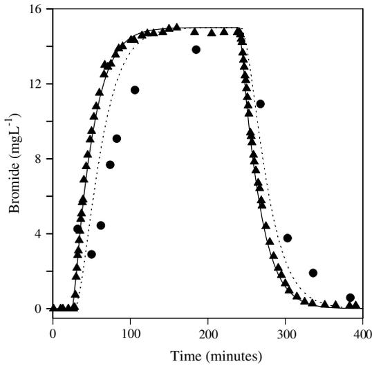
Fig. 5. Bromide concentrations measured in the channel (32 m reference point, triangles) and those predicted by the OTIS model (solid line), compared to Br concentrations predicted by the OTIS model (dotted line) in the storage zone at 37 m (dotted line) and measured in bead-bottom samples at 37 m (circles) during the July 6, 1995 addition to Innavait Creek.
