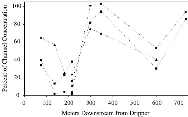
Fig. 6. Tracer concentrations within the hyporheic zone of Blueberry Creek as a percentage of channel plateau concentration. Samples were taken two to three hours after channel tracer concentration stabilized. All tracer additions were made during the 1994 field season; July 2 (circles), July 12 (squares), and August 6 (triangles).
