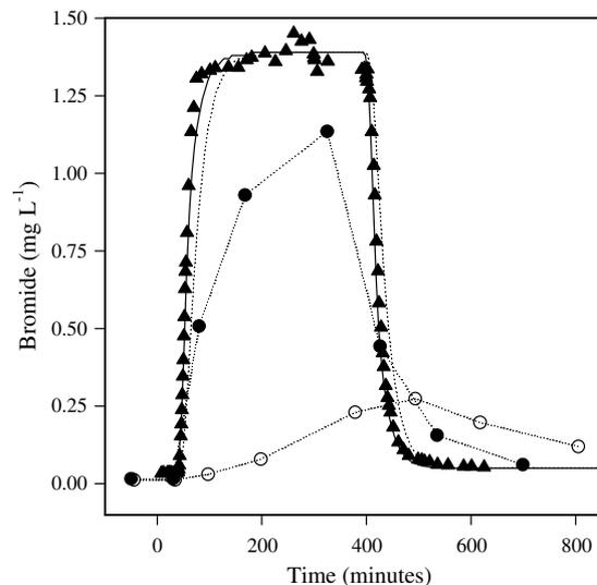
Fig. 4. Bromide concentrations measured in the channel (triangles) and those predicted by the OTIS model for the channel (solid line) and for the storage zone (dotted line), compared to values measured at downwelling hyporheic sites (filled circles) and upwelling sites (open circles) during the July 26, 1996 addition to the Kuparuk River.
