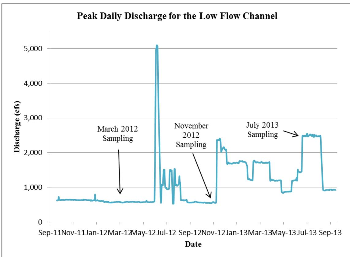
Figure 29: Hydrograph of the Low Flow Side Channel of the Feather River near Oroville, CA.
