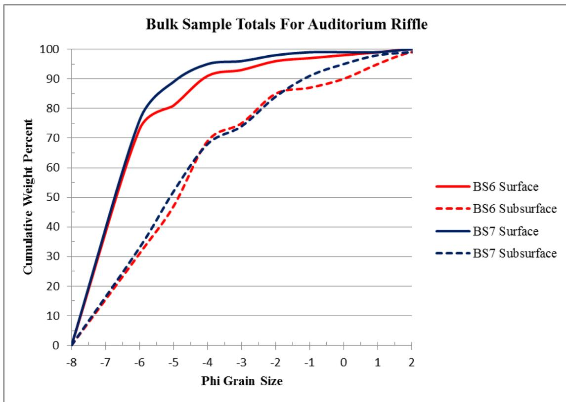
Figure 48: Bulk sample distribution chart for the Auditorium Riffle. Two bulk samples were conducted at the riffle complex and are separated into surface and subsurface sample sizes.
