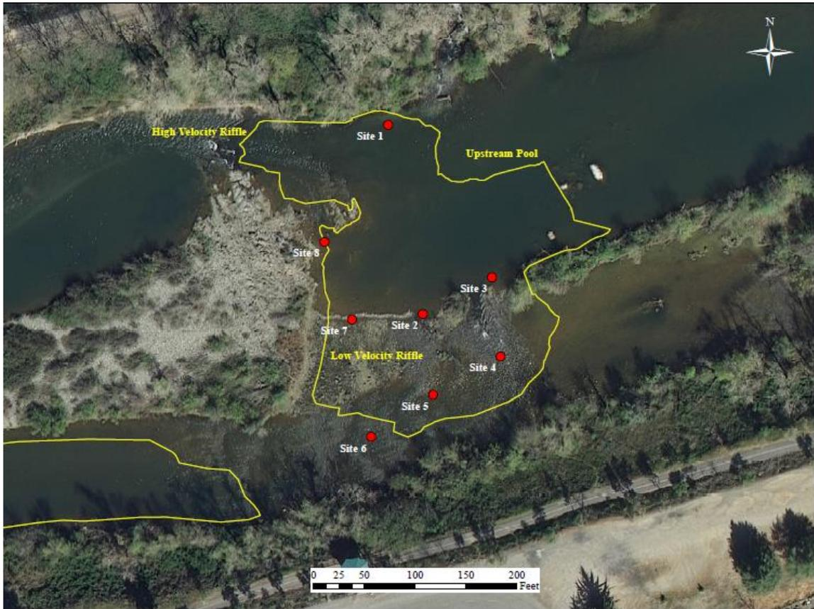
Figure 4: Cottonwood Hatchery Riffle mini-piezometer site locations. Mini piezometers were placed in areas that were “wadeable” and had some gravel over bedrock.
