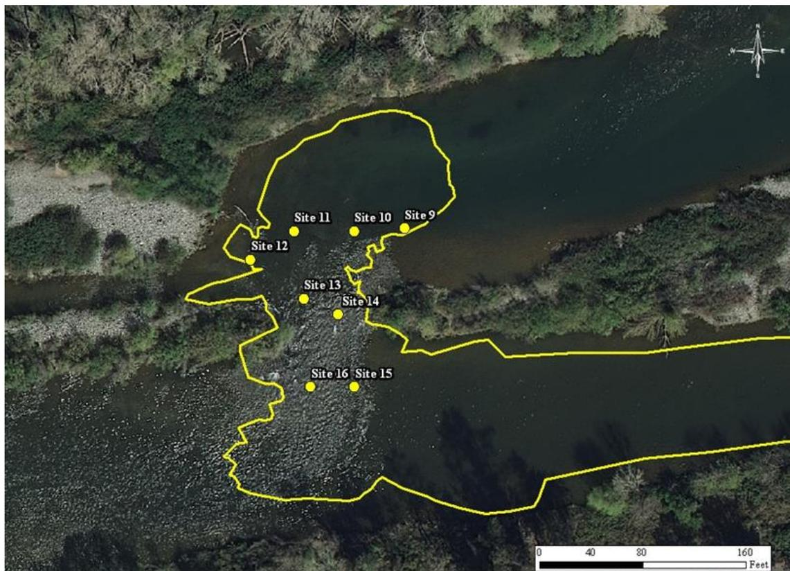
Figure 67: Site map of piezometers installed at Upper Auditorium Riffle.
