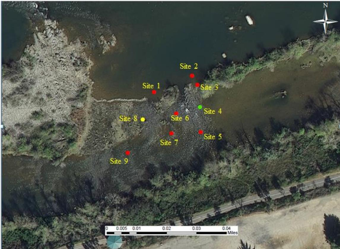
Figure 60: Permeability test locations at the Cottonwood Hatchery Riffle. Red dots are low K values, yellow dots are moderate K values, and green dots are high K values.
