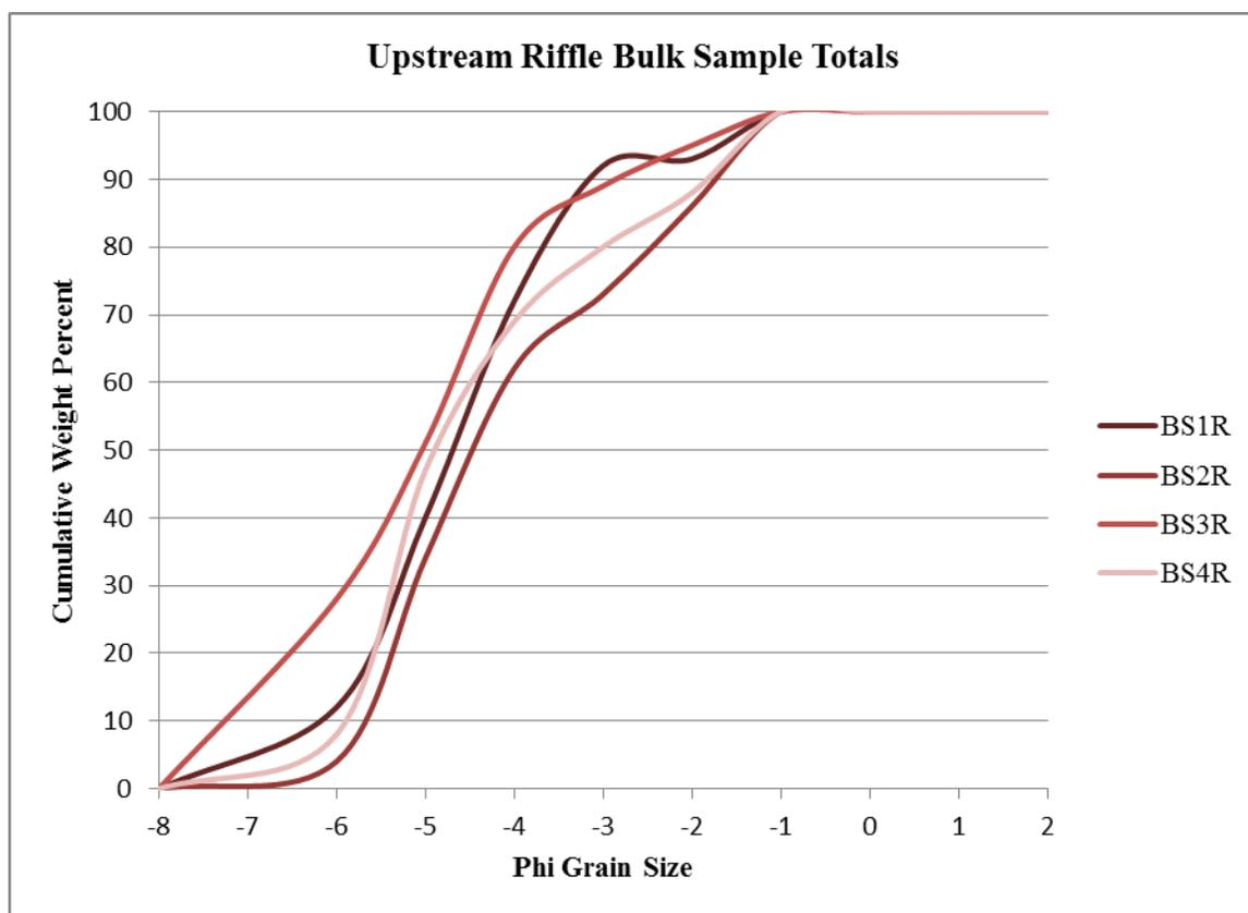
Figure 50: Bulk sample distribution graph of the Upstream Site. Four bulk samples were conducted the Summer of 2012.
