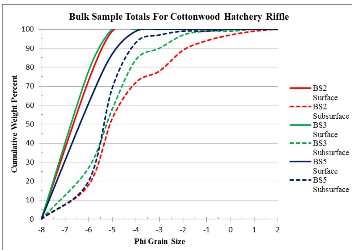
Figure 44: Bulk sample distribution chart for Cottonwood/Hatchery Riffle. Three bulk samples were conducted at the riffle complex and were separated into surface and subsurface sample sizes. The colored lines correspond to the colored dots on Figure 44.
