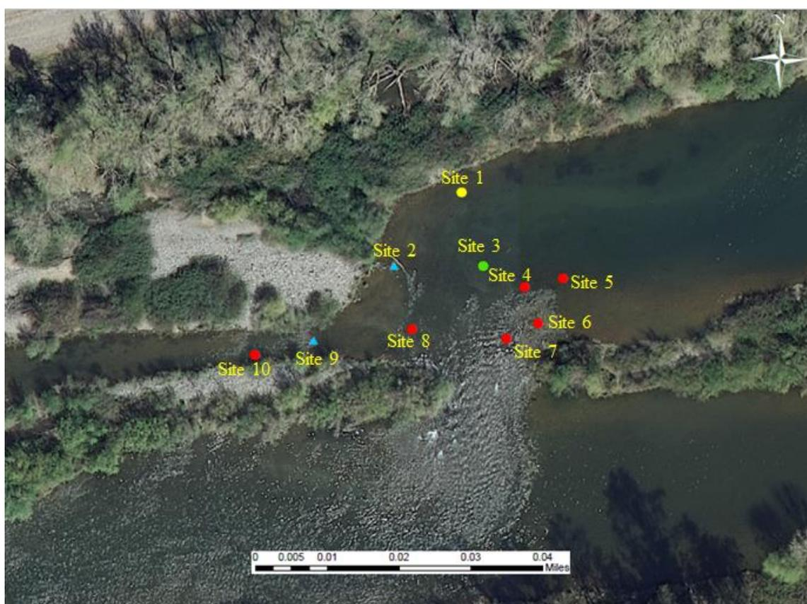
Figure 61: Locations of the standpipe tests at the Upper Auditorium Riffle. Red dots are low K values, yellow dots are moderate K values, green dots are high K values, and the blue triangles are wells that did not recover when pumped (very low permeability).
