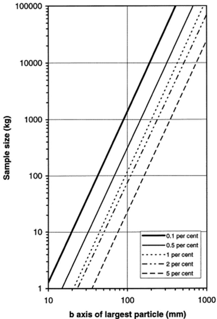
Figure 18: Bulk sample collection size chart. The intermediate (b-axis) size of the largest grain in the sample was measured and compared to this chart to yield a sample collection size and percentage of error. The larger the sample size, the smaller the percent error. From Church, et al (1987).
