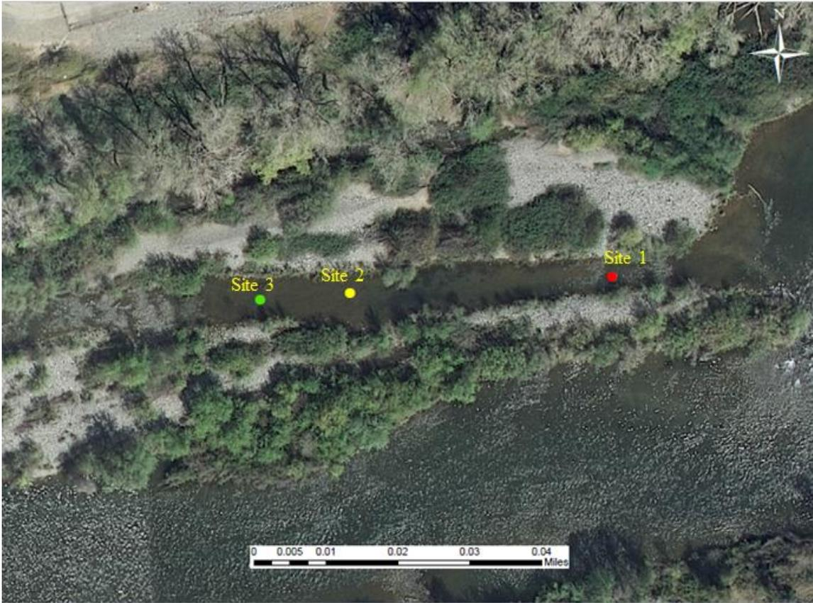
Figure 63: Locations of permeability tests at Moe's Ditch. Red dots are low K values, yellow dots are moderate K values, and green dots are high K values.
