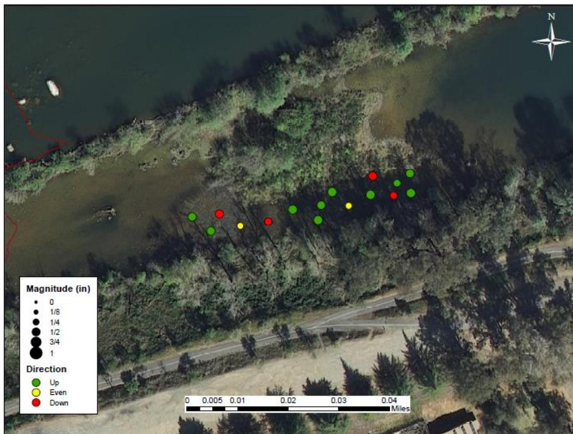
Figure 76: Upwelling/Downwelling map of the Upstream control site.
