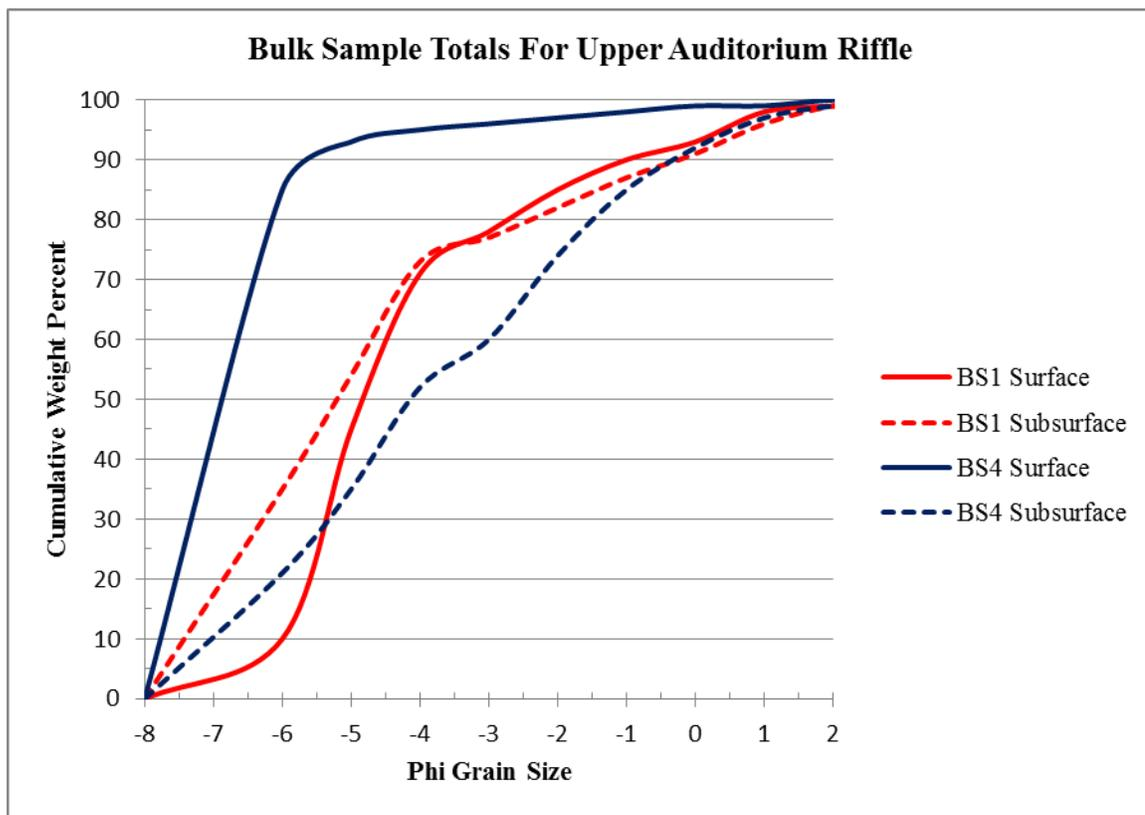
Figure 46: Bulk sample distribution chart for the Upper Auditorium Riffle Complex. Two bulk samples were collected at the riffle complex and are separated into surface and subsurface sample sizes.
