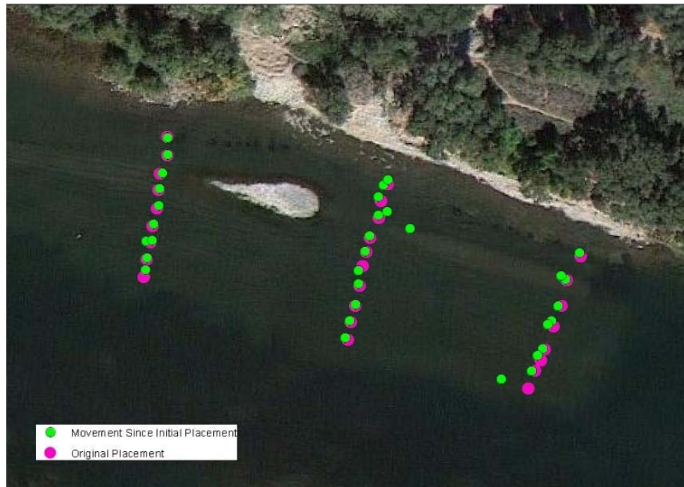
Figure 4.1: Post gravel addition map of Upper Sunrise 2010/2011 showing initial placement of tracer rocks (pink) and location of rocks located in May 2012 (green). Large (2.5 in. - 3 in.), medium (1.25 in. - 1.75 in.), and small (0.625 in. - 0.875 in.) tracer rocks were placed at each point on the map.
