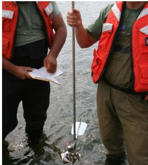
Figure 2.8: Field team determining surface water depth and velocity using a wading rod and Price AA current meter.
