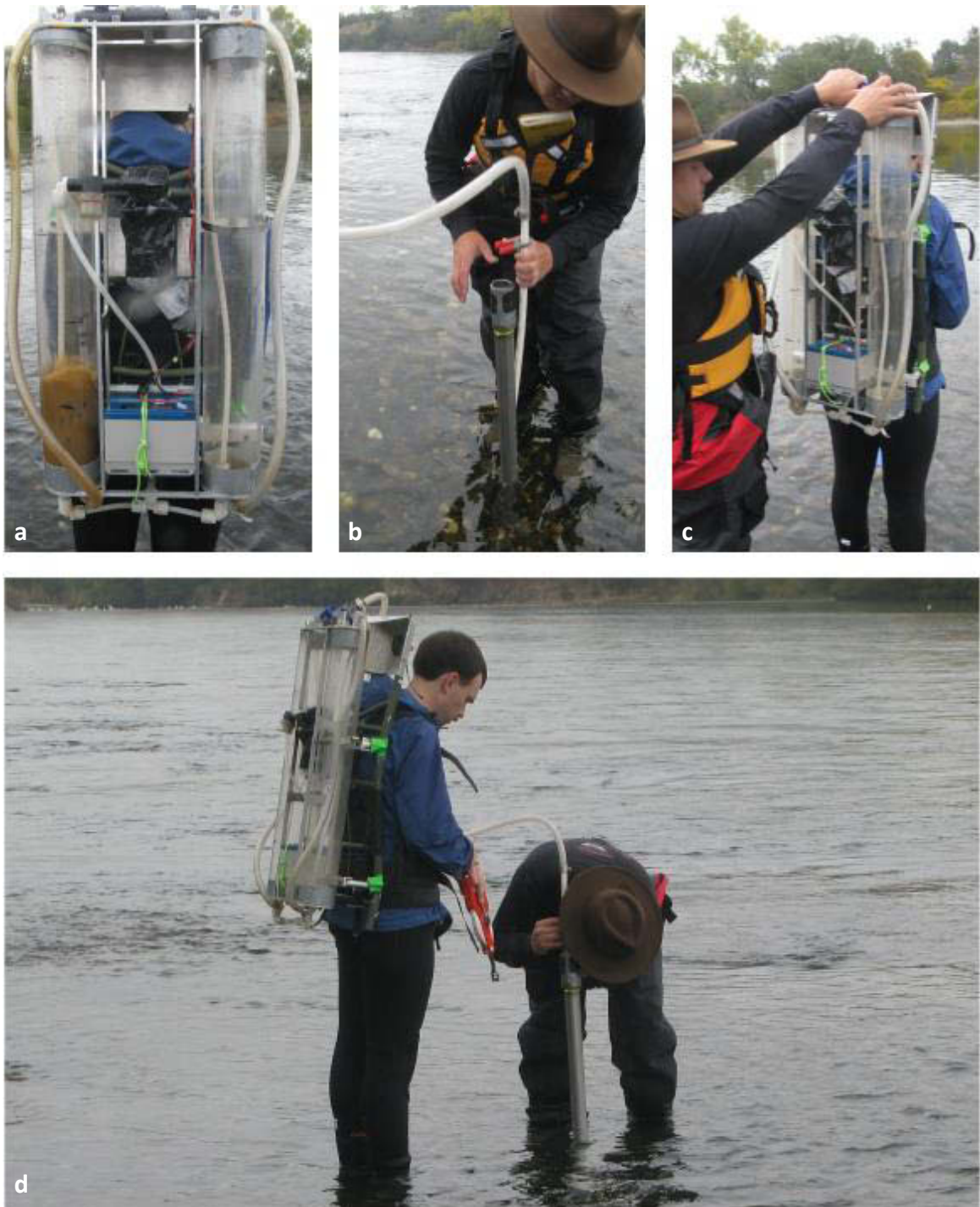
Figure 2.10: Drawdown testing uses a pumping apparatus (a) with two capture tanks. An extraction hose is inserted into the standpipe (b) one inch below the water level. The field team determined the water level in the pipe by listening for a “slurping” sound (d) that indicated the end of the hose had made contact with the water. When drawdown was achieved, the main capture tank was opened to collect the sample (c).
