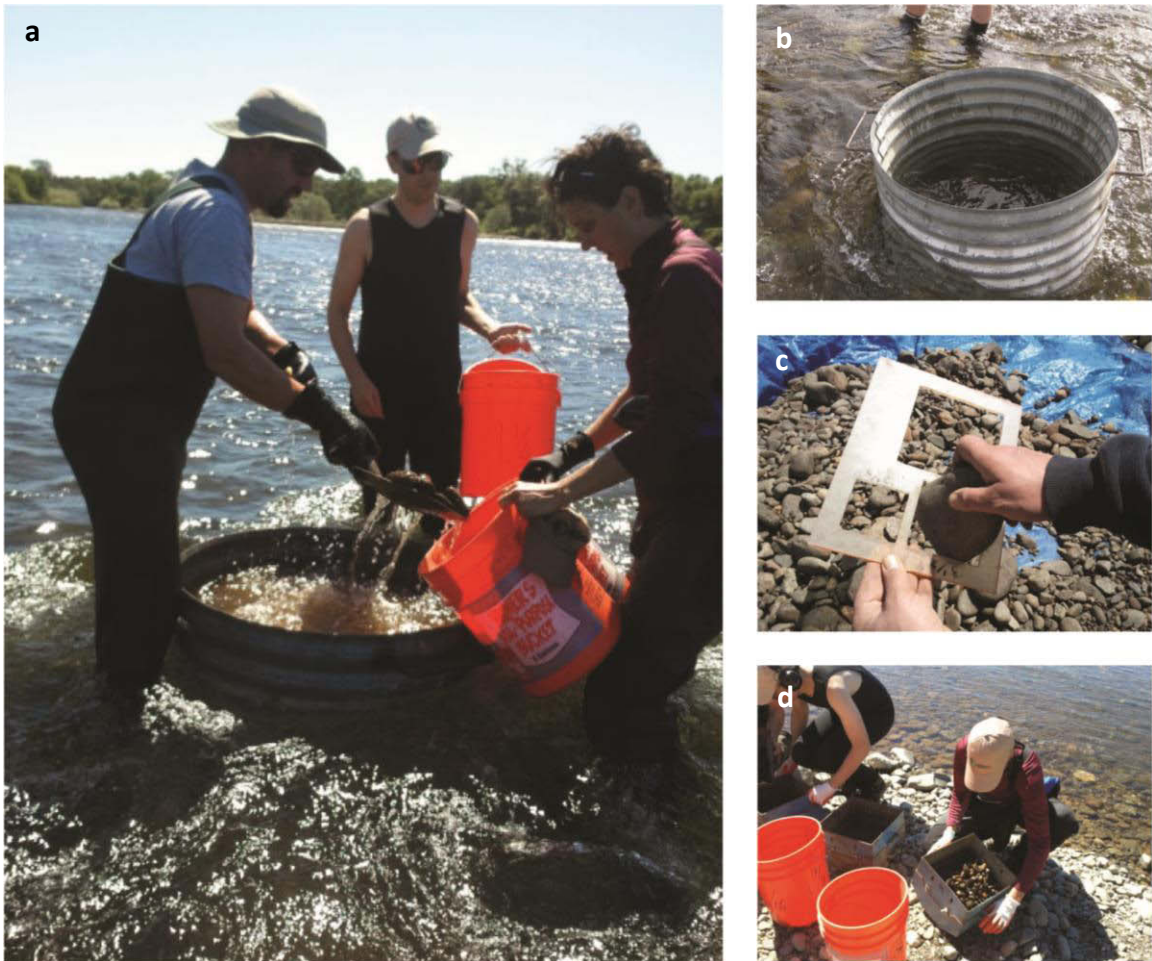
Figure 2.3: Bulk samples are (a) collected and transported to shore in 5 gallon buckets. (b) A metal baffle prevents fines from escaping during collection. (c) A pebble size template with square openings measures the intermediate axis diameter of grains; the largest opening through which the grain will not fit is considered the upper end of the grain size range. (d) Grains are sorted into size classes using rocker sieves.
