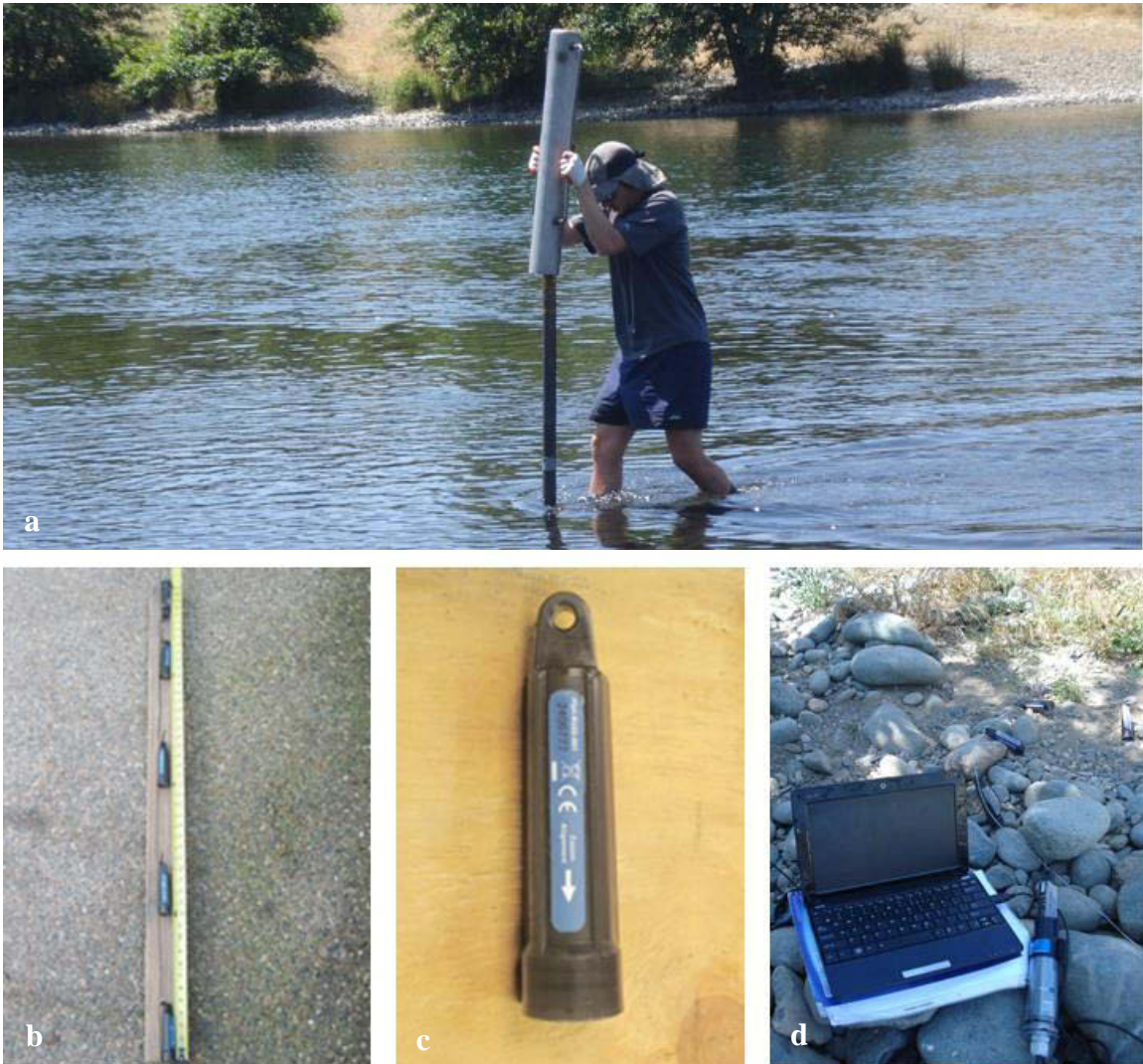
Figure 2.15: A string of (c) Hobo water Temp Pro v2 data loggers are affixed at (b) 0 foot (gravel river interface), 1 foot, 2 foot, 3 foot, 4 foot intervals and inserted into the streambed using a (a) sleeve assembly and post driver. Data is retrieved by (d) connecting each logger to a computer and uploading information.
