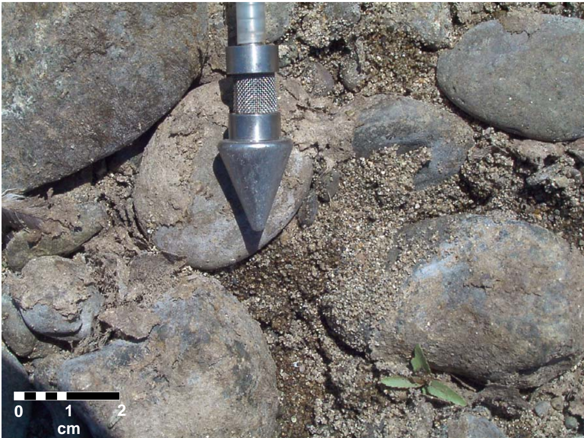
Figure 2: Photograph of mini-piezometer tip. Mini-piezometer tips were installed to a depth of 30 cm in the gravel using a steel over-drive rod. Piezometer tips were connected to the surface with 6 mm diameter plastic tubing. This allowed pore water samples to be collected from a discrete interval in the gravel. Vertical gradient (upwelling and downwelling) was also measured using these points and a bubble manometer board.
