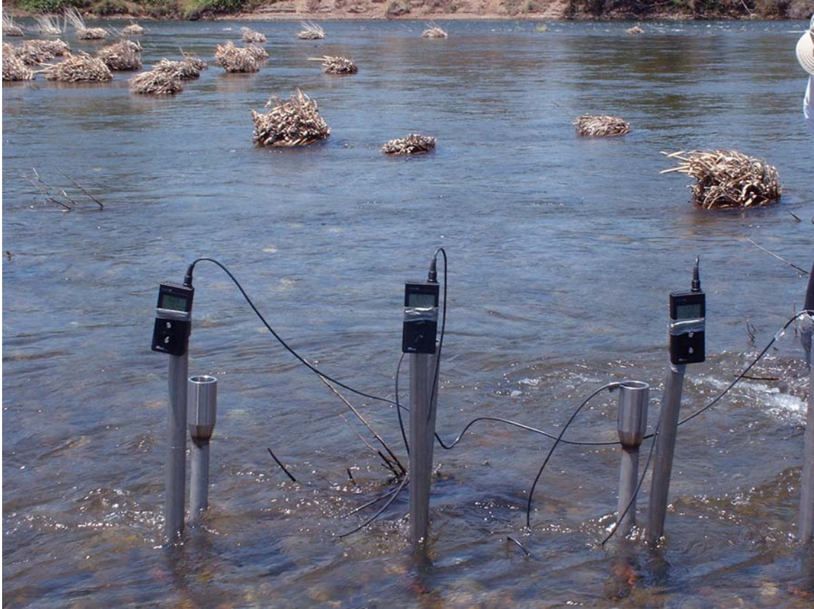
Figure 5: Piezometer array with dedicated electrical conductivity meters was used to track progress of the salt water plume during tracer tests. Piezometers were spaced 50 cm apart, and salt water was injected in the upstream piezometer (barely visible to the right of this photo).
