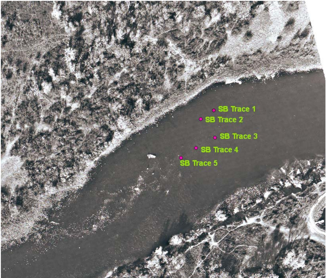
Figure 5.13: After gravel addition map of inter gravel velocity locations. SB Trace 1 and SB Trace 2 were conducted March 2010. SB Trace 3-5 were conducted April 2010.
