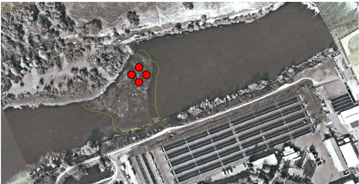
Figure 4.13: After gravel addition map of the salt water tracer tests. Tracer tests were conducted in March 2010.
