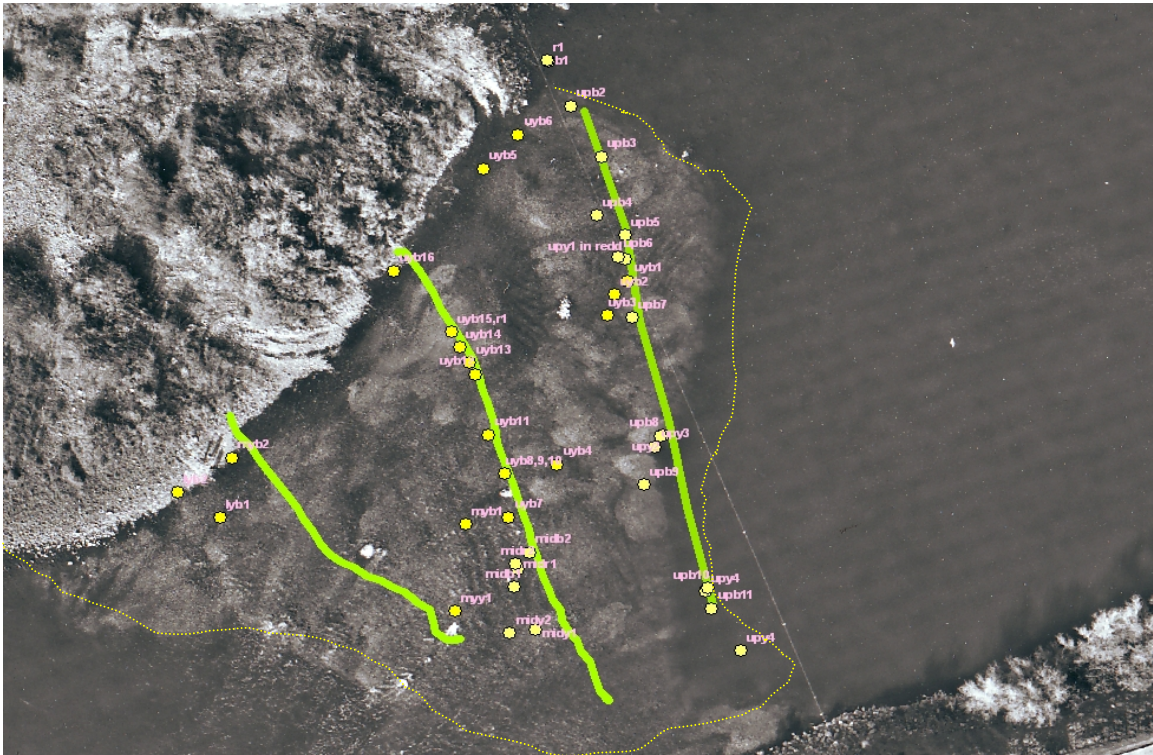
Figure 4.12: After gravel addition map showing the tracer rock transects from June 2009. Yellow points indicate rocks located.
