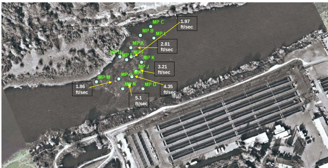
Figure 4.11: After gravel addition map showing average surface water velocity measurements in February 2009. Stream flow was 780 cfs. Mini piezometers without velocity values were either too shallow or less than 1 foot per second.
