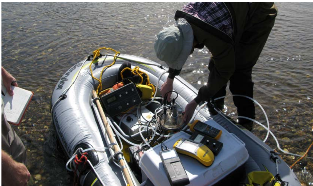
Figure 2.4: Picture of the field setup for the flow-through cell and water quality equipment.
