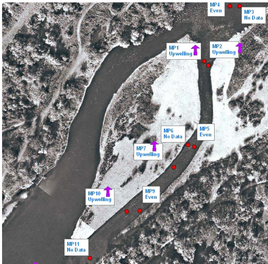
Figure 3.10: GIS map showing the bubble monometer measurements for the side channel from February 2009.
