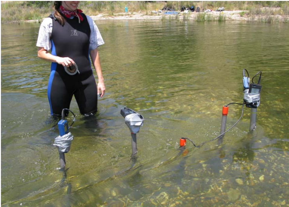
Figure 2.8: Picture showing the field set up of the permeability measurements.
