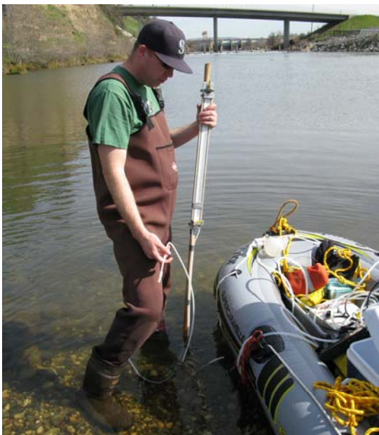
Figure 2.5: Picture of the manometer used for measuring the upwelling or downwelling for each mini piezometer.
