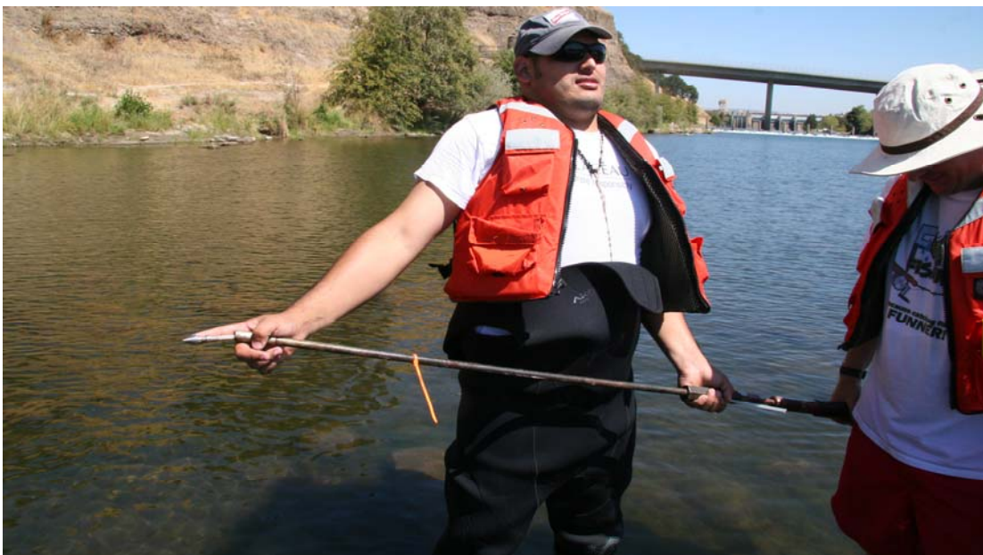
Figure 2.3: Picture of the piezometer tip and \frac{1}{4} inch tubing used for mini piezometers. The mini piezometer is inside of the drive rod device used for mini piezometer installation.
