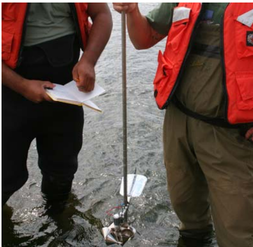
Figure 2.7: Picture showing the Price AA wading rod stream velocity measuring equipment.
