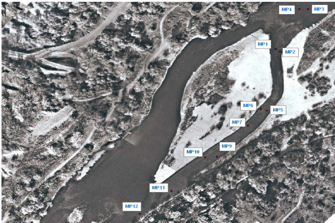
Figure 3.8: GIS Map showing the side channel mini piezometer locations.
