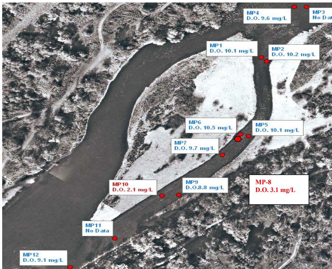
Figure 3.9: GIS map showing the D.O. values measured.
