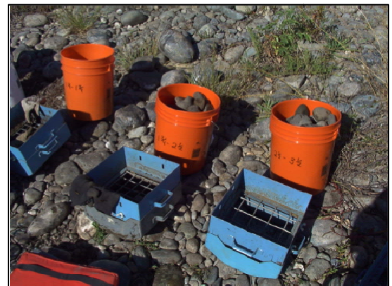
Figure 2.1: i). Metal baffle prevents fines from escaping downstream. ii) Five gallon buckets containing different size classes after grains were sieved.
