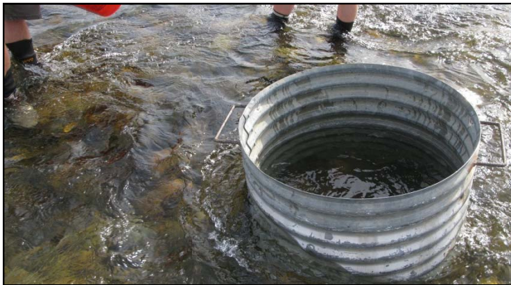
Figure 2.1: i). Metal baffle prevents fines from escaping downstream. ii) Five gallon buckets containing different size classes after grains were sieved.
