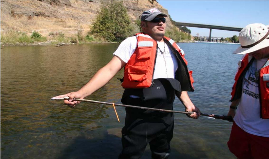
Figure 3: Picture of the piezometer tip and  $\frac{1}{4}$  inch tubing used for mini piezometers. The mini piezometer is inside of the drive rod device used for mini piezometer installation.
