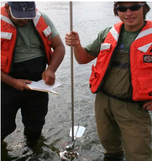
Figure 6: Picture showing the Price AA wading rod stream velocity measuring equipment.
