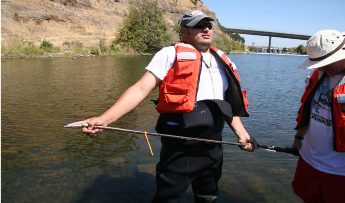
Figure 3: Picture of the piezometer tip and ¼ inch tubing used for mini piezometers. The mini piezometer is inside of the drive rod device used for mini piezometer installation.
