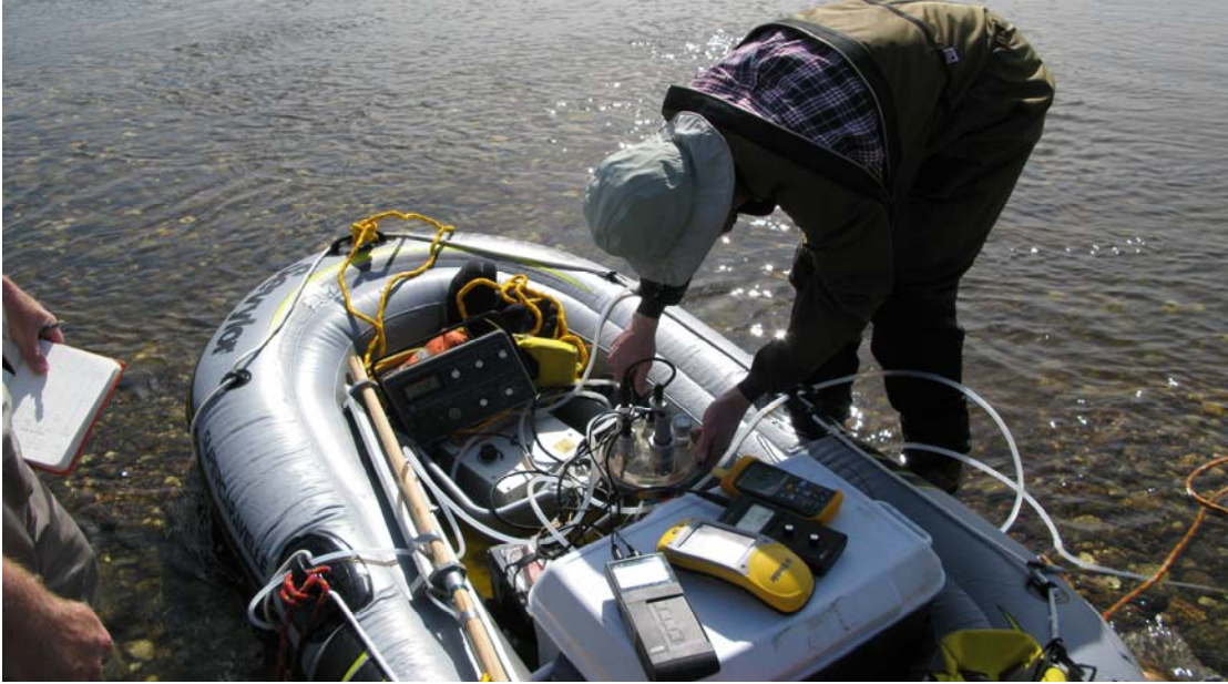
Figure 4: Picture of the field equipment with the pump, flow-through cell, and water quality meters.
