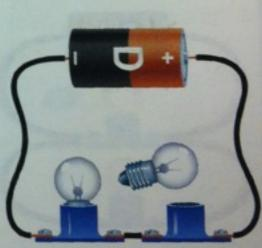
If one part of a series circuit is removed or broken, electric current cannot flow in the circuit.
