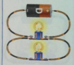
In a parallel circuit, each part, or branch, has its own path for electric current. The electric current passes through all of them at the same time.
