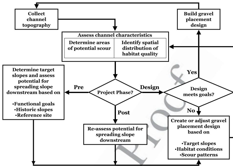
**Figure 2.** Conceptual model describing slope creation methodology used in this study for Chinook salmon spawning habitat rehabilitation. Before using this, preliminary planning including goal setting should be performed, such as described by *Wheaton et al.* [2004a].
