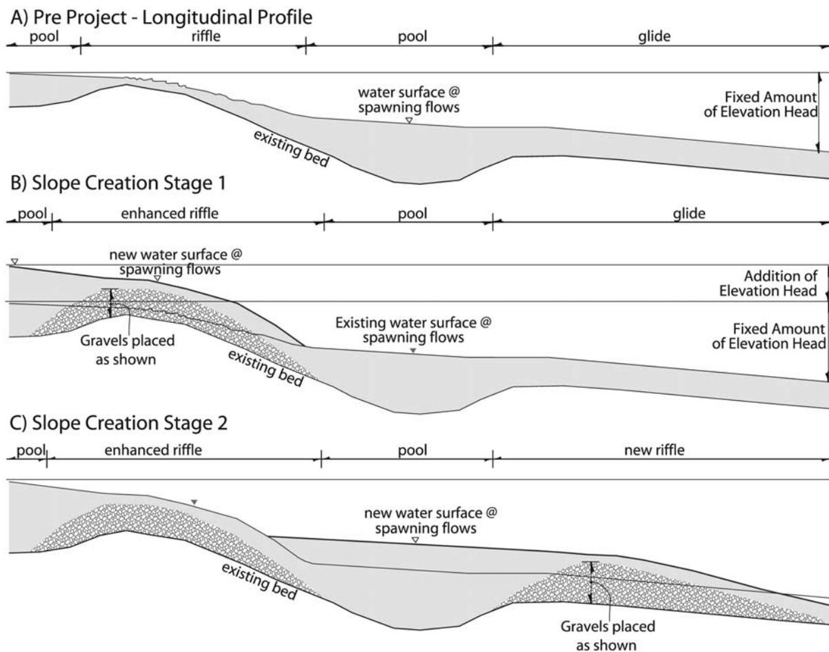
**Figure 1.** Longitudinal profile of a stream illustrating a two-stage addition of gravel for “slope creation,” such as performed in this study. After the first stage, riffle-to-riffle slope is steeper than desired, but that is resolved in the second stage.
