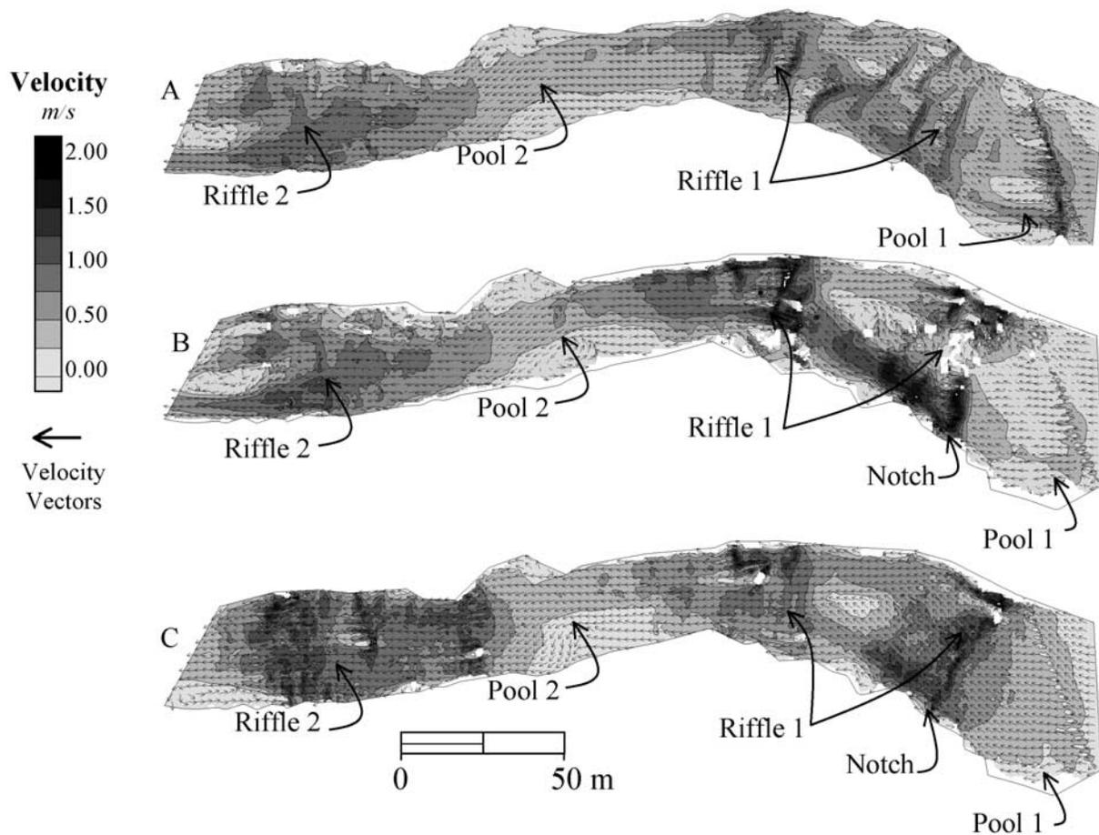
**Figure 8.** Two-dimensional model velocity predictions at 11.33 m<sup>3</sup>/s for the (a) premanipulation, (b) midmanipulation, and (c) postmanipulation stages. Arrows indicate velocity direction, while darker shading equals higher velocity.
