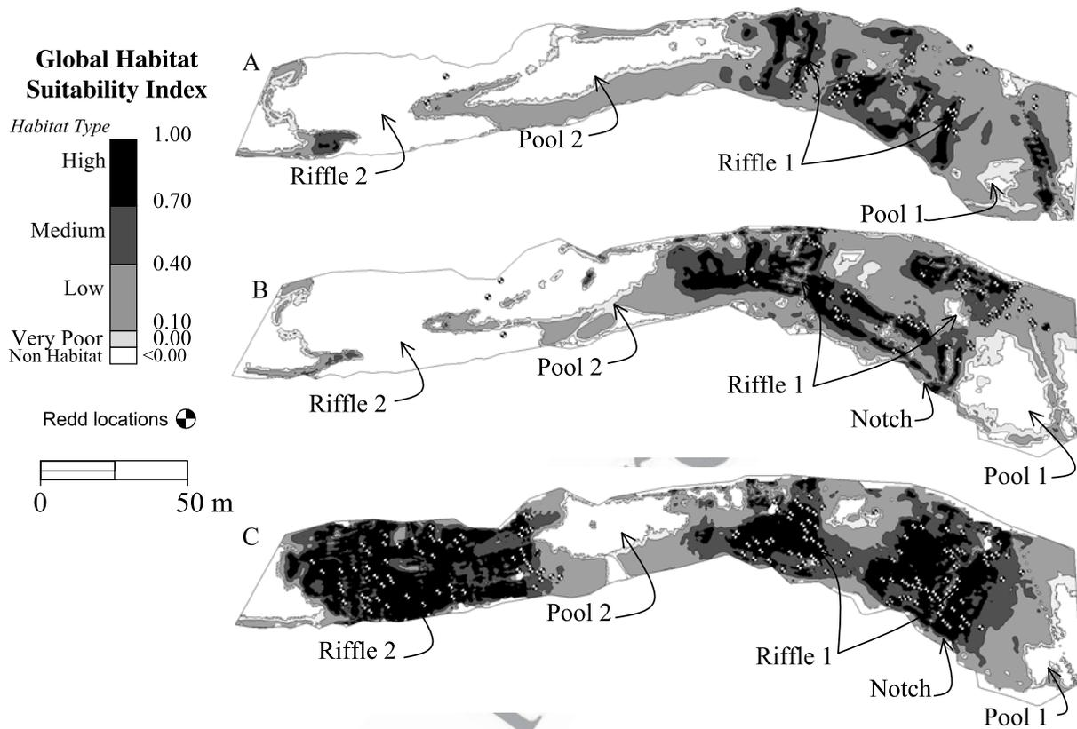
**Figure 9.** Two-dimensional model habitat quality predictions at 11.33 m<sup>3</sup>/s showing the global habitat suitability index (GHSI) at the (a) premanipulation, (b) midmanipulation, and (c) postmanipulation stages. Validation is provided by comparison against actual redd locations for each stage, shown as targeted disks.
