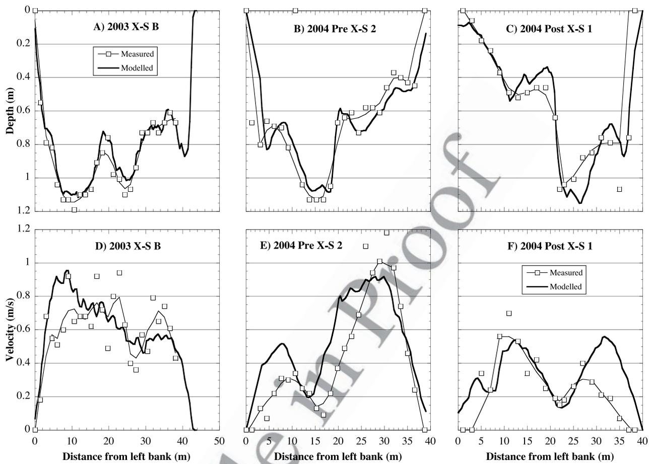
**Figure 6.** Comparisons of observed versus predicted depths and velocities at a representative cross section for the (a, d) preproject, (b, e) midproject, and (c, f) postproject stages. Field observations were fit with a curve using the locally weighted least squares error method to reduce measurement noise.
