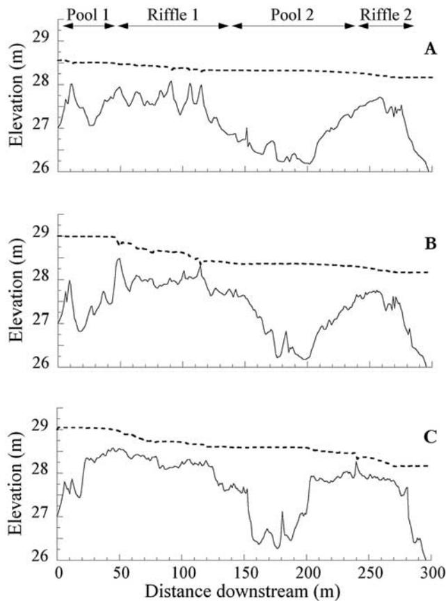
**Figure 7.** Longitudinal profiles showing change in thalweg elevation (solid line) and water surface elevation (dashed line) for the (a) premanipulation, (b) midmanipulation, and (c) postmanipulation stages of the study.
