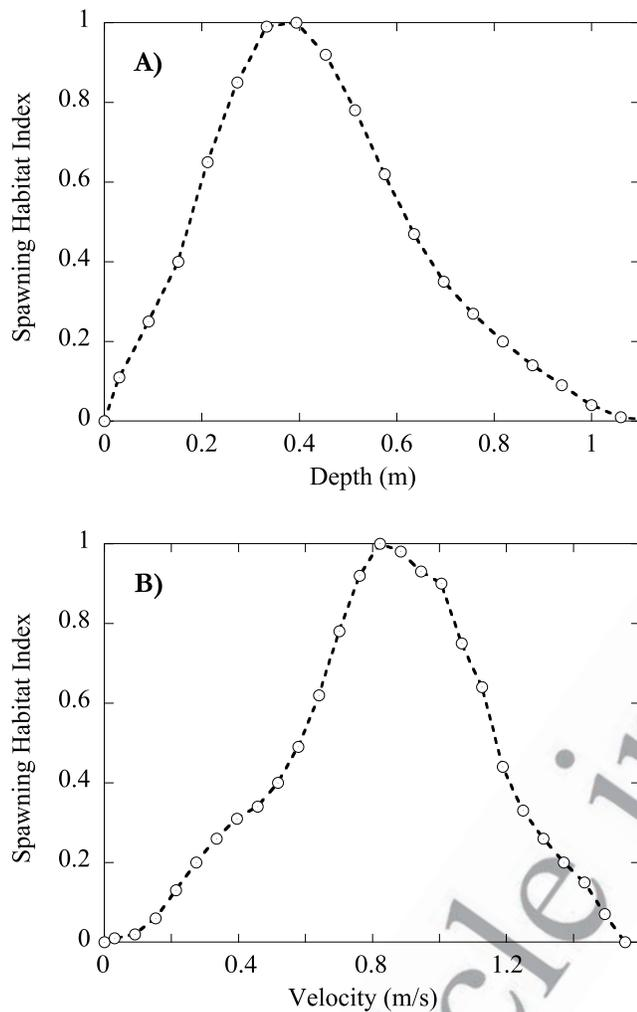
**Figure 5.** Habitat suitability curves developed for the Mokelumne River by *CDFG* [1991]. Curves predict habitat quality based on flow depth, velocity, and substrate type.
