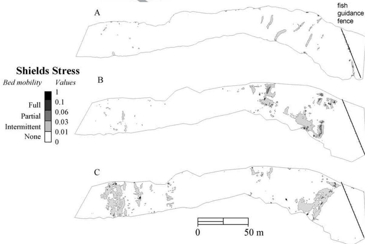
**Figure 11.** Two-dimensional model predictions of Shield stress at 11.33 m<sup>3</sup>/s for the (a) premanipulation, (b) midmanipulation, and (c) postmanipulation stages of the study.
