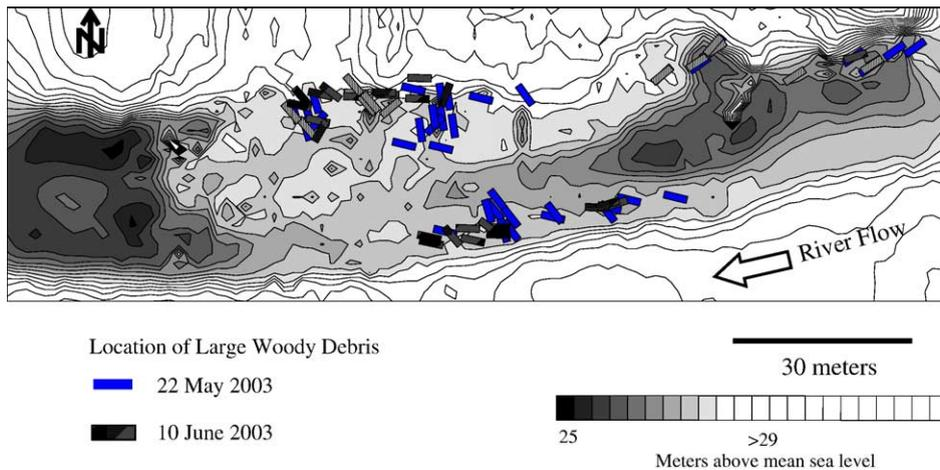
Fig. 11. Location of large woody debris before and after a 19-day flow increase at site A, lower Mokelumne River, California.
