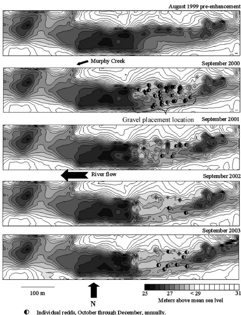
Fig. 4. Contour maps depicting streambed elevation before and after gravel placement at site A, lower Mokelumne River California.
