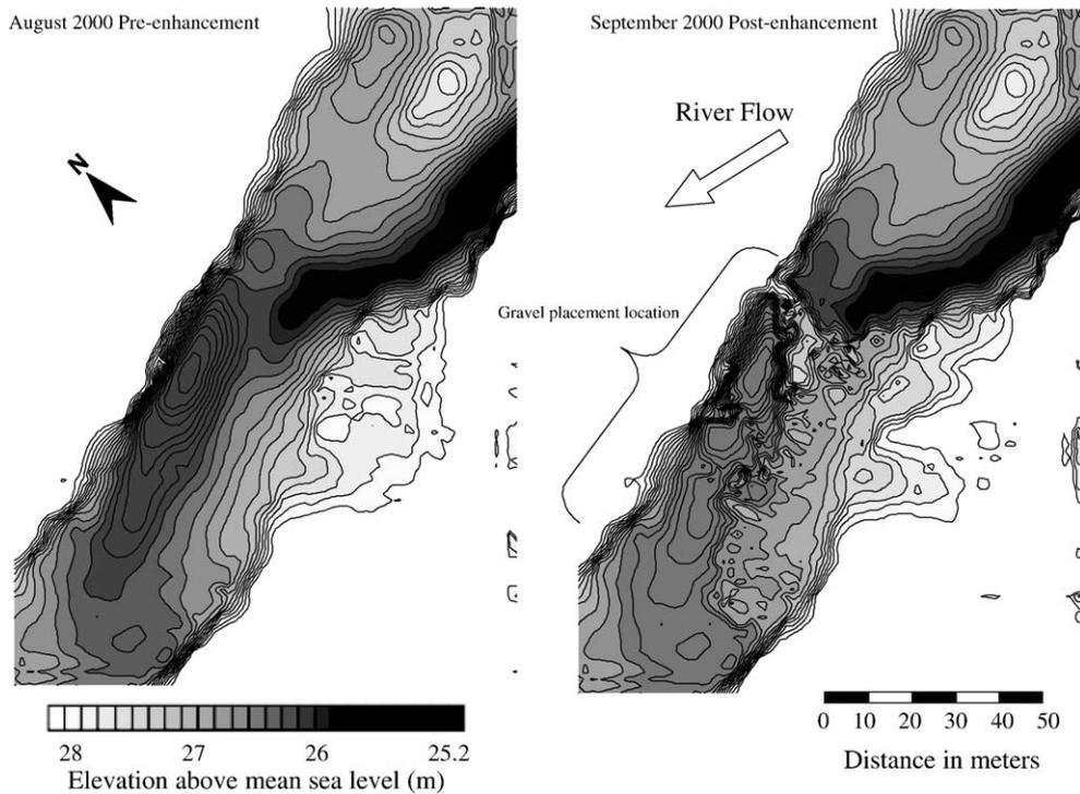
Fig. 5. Contour maps depicting streambed elevation before and after gravel placement at site B, lower Mokelumne River, California.
