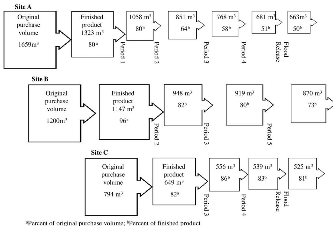
Fig. 13. Volumetric gravel budget for three Chinook salmon spawning enhancement projects in the lower Mokelumne River, California. Time periods are provided in Fig. 3 and Table 2.
