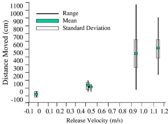
Fig. 9. Distance downstream tracer rocks were recorded after 12 months, compared to velocities recorded at initial release, site A, lower Mokelumne River, California.
