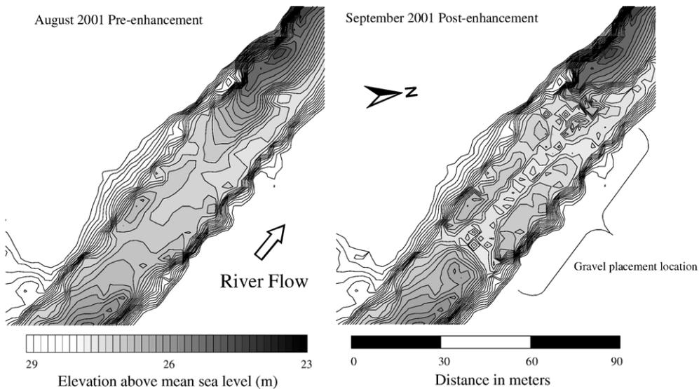
Fig. 6. Contour maps depicting streambed elevation before and after gravel placement at site C, lower Mokelumne River, California.
