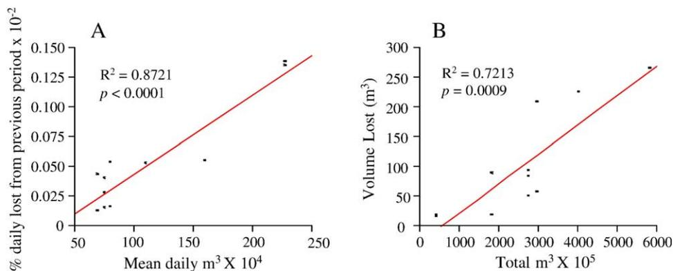
Fig. 8. Comparison of bed cut, as indicated by volume and percent, to river flow at 3 gravel enhancement sites over 5 various time periods, lower Mokelumne River, California. A: Percent daily gravel volume lost from previous period by mean daily m<sup>3</sup> of water released from Camanche Dam; B: Total gravel volume lost (m<sup>3</sup>) by total m<sup>3</sup> of water released from Camanche Dam.
