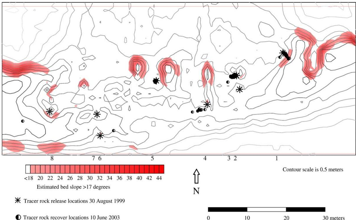
Fig. 10. Tracer rock release and recovery locations in relation to estimated bed areas where slope meets or exceeds the angle of repose. Base map is of as-built contours of site A, 30 August 1999. Numbers indicate tracer rock release pile designation.
