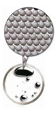
◀ Figure 5.8 An atomic element The basic units that compose mercury, an atomic element and a metal, are single mercury atoms.
