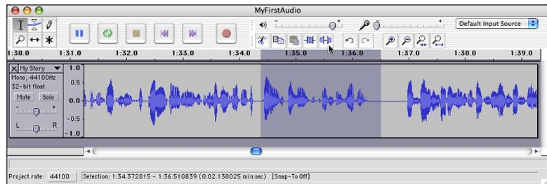
Figure 4.11. The audio region after converting region to silence.
