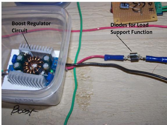
Figure 41: Boost Regulator installed on prototype and interfaced with diodes
