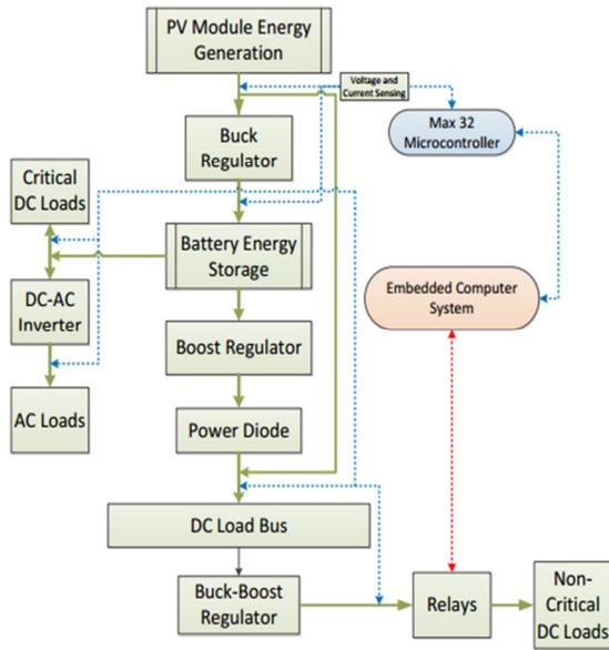
Figure 36: Hardware Block Diagram Model
