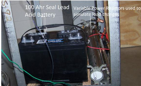
Figure 42: Sealed Lead Acid Battery and Variable Power Resistors
