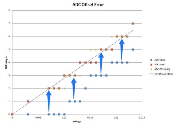
Figure 63: ADC Offset Error
