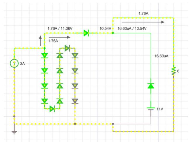
Figure 32: Load Support Simulation with Diode Reverse Biased
