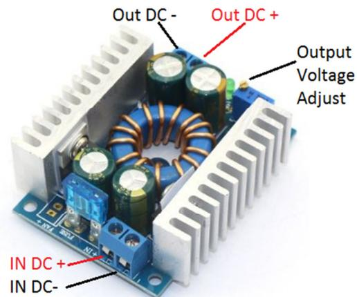
Figure 40: DROK Boost circuit used in laboratory prototype
