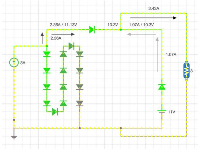
Figure 34: Load Support Simulation with Battery Supply
