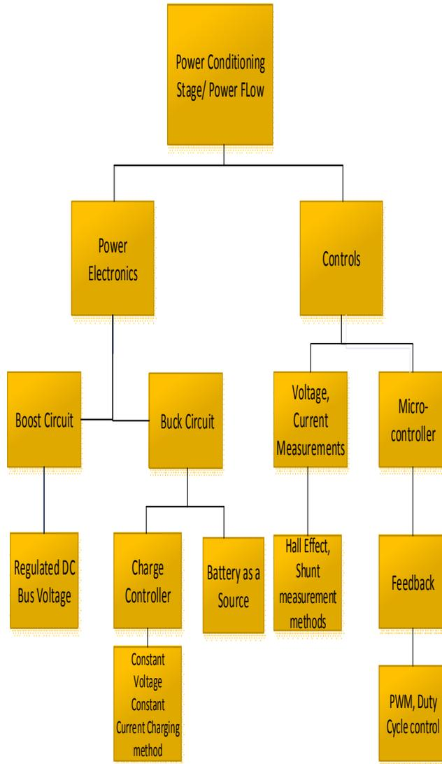
Figure 12: WBS Flow Diagram of the Power Conditioning and Flow Stage
