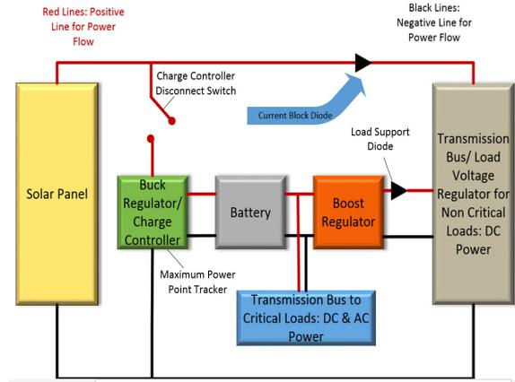
Figure 62: Block Diagram of Microgrid Power Flow
