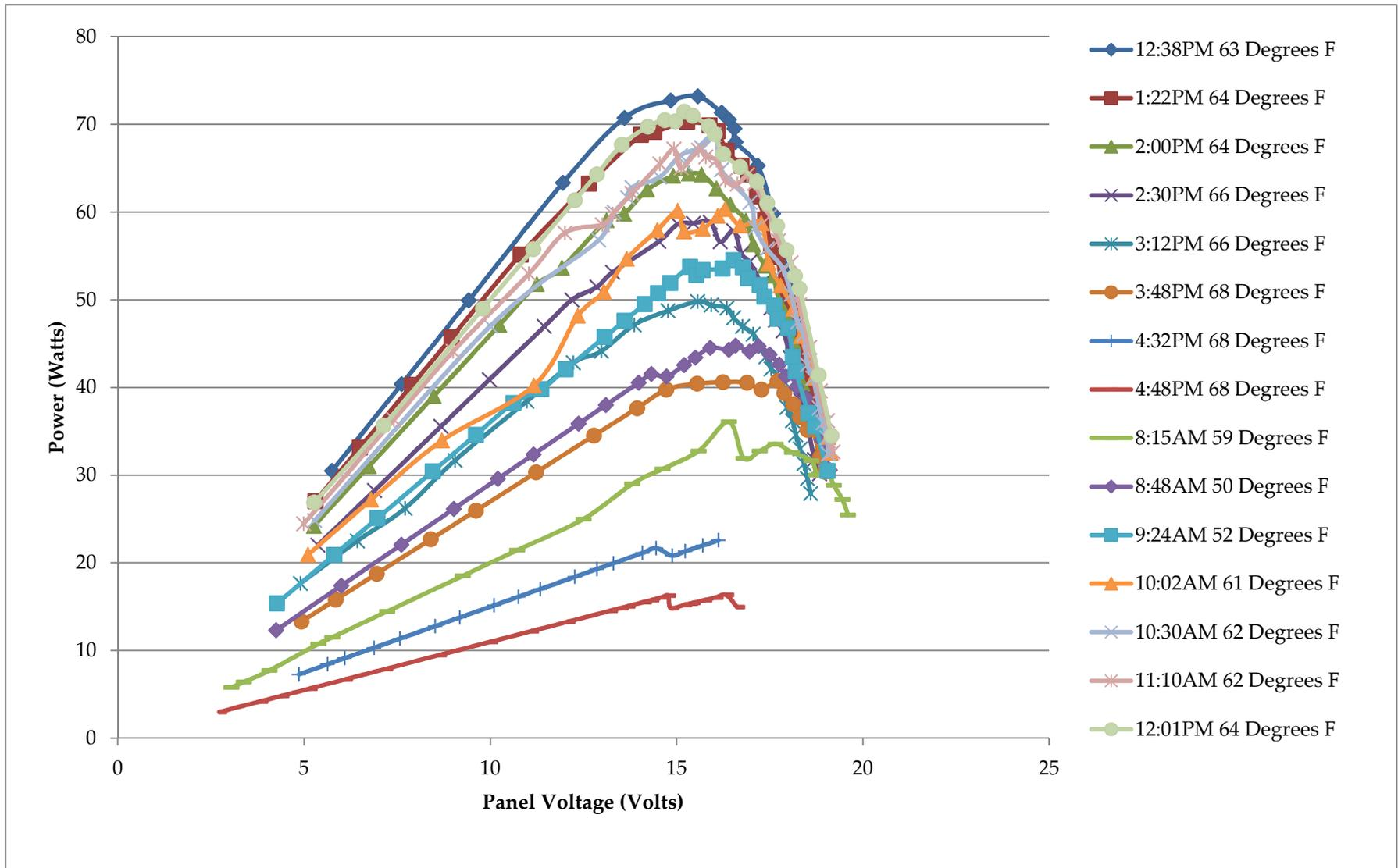
Figure 59: Ramsond 100W Mono-Crystalline Power Output versus Panel Voltage
