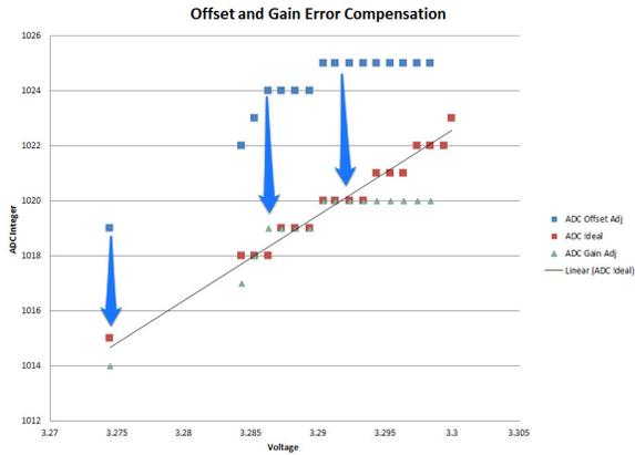
Figure 64: Offset and Gain Error
