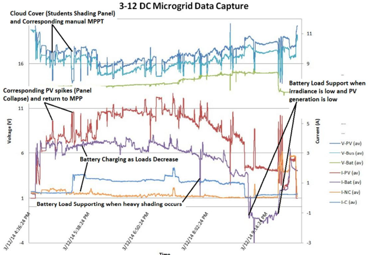
Figure 61: Data collected from diurnal testing of 100 watt rapid prototype on March 12th 2014
