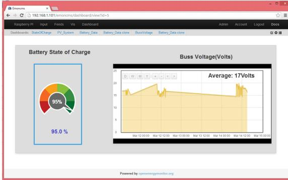
Figure 68: Bus Voltage and Battery State of Charge
