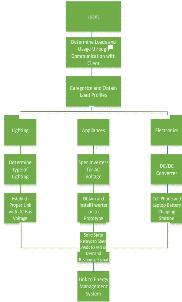
Figure 14: WBS of the Loads Stage
