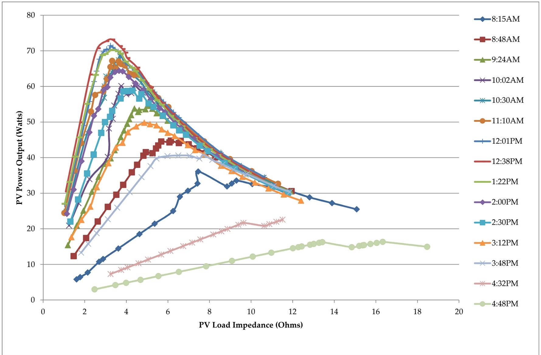
Figure 60: Ramsond 100W Mono-Crystalline Power Output versus Load Impedance
