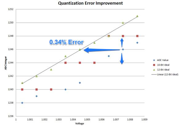
Figure 65: Quantization Error
