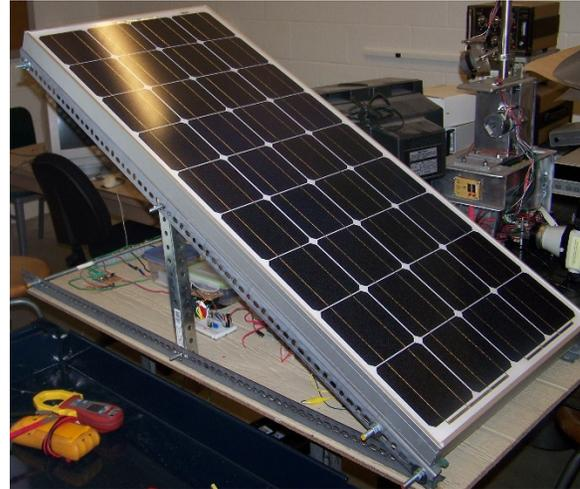
Figure 37: 100 Watt Ramsond solar panel installed on laboratory prototype
