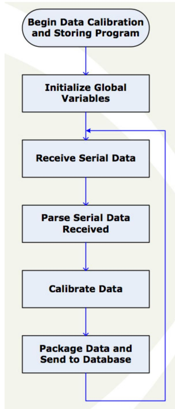
Figure 45: Python Code Calibration and Storage Flow Chart
