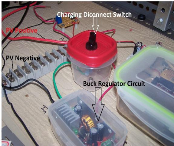
Figure 39: Buck Regulator interfaced with Disconnect Switch (in on position)
