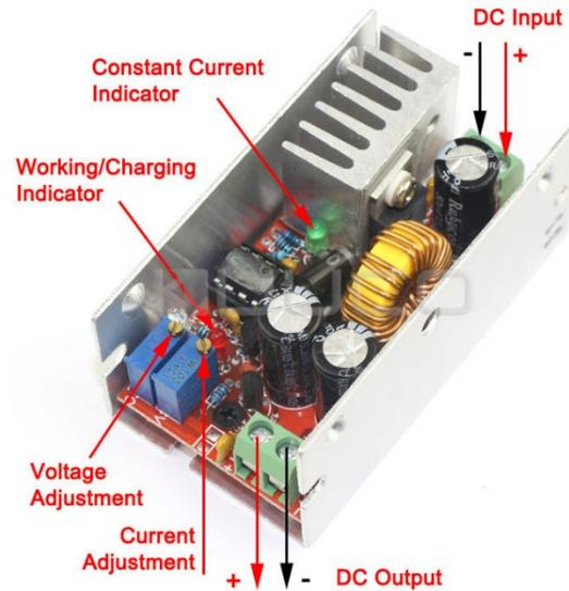
Figure 38: DROK Buck circuit used in laboratory prototype
