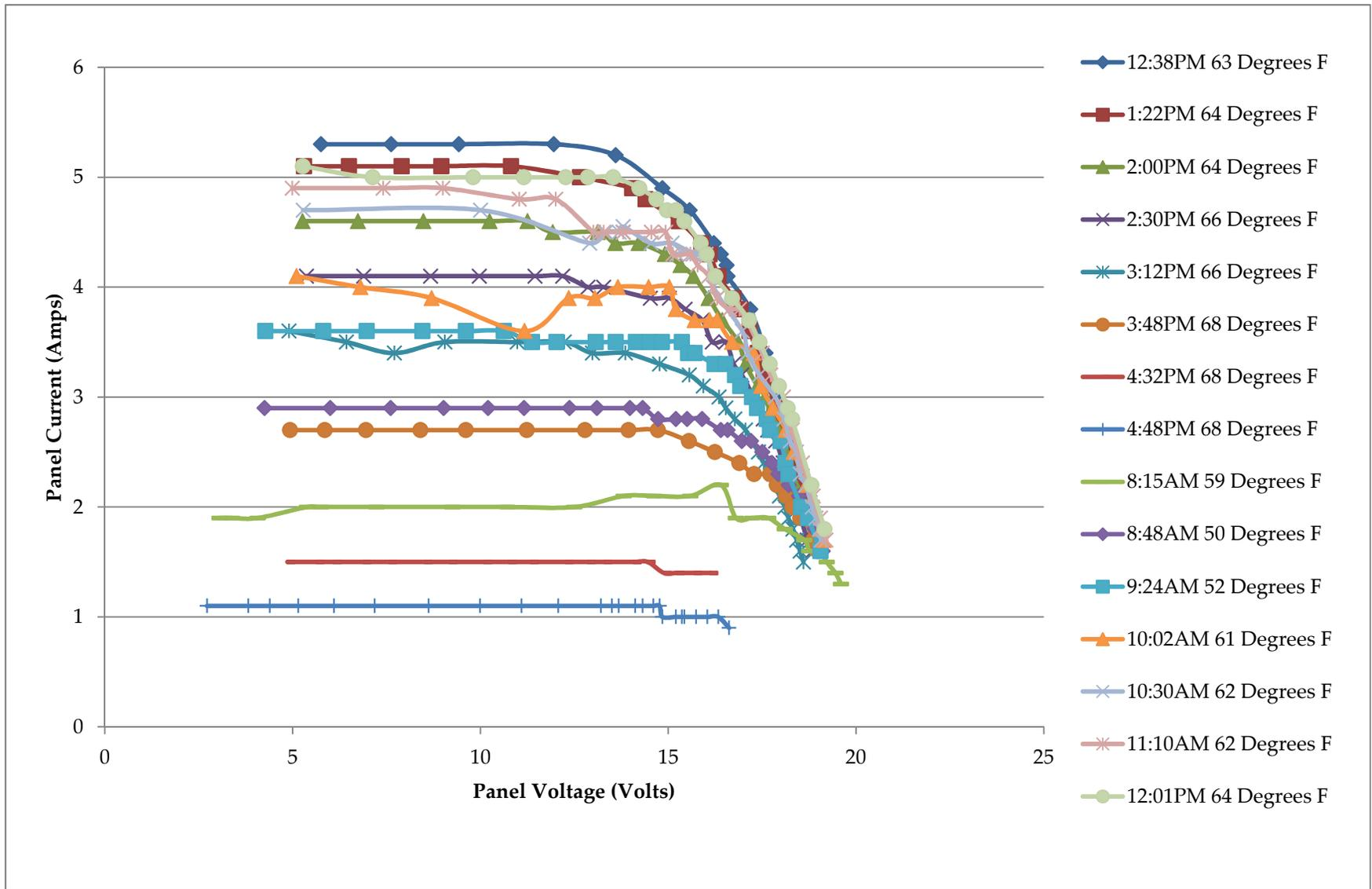
Figure 58: Ramsond 100W Mono-Crystalline Measured I-V Characteristics
