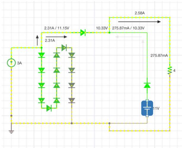
Figure 33: Load Support Simulation with PV @ Max. Power
