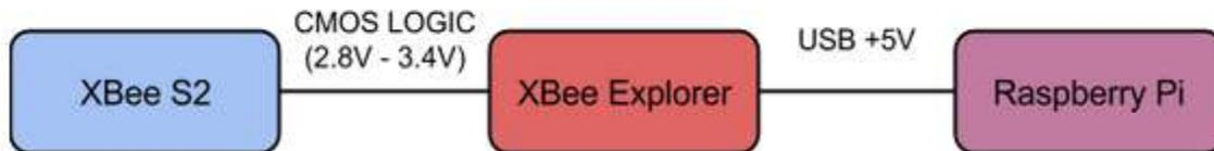
Figure 39: Base Station Block Diagram
