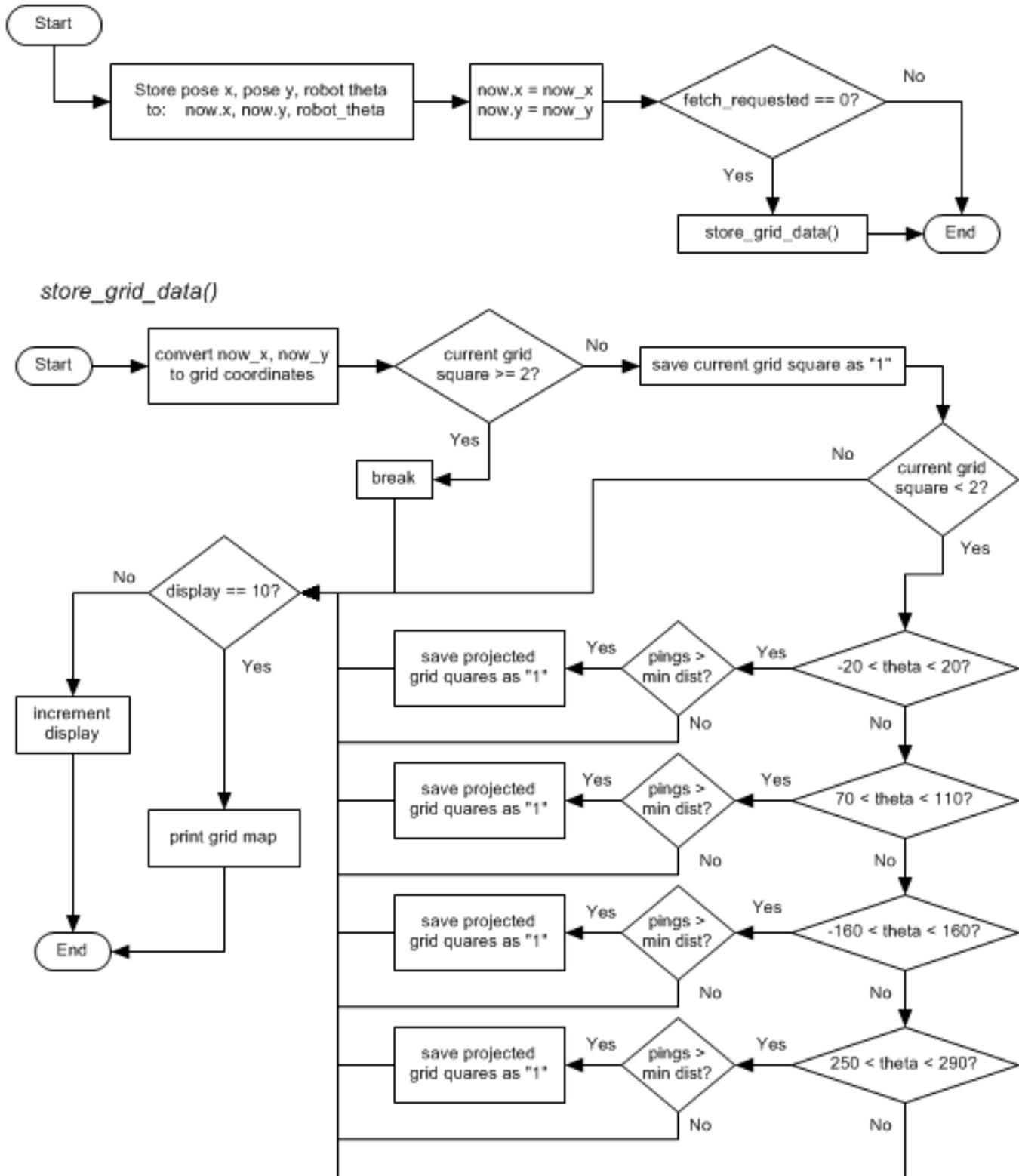
Fig. 17: Robot Position & Create Map Flowchart
