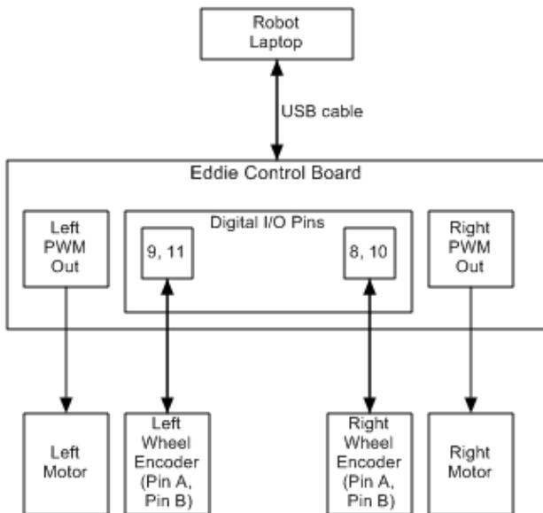
Fig. 10: Robot Hardware Flowchart
