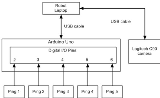
Fig. 9: Microcontroller w/Pings and Camera to Laptop
