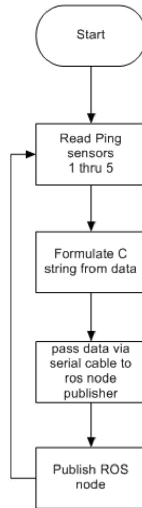
Fig. 15: Ping Sensor Flowchart
