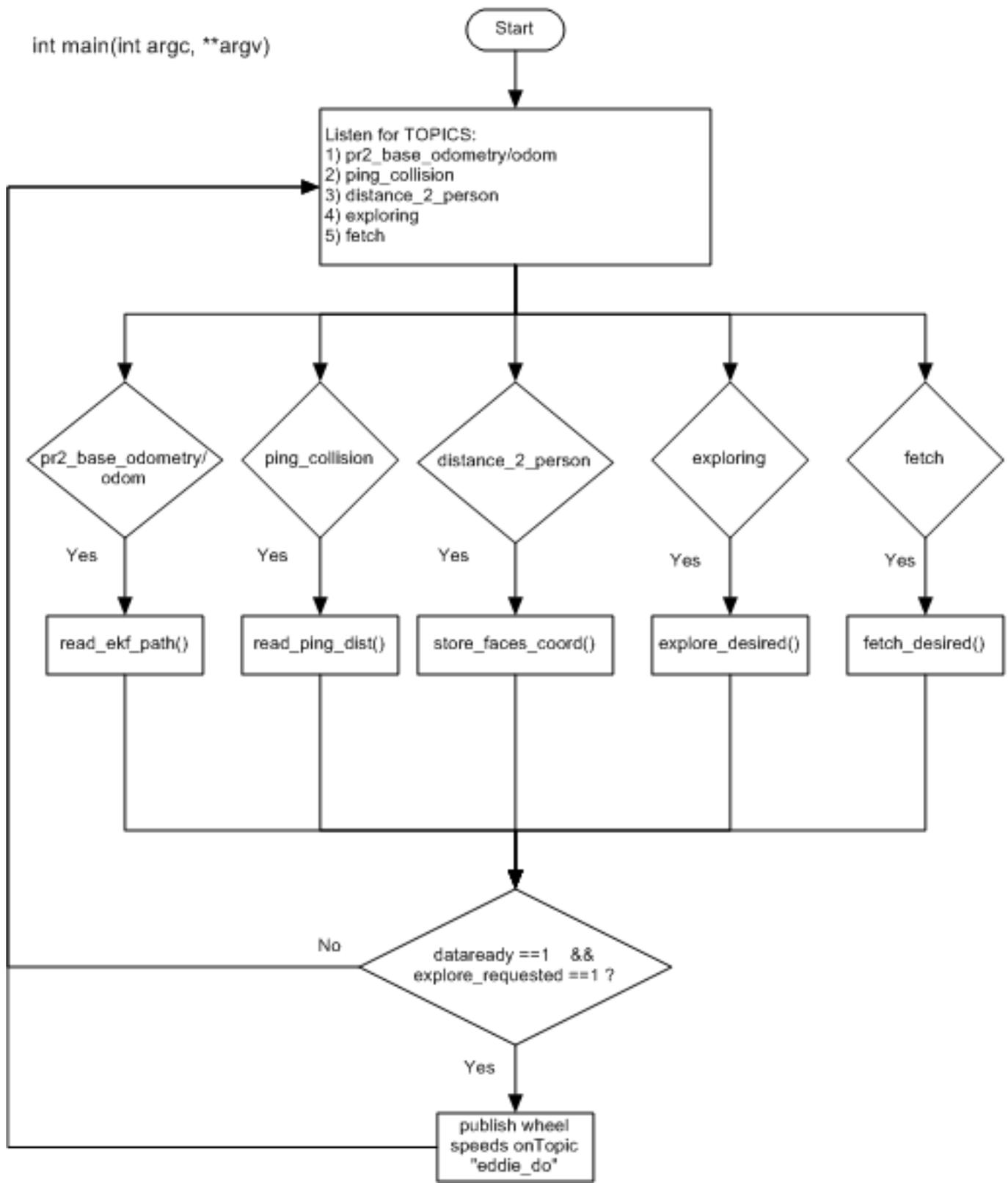
Fig. 16: Path Planning System Flowchart
