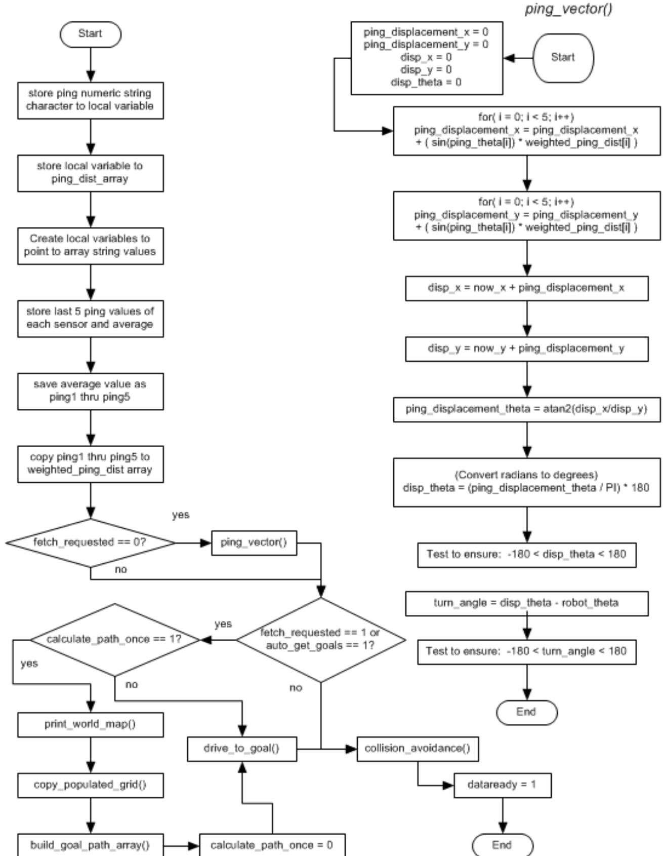
Fig. 18: Read Ping Distance Flowchart
