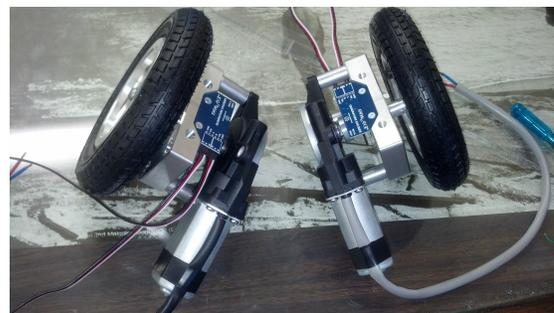
Fig. 5: Motors with 144 tick encoders
