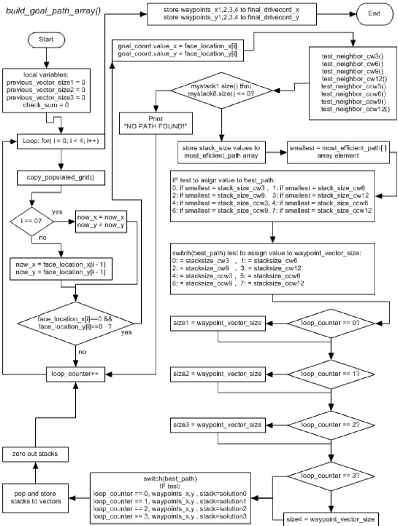
Fig. 19: Path Planning Algorithm Flowchart
