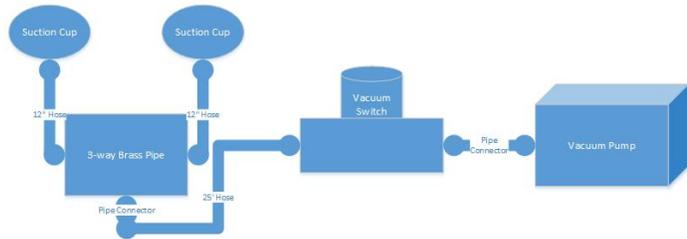
Fig. 23: Final High Level Overview of Vacuum System [20].
