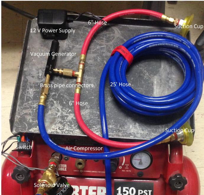
Fig. 20: Vacuum System Components [18].
