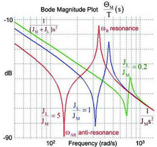
Fig. 19: Impact of Different Motor/Load Inertia Ratios [17].
