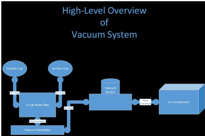
Fig. 22: High Level Overview of Vacuum System [20].
