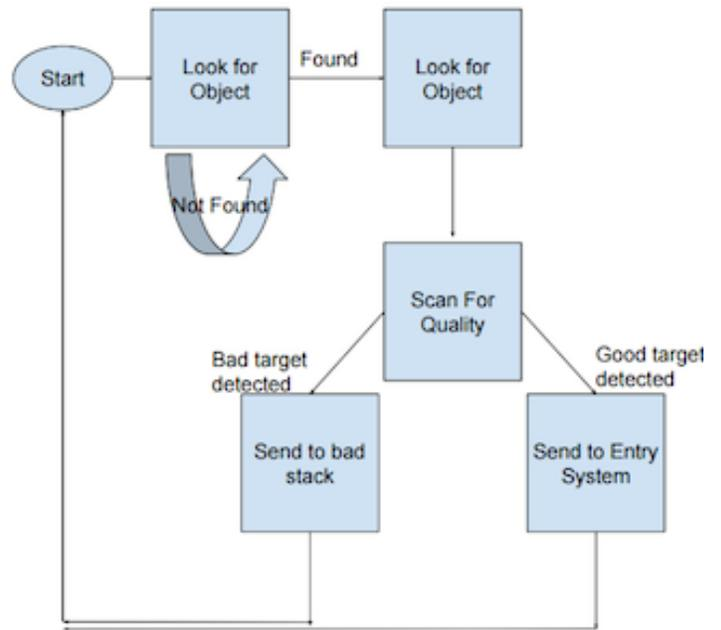
Fig. 24: High Level view of the Vision System [21].
