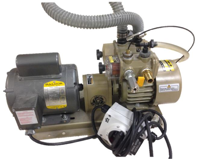
Fig. 21: Vacuum System Pump [19].
