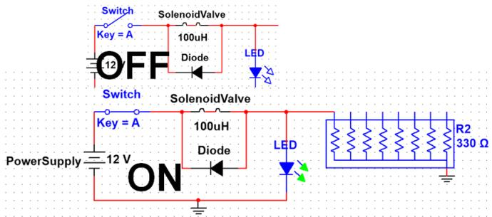
Fig. 26: Solenoid Valve Circuit [23].
