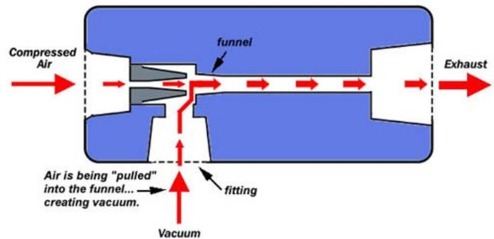
Fig. 3: Working Process of a Vacuum gripper [3].
