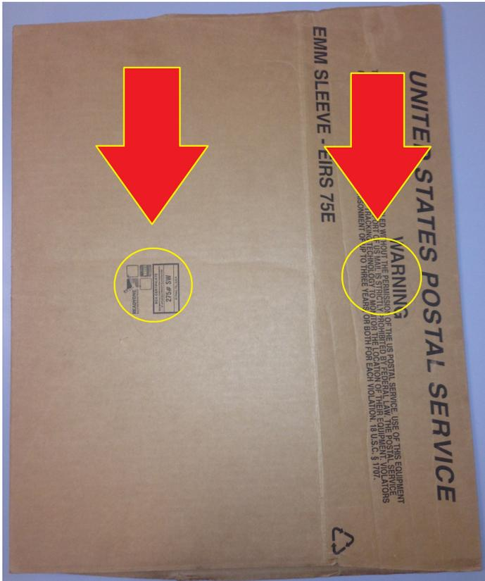
Fig. 15: Marks left by suction cups. Note: not to scale & the color yellow was used to show a clear distinction [13].
