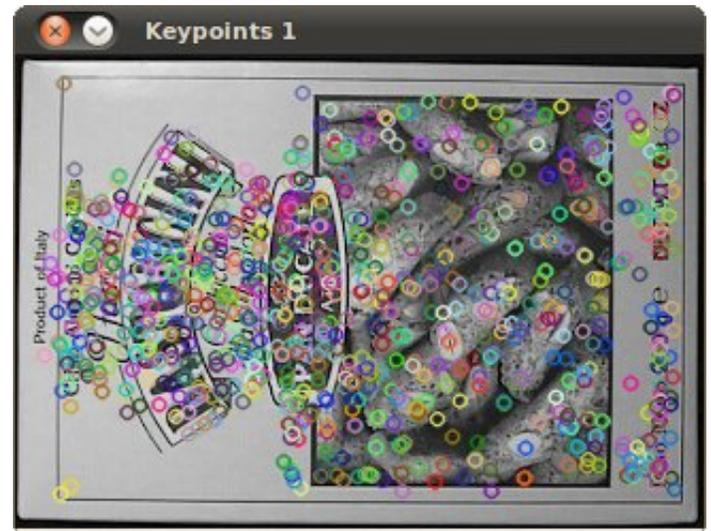
Fig. 14: Example of Features being defined by the "Surf" algorithm [12].
