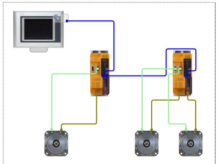
Fig. 25: Overview of Motion Control System [22].
