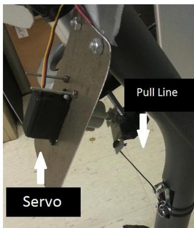
Figure B-7: The Servo and its connected line.
