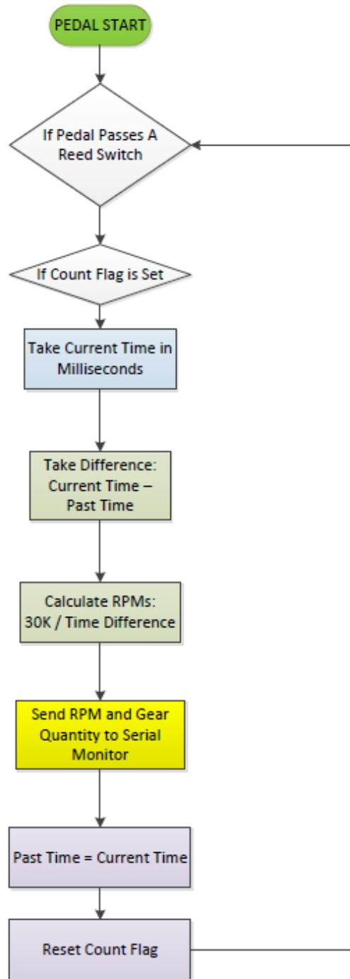
Figure B-10: Arduino Uno Flow of Operations.
