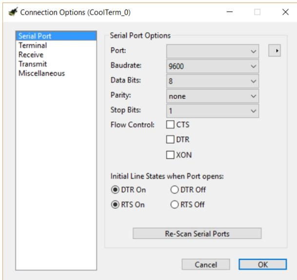
Figure A-3: Coolterm Options window [33].
