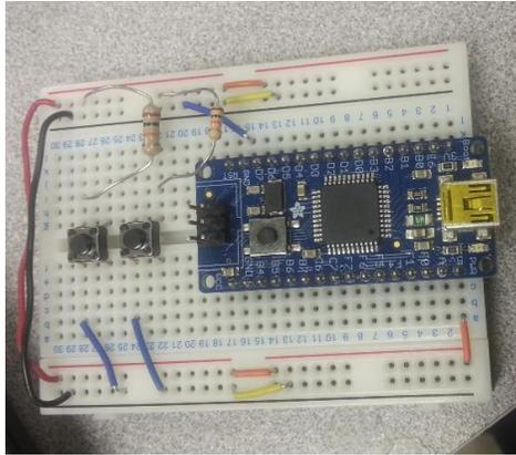
Figure B-9: A look at the Atmel ATmega32U4 Breakout Board.
