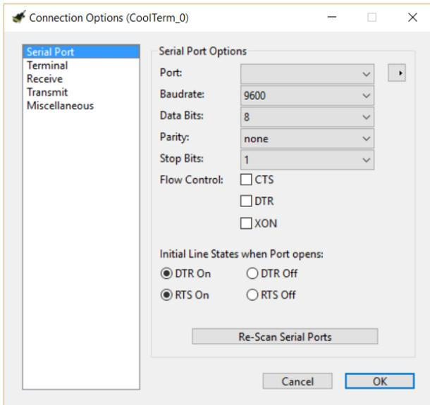
Figure A-3: Coolterm Options window [33].
