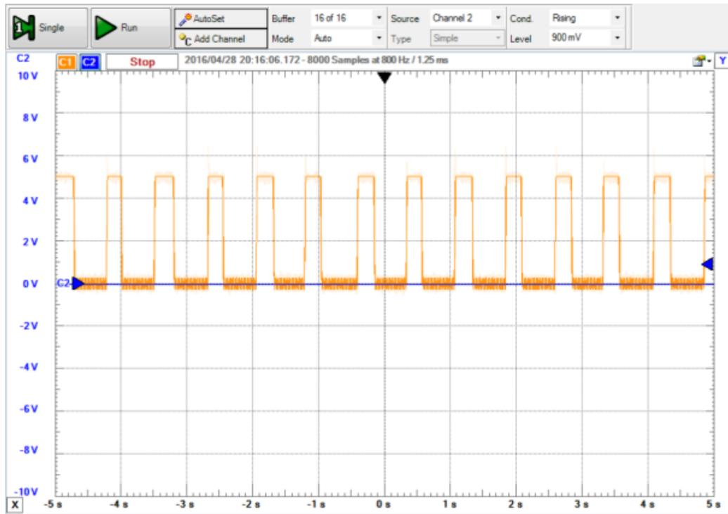
Figure B-2: The 40 BPM Waveform.
