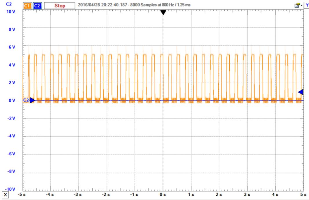
Figure B-5: The 100 BPM Waveform.
