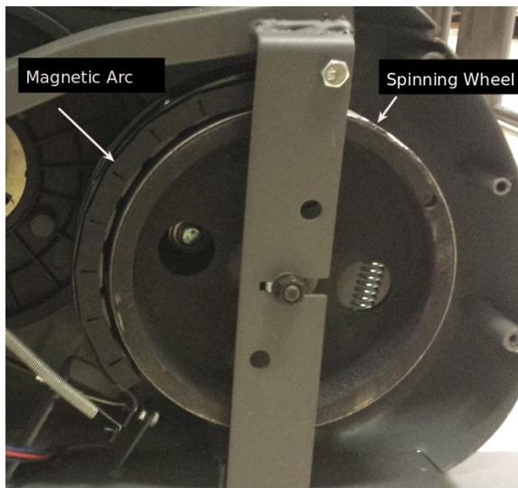
Figure D-3: Magnetic Arc and Spinning Metal wheel
