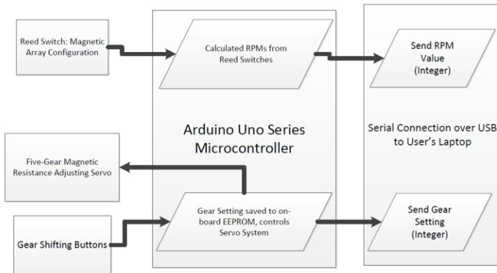
Figure B-1: The Block Level View
