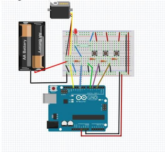
Figure B-8A: The Fritzing Diagram showing the Arduino Connections. Two of the buttons represent the Reed Switches, the third represents a reset state.
