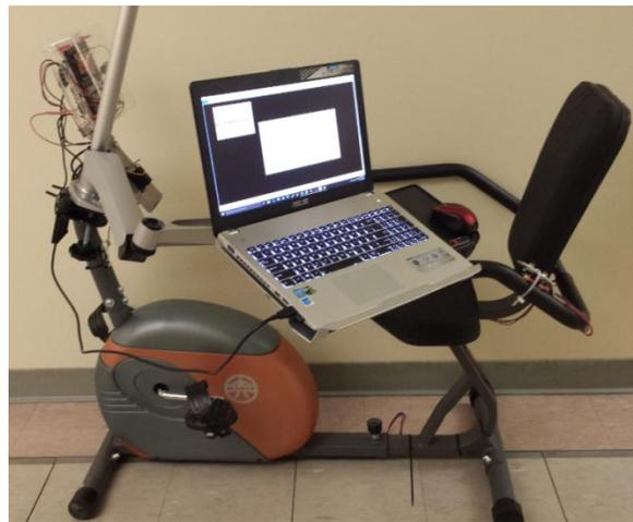
Figure D-2: Fully assembled Lapcycle with laptop stand and modified recumbent spin bike.
