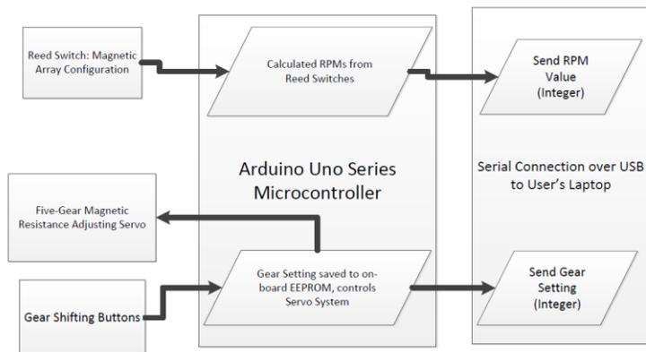
Figure B-1: The Block Level View
