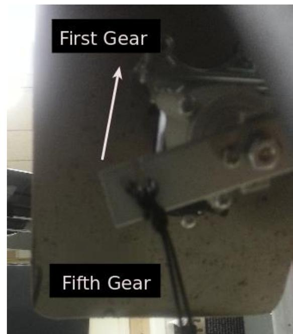
Figure D-4: Servo arm with corresponding gear positions
