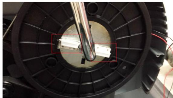
Figure B-6: The Finalized Reed Switch Array Configuration.
