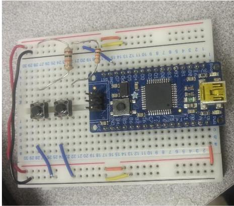
Figure B-9: A look at the Atmel ATmega32U4 Breakout Board.
