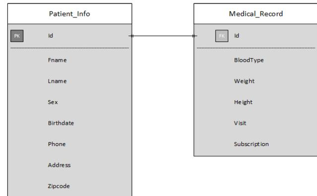
Fig 41 - Database Schema [77]
