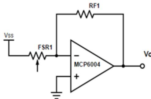
**Fig. 29 Inverting op-amp configuration. [63]** FSR1 is the force sensitive resistor and RF1 is the reference resistor.
