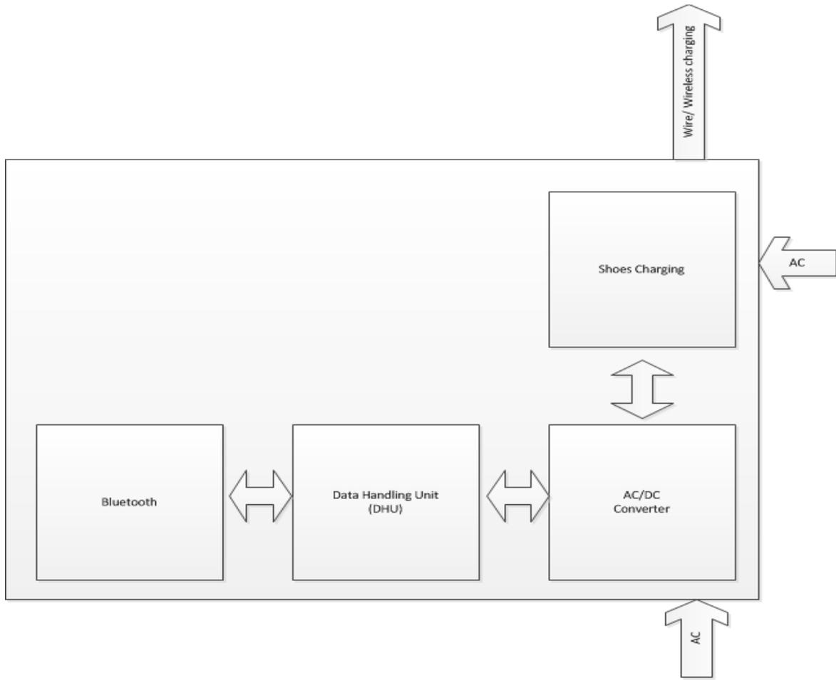
**Fig. 7 Docking Station Diagram [32]**
