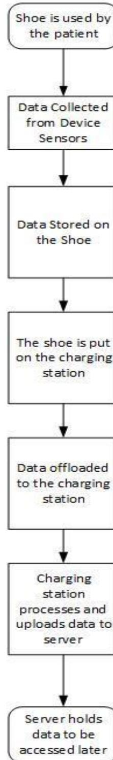
**Fig. 13 Top down level of Design [44]**
