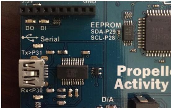
**Figure 17 : Serial Port on Propeller Board [50]**
