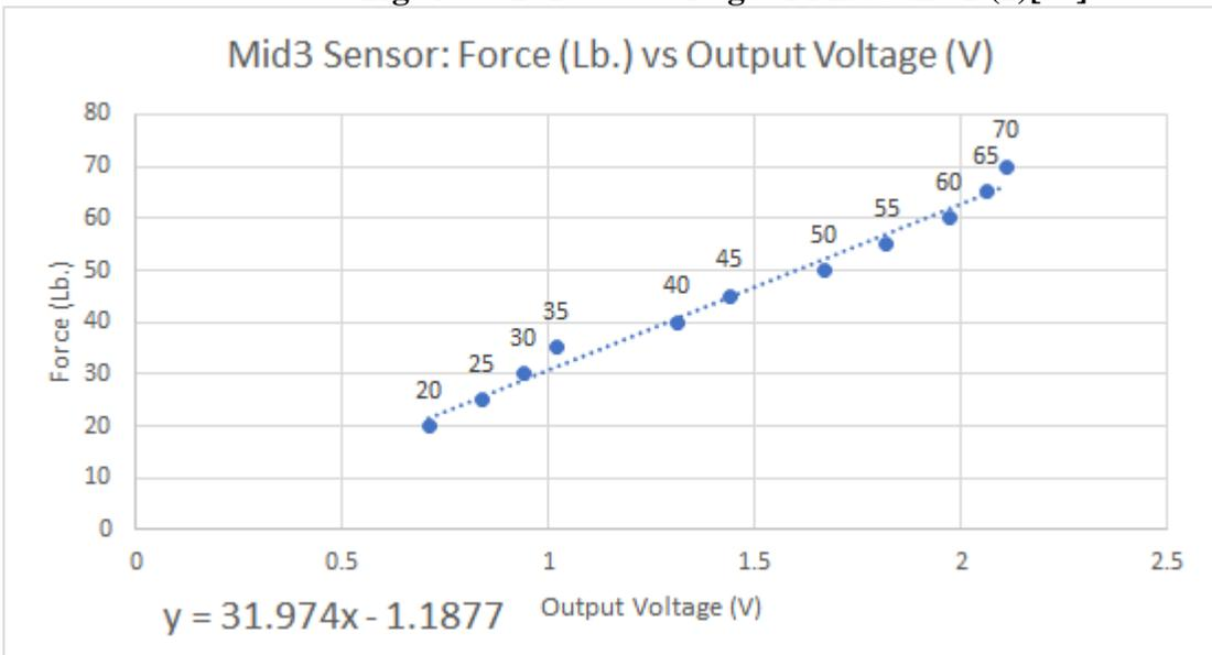
**Fig. 49c - Force vs Voltage of Mid Sensor (3) [86]**
