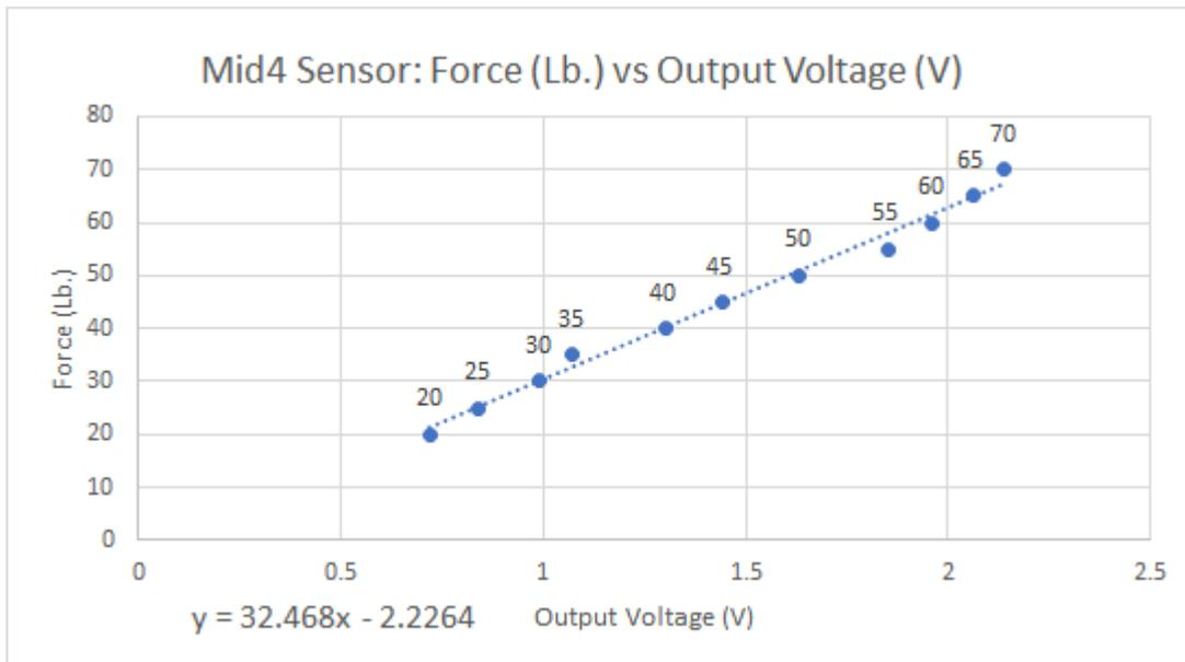
**Fig. 49d - Force vs Voltage of Mid Sensor (4) [86]**
