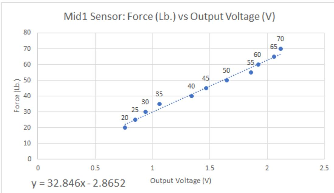
**Fig. 49a - Force vs Voltage of Mid Sensor (1) [86]**
