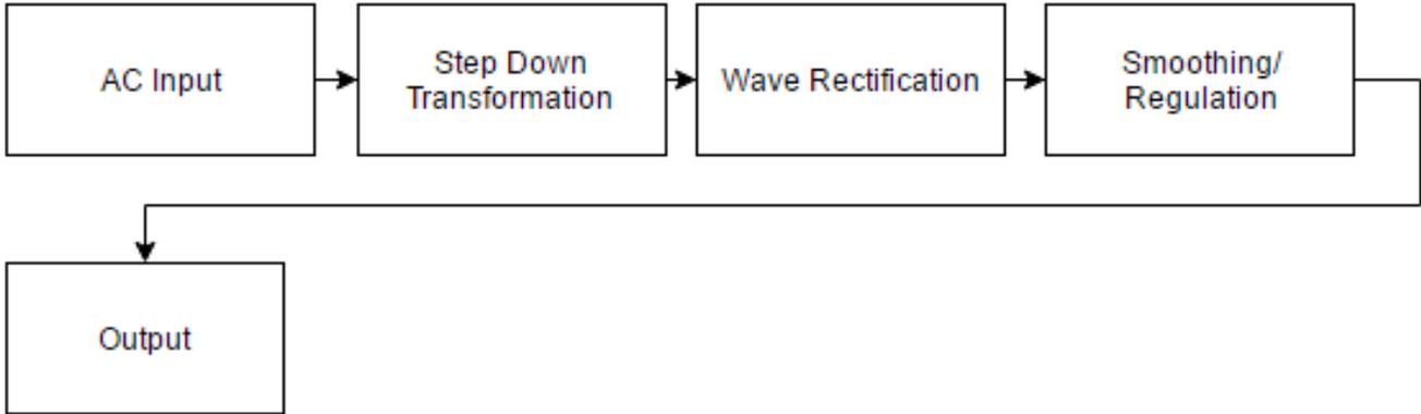
Figure 37 - Block level diagram for the AC/DC converter [70]
