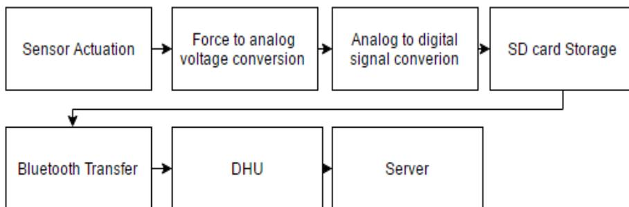
**Fig. 24 - Block diagram of hardware [58]**
