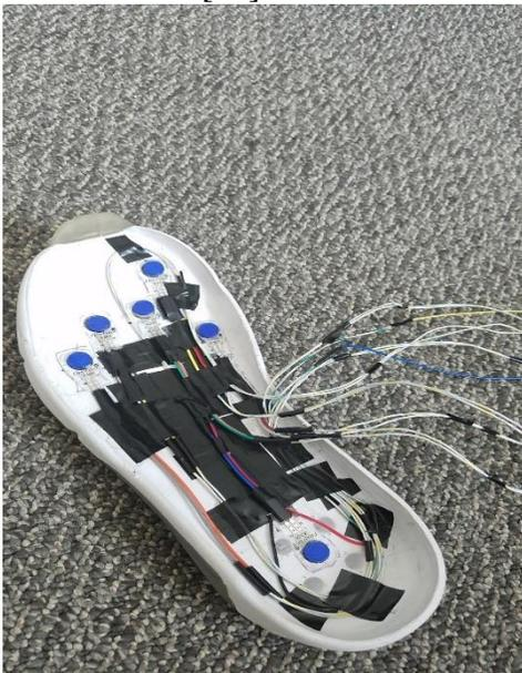
**Fig. 43 - Bottom Shoe Sensors Assembly-1 [80]**
