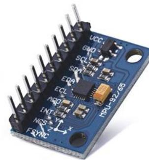
**Fig. 32 MPU-9250 gyroscope-acceleration-magnetometer combo.** [65]
