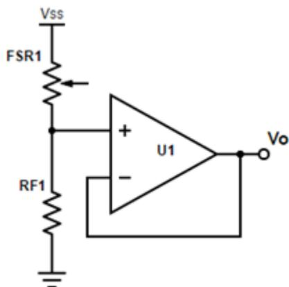
**Fig. 30 Voltage divider with unity buffer.** U1 is an MCP6004 op-amp.[64]
