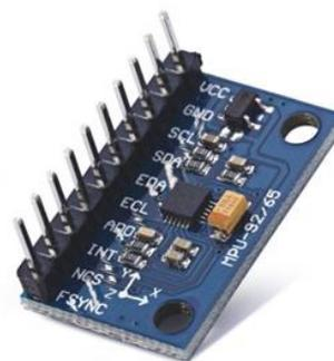
**Fig. 32 MPU-9250 gyroscope-acceleration-magnetometer combo.** [65]
