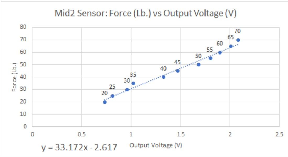
**Fig. 49b - Force vs Voltage of Mid Sensor (2)[86]**
