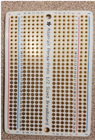
**Figure 46 - Protoboard by Ardafruit [83]**
