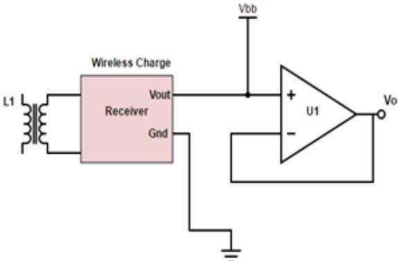
Figure 35 - Wireless charging circuit [68]
