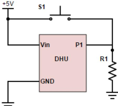
Figure 36 - DHU power circuit [69]
