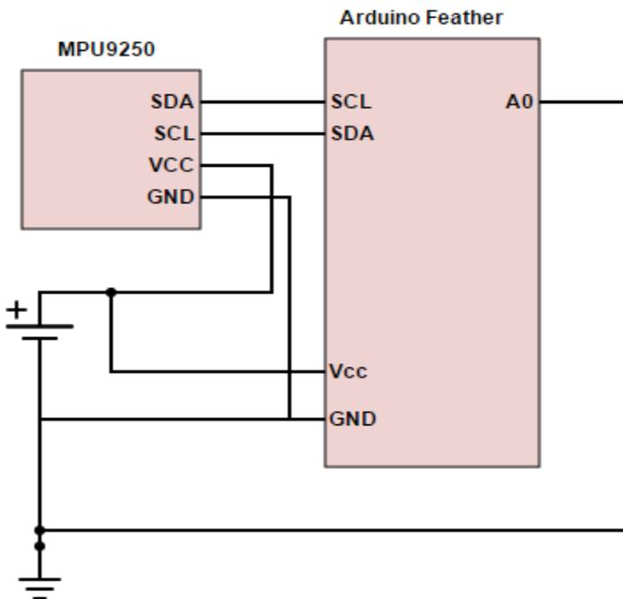
**Figure 33 - MPU - Feather Pins Connection [66]**
