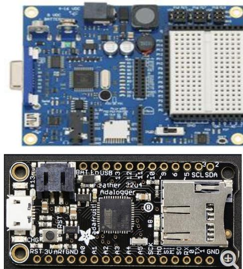
**Figure 15 - Propeller and Feather 32u MCU [47]**
