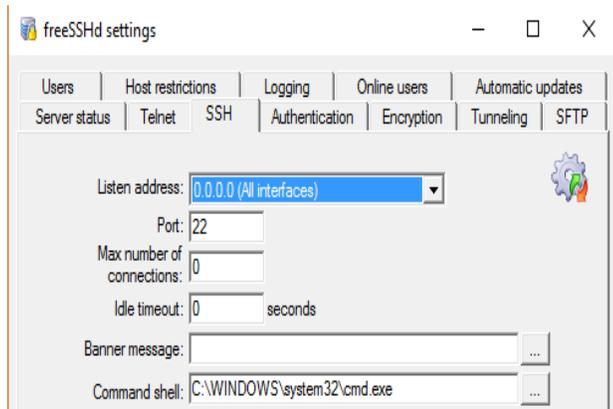
Figure 39-Configuration of SSH Server-1[75]
