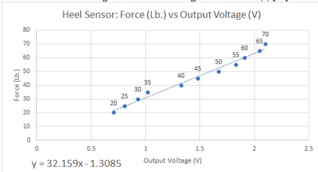
**Fig. 50 - Force vs Voltage of Heel Sensor [87]**
