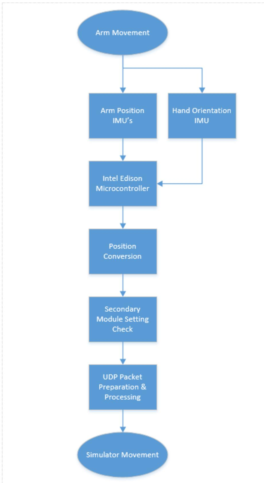
Fig. 9. Software block diagram for Precision Controller.
