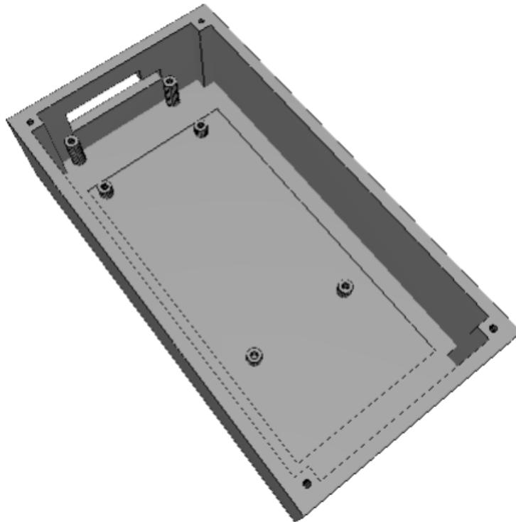
Fig. 13. Base design for the Precision Controller enclosure.
