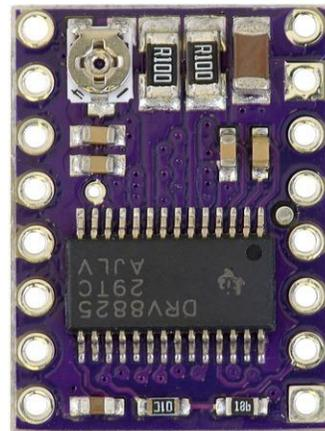
Figure 7- The Pololu DRV8825 stepper motor driver – image provided by Pololu Corporation
