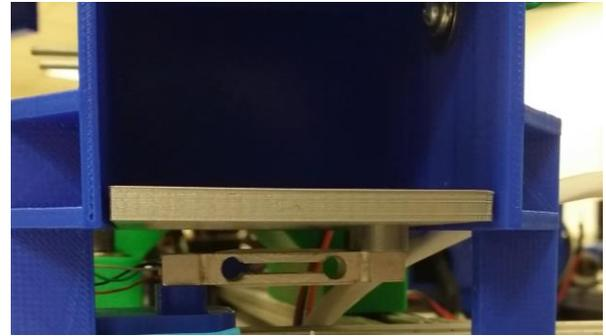
Figure 10 - The load cell mounted under the QTI chute and weigh plate
