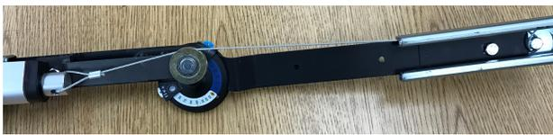
Figure 4: Pulley system on mounting bracket
