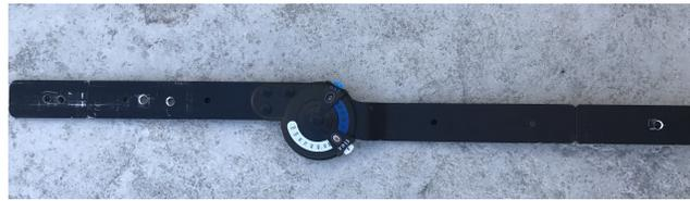
Figure 20: Brace with attachment holes drilled and threaded
