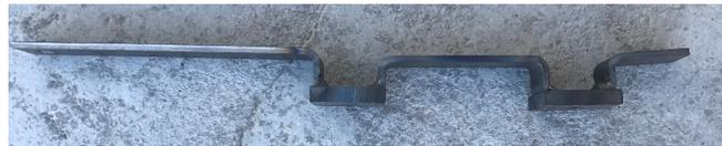
Figure 21: Machined steel mounting bracket for pulley system. The mounting bracket design was developed with the requirement of supporting 35 pounds of weight.
