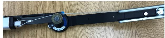
Figure 8: Pulley system on mounting bracket
