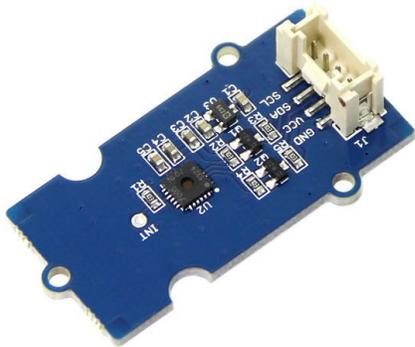
Figure 11: Temperature and Humidity Sensor [11]
