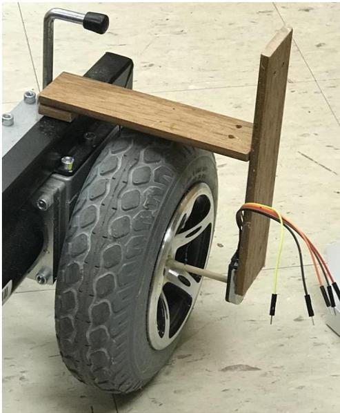
Figure 8. Mounting encoder onto wheelchair
