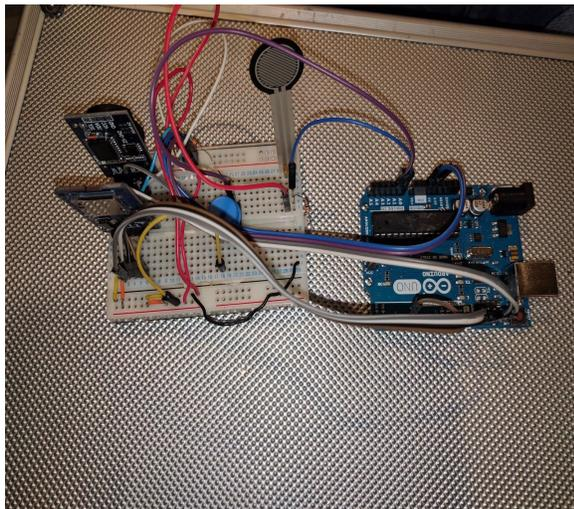
Figure 9 - Prototype Layout on Breadboard [22]
