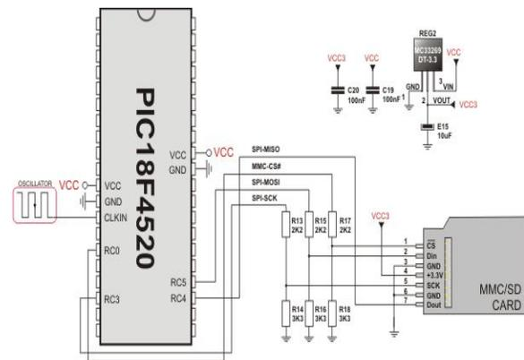
Figure 6: PIC Schematic with a MMC/SD Card [8]
