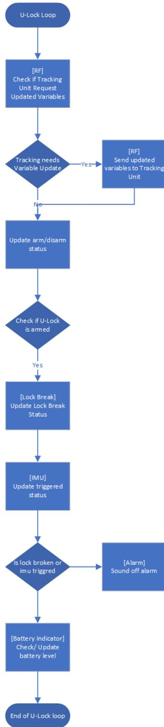
Fig. 12. Software flowchart of U-Lock component of combATS
