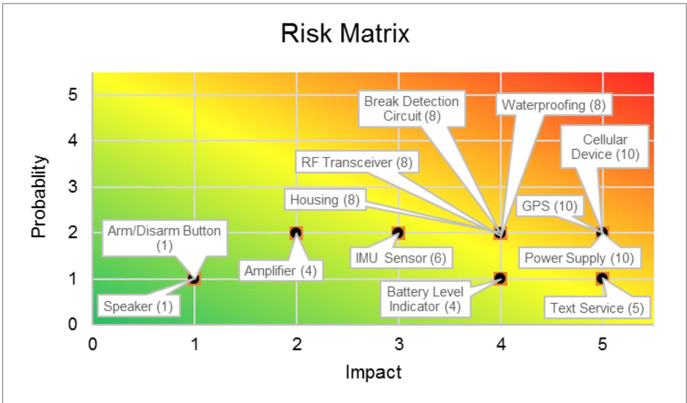
Fig. 7. Risk Matrix showing the Impact of component failure vs. the Probability of occurrence on a scale of 1 (low) to 5 (high). [11]
