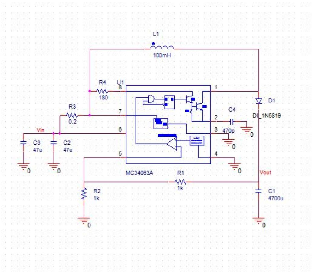
Fig. 11. Power Supply Schematic [15]
