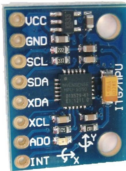
Fig. 3. InventSense MPU-6050 [9]
