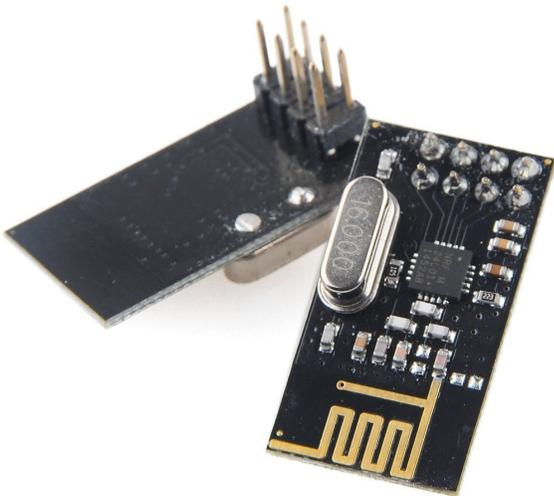
Fig. 5. A 2.4 GHz RF Transceiver [10]
