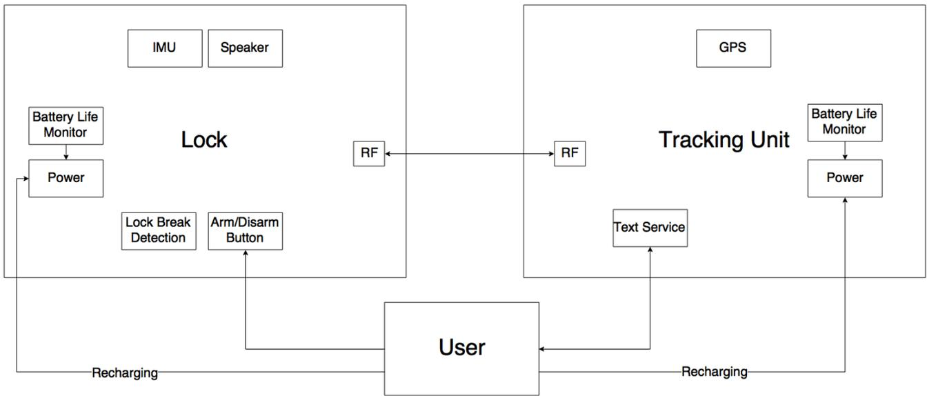
Fig. 10. Block Diagram of combATS
