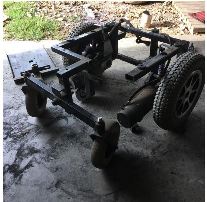
Fig. 10: Second Semester Chassis with Motors and Encoders
