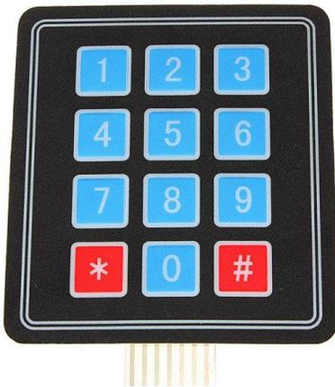
Figure 4: Membrane Keypad
