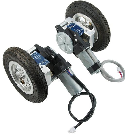
Fig. 18: DC motors by Parallax
